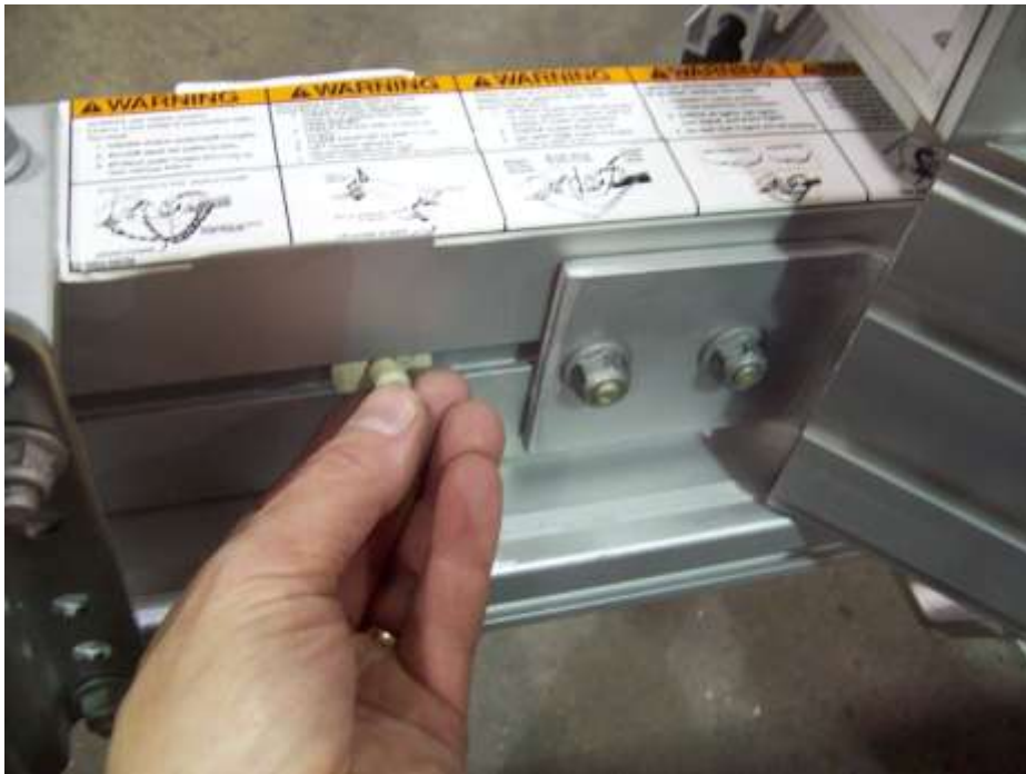
Insert one repair T-bolt on each side of the front tongue section. Repeat this process for the rear tongue section. These will be used to mount the side arm.
