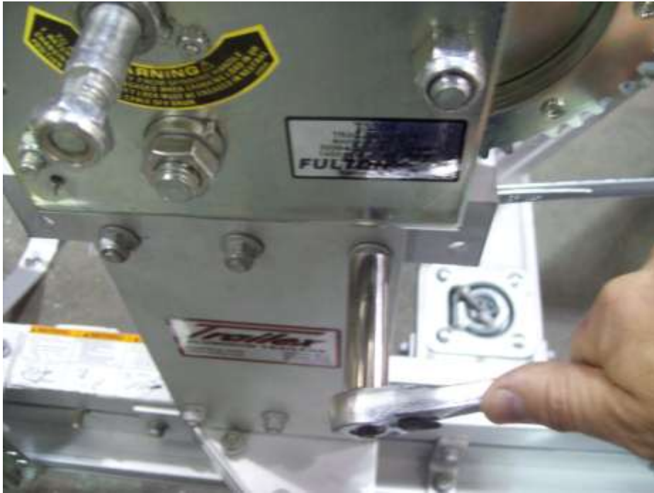
Tighten nuts on both of the side plates.
