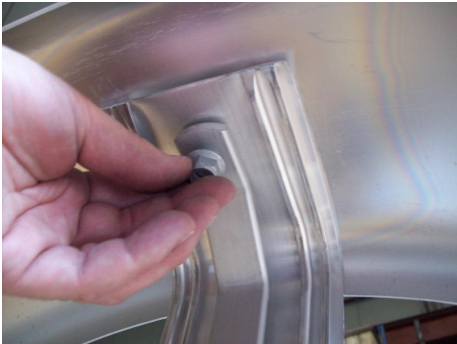
Install nut on the underside of fender.
