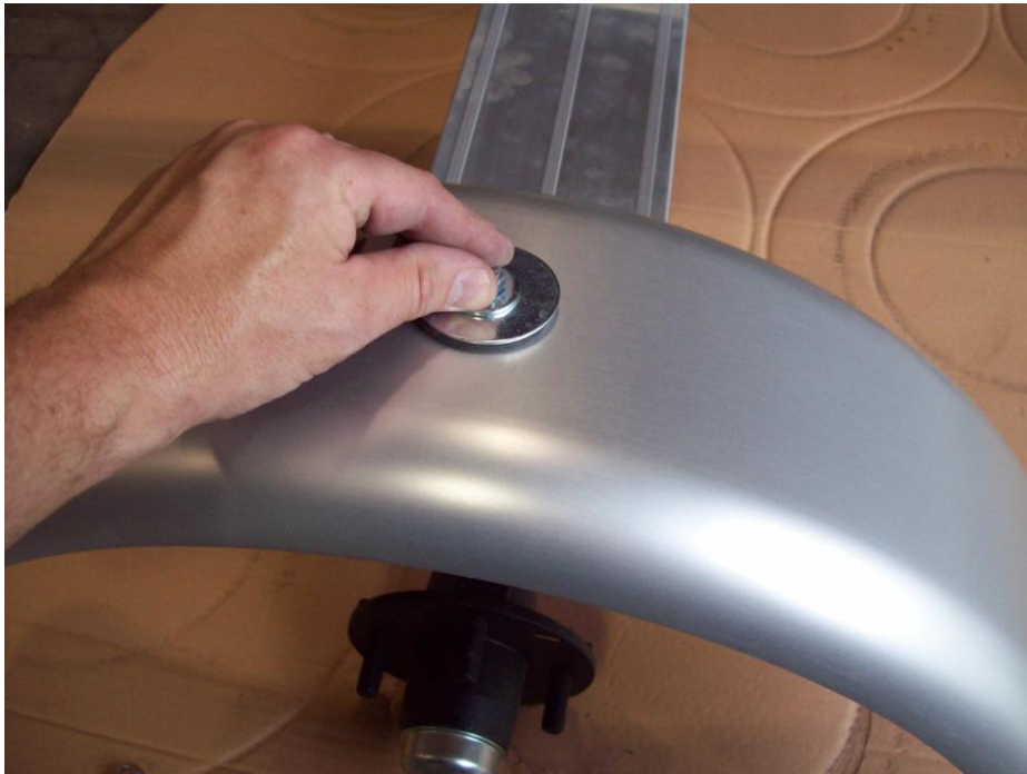
Insert bolt through washer, fender and brackets.
