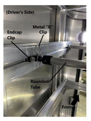
Replace the metal "R" clip, securing the rounded tube to the endcap clip.
