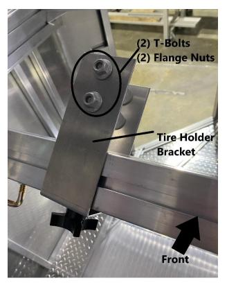
Loosely install (2) T-bolts and (2) flange nuts to the tire holder bracket as shown. At this point (4) T-bolt heads should be facing the inside the tire holder bracket.
