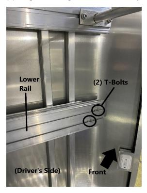
Locate (2) T-bolts from the hardware bag (Part "K"). Install (2) T-bolts into the grooves of the lower rail on the driver's side as shown.
