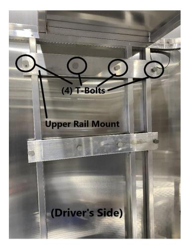
Repeat this process to loosely install (4) T-bolts and (4) flange nuts to the upper rail mount.
