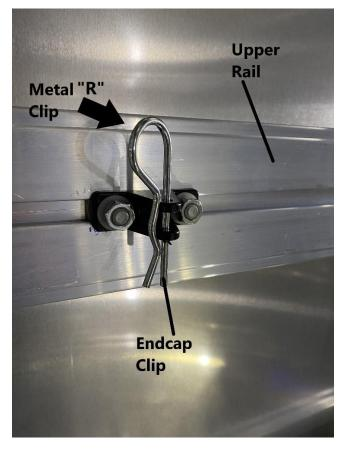
Remove the metal "R" clips from both endcap clips.
