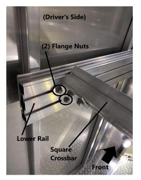
Loosely install (2) flange nuts onto the (2) T-Bolts.
