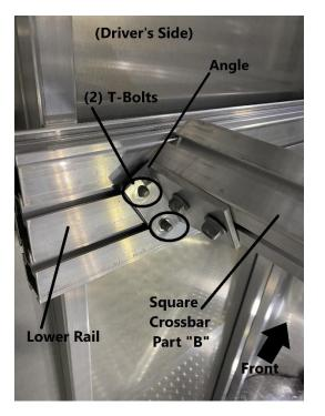
Two people will be necessary to install the square crossbar assembly (Part "B"). The square crossbar assembly <u>must</u> be supported by a second person during this process. Carefully bring the square crossbar into the trailer. Install the angle on the square crossbar assembly to the (2) T-bolts installed on the lower rail. <u>Use caution during this step as to not damage the enclosed skin.</u>
