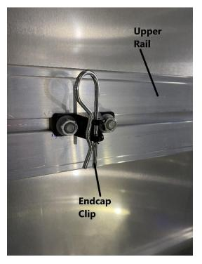
Locate the (2) endcap clips installed in the upper rails.
