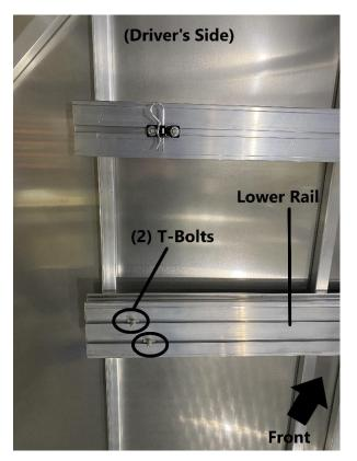
Install (2) T-Bolts into the grooves of the lower rail on the driver's side.
