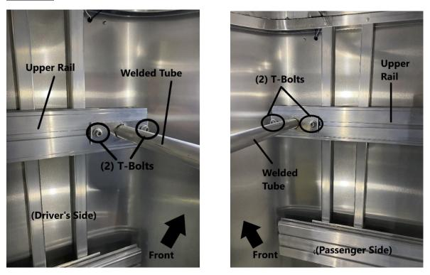
Rotate the welded tube sideways and install the remaining T-bolt into the grooves of the upper rails as shown. <u>Great care should be taken as to not damage the enclosed skin when installing the welded tube.</u>
