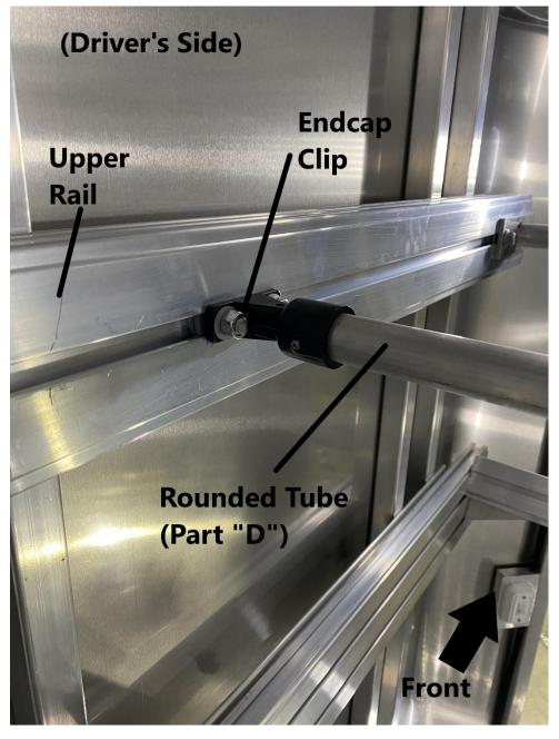
Two people will be necessary to install the rounded tube. Carefully bring the rounded tube into the trailer. Place the end of the rounded tube into the endcap clip. Line-up the hole of the round tube with the (2) holes of the endcap clip.
