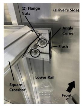
Slide the square crossbar assembly so that the end of the lower rail is flush with the leading corner of the angle installed on the square crossbar assembly. Tighten the (2) flange nuts using a 9/16" wrench. Repeat this process for the passenger side.
