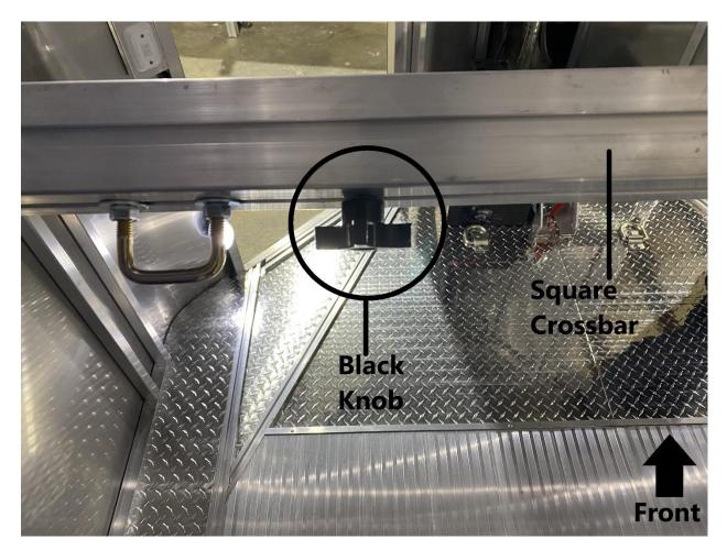
Locate the black knob installed on the square crossbar. Twist the black knob counterclockwise to remove it. This will leave a T-bolt installed.
