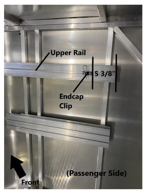
Repeat this process to install the remaining endcap clip to the passenger side upper rail.
