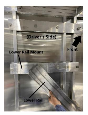
Starting with the second T-Bolt installed on the lower rail mount, slide the T-bolt head into the groove of the lower rail. <u>Take care not to damage the enclosed skin during installation of the rails.</u>
