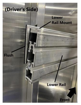
Confirm that the left side of the lower rail is flush with the left side of the lower rail mount. At this point the flange nuts can be tightened. Tighten the flange nuts using a 9/16" wrench. Take care not to damage the enclosed skin while tightening the flange nuts.
