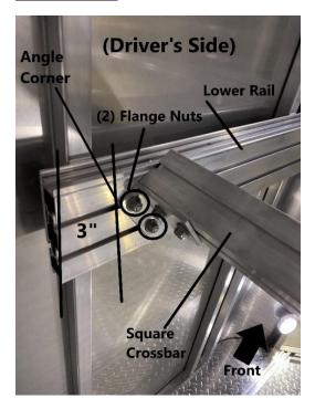
Measure 3" from the end of the lower rail to the leading corner of the angle installed on the square crossbar assembly. Tighten the (2) flange nuts using a 9/16" wrench. <u>Note that the 3"</u> <u>measurement is what we consider a reasonable starting point. This can be changed later if needed.</u>
