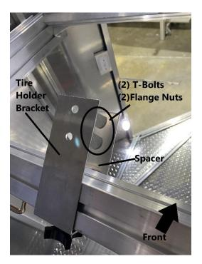
Loosely install (2) T-bolts and (2) flange nuts to the tire holder bracket as shown. At this point (2) T-bolt heads should be facing the inside the tire holder bracket.
