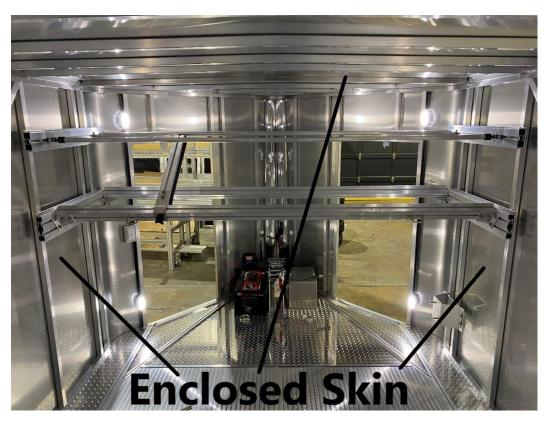
Before installing the tire rack, note the enclosed skin in the above picture. Great care should be used when installing the tire rack as to not damage the enclosed skin. The enclosed trailer should also be empty before installing the tire rack.
