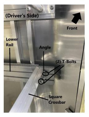
Two people will be necessary to install the square crossbar assembly (Part "C"). The square crossbar assembly <u>must</u> be supported by a second person during this process. Carefully bring the square crossbar into the trailer. Install the angle on the square crossbar assembly to the (2) T-bolts installed on the lower rail. <u>Use caution during this step as to not damage the enclosed skin.</u>
