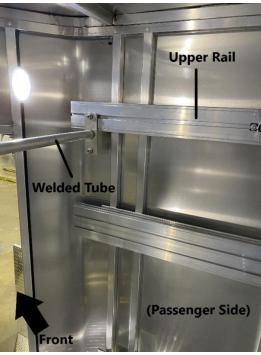
Two people will be necessary to install the welded tube. <u>*Carefully bring the welded tube into the trailer*</u>. Loosely install the welded tube into the grooves of the upper rails as shown.
