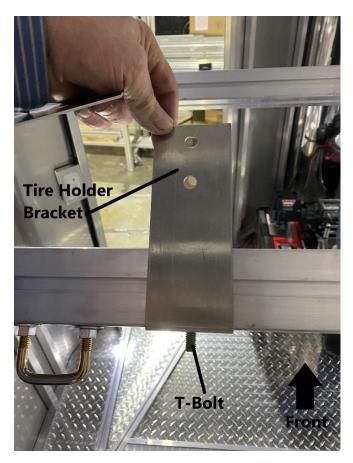
Install the tire holder bracket on to the T-bolt as shown.
