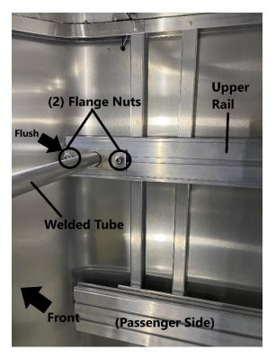
Confirm that the end of the welded tube is flush with the end of the upper rail. Tighten the (2) flange nuts using a 9/16" wrench. Repeat this process for the driver's side.
