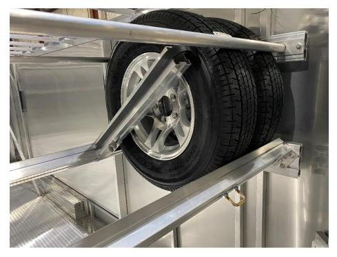
Place additional tires on the tire rack as shown. Move the adjustable tire holder next to the tires. Tighten the black knob on the adjustable tire holder to hold the tires in place. Straps are also recommended to secure the tires to the tire rack. Note that the crossbars may need adjusted if the tires don't fit or can fall through the crossbars. Do not load the trailer until all tires are secure and not moving.
