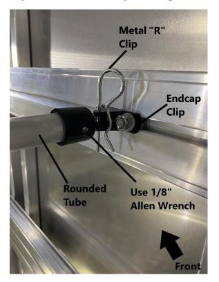
Repeat this process for the passenger side. Note that the holes may not line-up on the passenger side. If needed, use a 1/8" Allen wrench to adjust the endcap so that the holes line-up.
