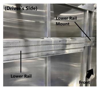
Continue sliding the lower rail towards the rear of the trailer. Install the first T-bolt into the groove of the lower rail.
