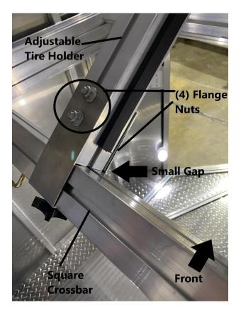
Leave a small gap between the square crossbar and the adjustable tire holder. Tighten the (4) flange nuts using a 9/16" wrench.
