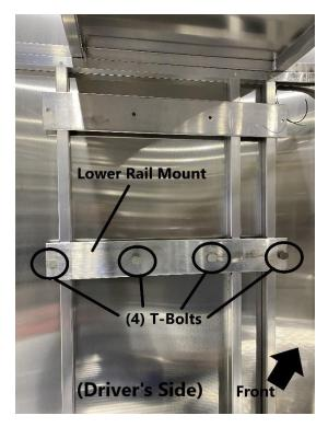
Loosely install (4) T-Bolts and (4) flange nuts to the lower rail mount as shown. The head of the T-bolt will be facing the inside of the trailer and the flange nut will be installed behind lower rail mount.
