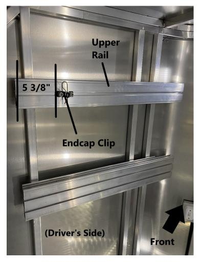
Install the endcap clip to the driver's side upper rail as shown. Measure 5 3/8" from the end of the upper rail to the left side of the endcap clip. Tighten the nuts installed on the endcap clip using a 9/16" wrench. <u>Note that the 5 3/8" measurement is what we consider a</u> <u>reasonable starting point. This can be changed later if needed.</u>
