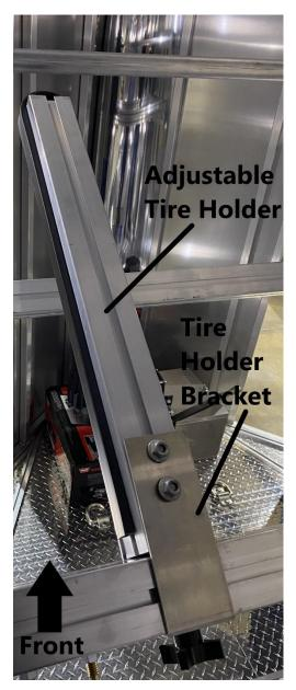
Install the adjustable tire holder to the tire holder bracket as shown. Slide the (4) T-bolts installed on the tire holder bracket into the grooves of the adjustable tire holder.
