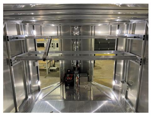
Completed tire rack. Confirm that all bolts/nuts are tightened before loading the tire rack.
