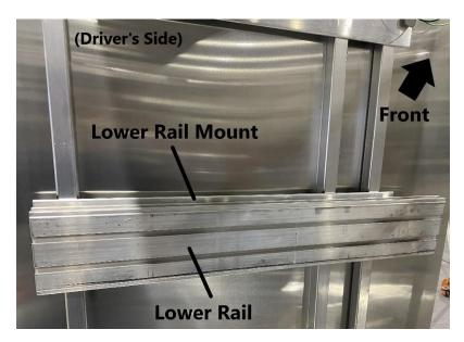
Slide the lower rail towards the front of the trailer, installing the remaining third and fourth T-bolts in to the groove of the lower rail. At this point all four T-bolts should be installed in the groove of the lower rail.
