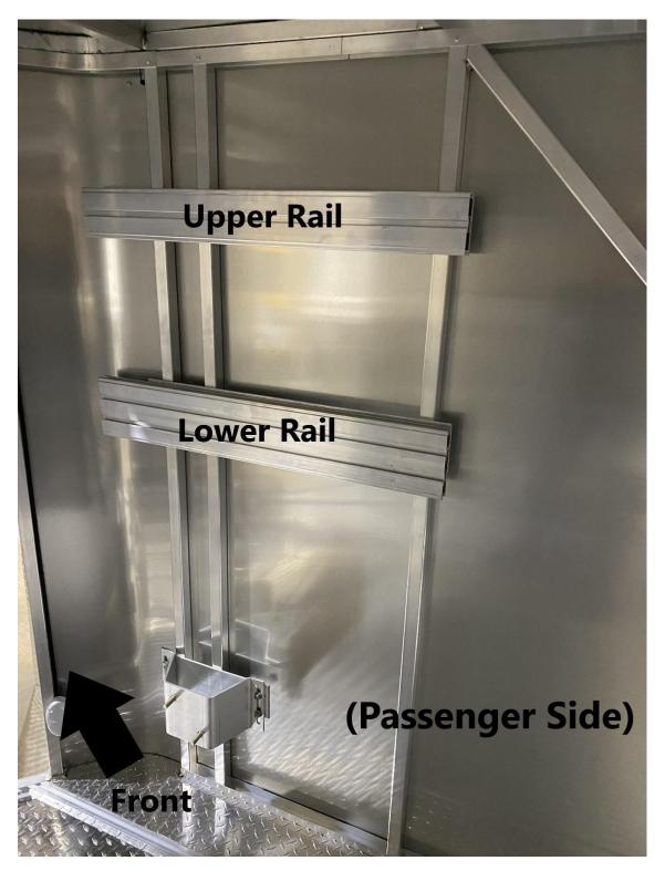
Move to the passenger side of the trailer. Repeat the earlier steps to install the remaining upper and lower rails to the mounts on the passenger side. At this point the passenger side of the trailer will look like this.
