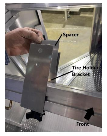
Place the spacer on the tire holder bracket as shown. Line-up the holes of the spacer with the holes on the tire holder bracket.
