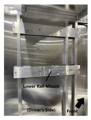
Move to the inside of the enclosed car trailer. Locate the lower rail mount on the driver's side of the trailer. This will be close to the front of the trailer.
