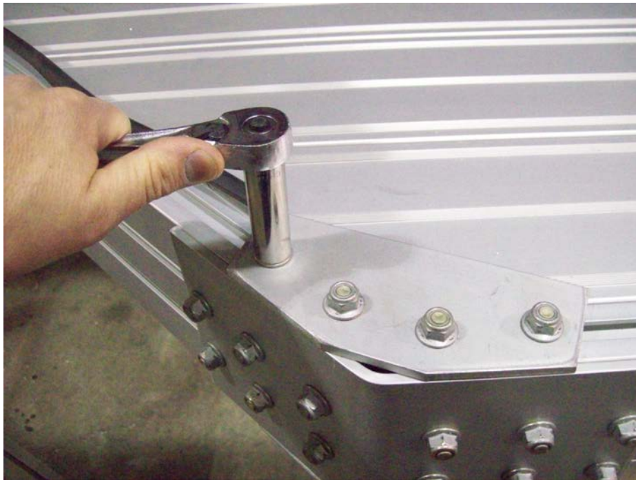
Remove the nuts on the top elbow plate.
