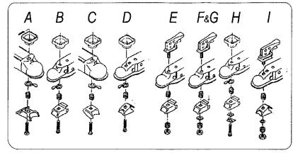
DANGER If housing is deformed, replace complete coupler.
