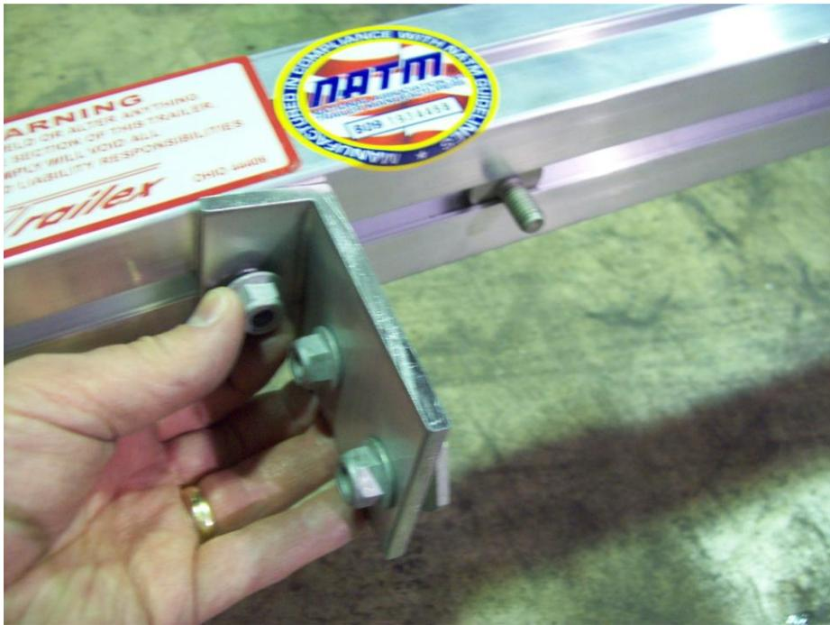
Install the angle bracket where the roller assembly was mounted.
