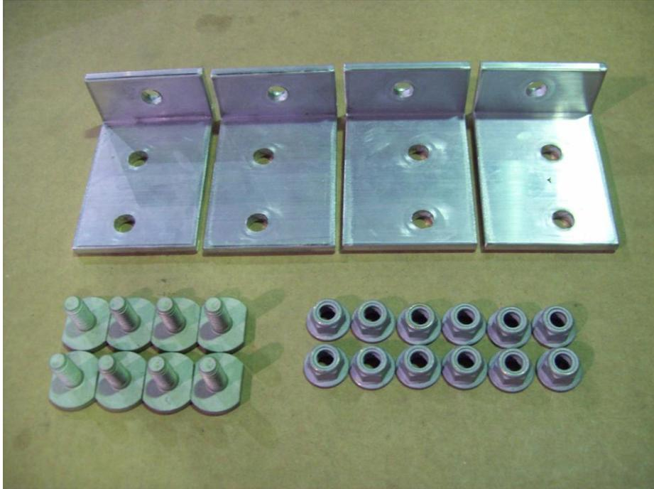
Locate 4 angle brackets, 8 T-bolts, and 12 nuts as shown.
