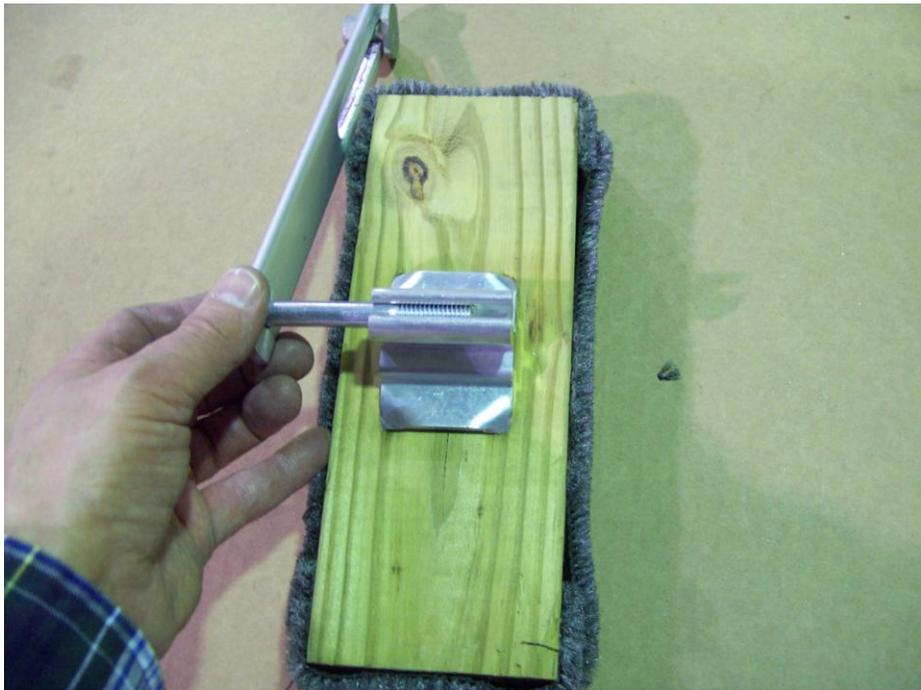
Insert bolt from the slotted bracket through the bunk pivot plate.
