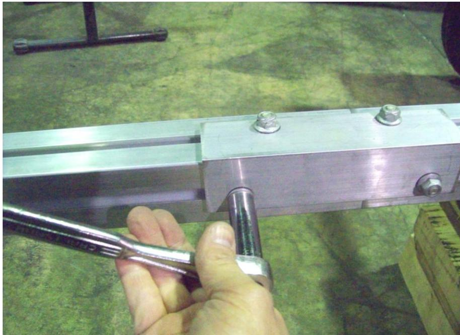
Start by loosening the nuts on the splice plate of the trailer.
