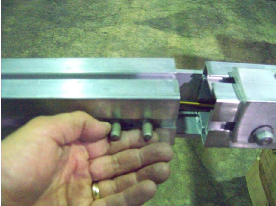
Slide two T-bolts in the front tongue sections on the left side. Then reinstall the splice plate and repeat for the other side.
