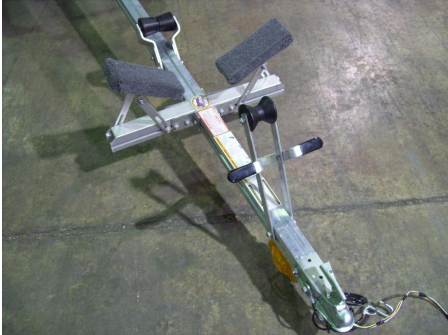
Final adjustment for the cradles will be made when boat is in position on the trailer.
