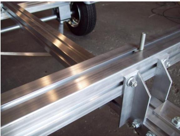
Slide the 1 1/8" T-bolt in the rear cradle holder to the center of the trailer.
