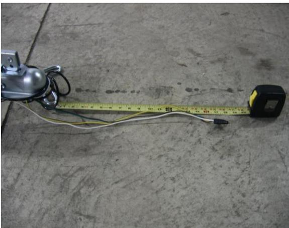
Pull the two wires at the back of the trailer through the tongue until there is approximately 18" protruding from the front.
