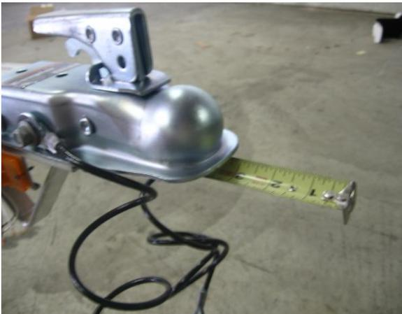
Extend a tape measure inside the tongue from the rear of the trailer until it protrudes at the front of the trailer under the coupler.
