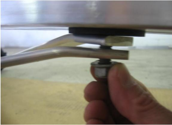
Install the forward ends of both tie rods to the 1 1/8" T-bolt.
