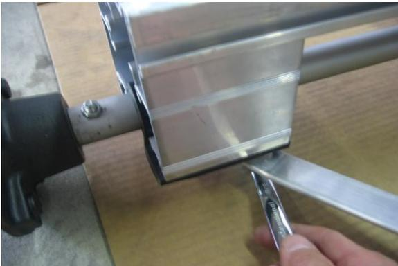
Important! Tighten nuts at both ends of the tie rods.
