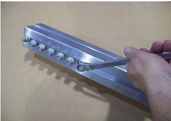
Remove the nuts from the two forward most T-bolts located on either side at the end of the rear tongue section.
