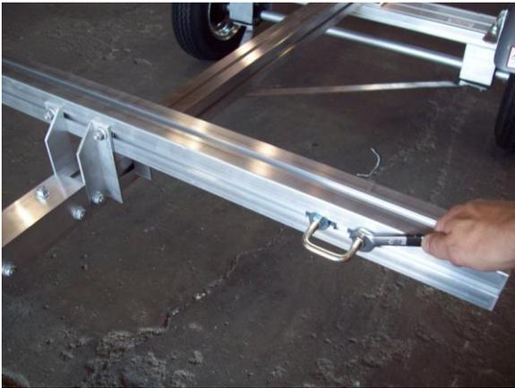
Tighten the nuts. Repeat by installing 2 clips in the rear slot of the rear cradle bracket.
