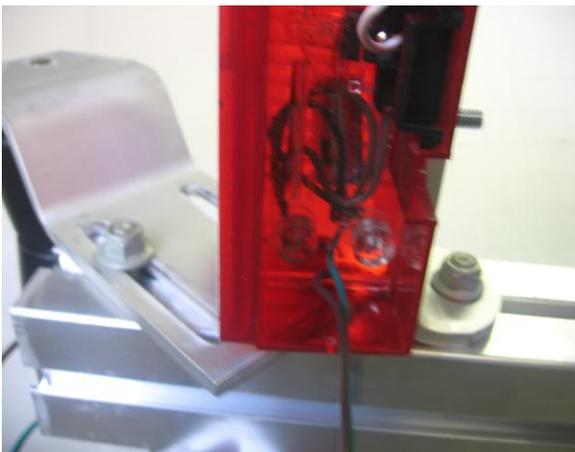
Re-install the bulb assembly into the light housing making sure to route the wires through the slot in the base of the bulb assembly. Repeat for the left side.
