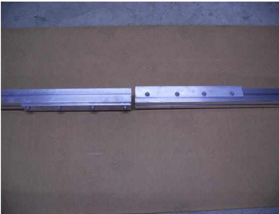
Unwrap the two tongue sections and lay them end to end with the splice plates adjacent to each other.
