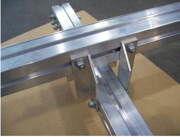
Install the rear cradle holder 8 1/2" from the end of the rear tongue section. Final location will be determined later when the tail lights and rear roll are installed.
