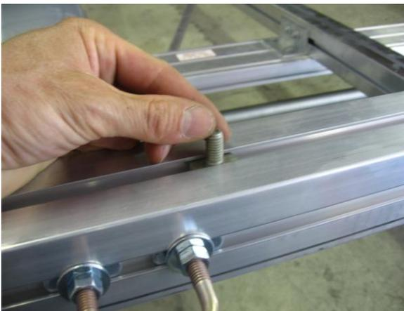
Slide the 3/4" T-bolts on either side of the 1 1/8" T-bolt.
