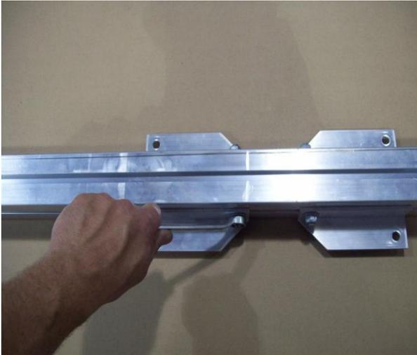
Loosen the four nuts securing the mounting angles to the front cradle holder and rotate them downward into position.
