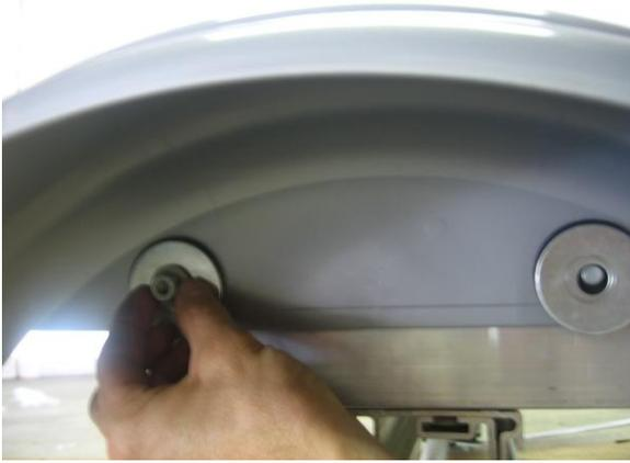
Install the remaining (2) rubber washers, (2) steel washers, and (2) lock nuts as shown. Repeat for the other fender.
