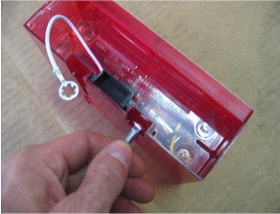
Slide the carriage bolts into the slots in the back of the tail lights.
