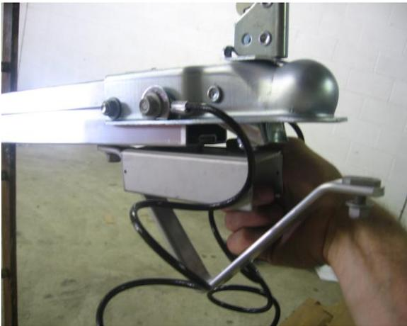
Slide the running light bracket into the bottom slot in the front tongue section.
