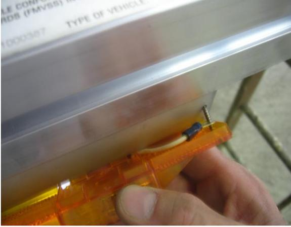
Install the running lights into the pre-drilled holes in the running light bracket using a Philips screwdriver. Be sure the screw is through the ring terminal on the back side of the lights. DO NOT OVER TIGHTEN.
