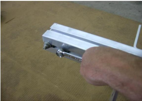
Remove the remaining two nuts and bolts from both sides of the rear tongue section.
