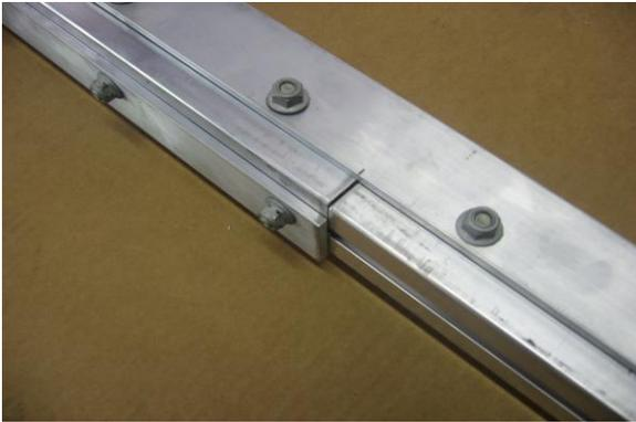
Slide the plate over the adjacent tongue section until the pencil mark at the center of the splice plate is aligned with the gap between the tongue sections.
