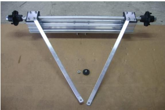
Rotate both tie rods forward.
