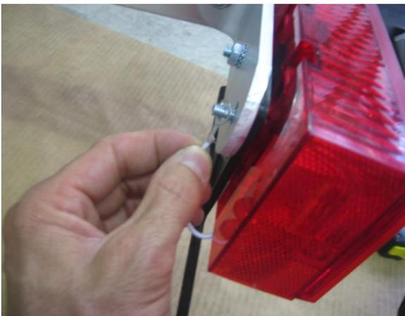
Install the white ground wire from the tail light onto the carriage bolt. Repeat this procedure to install the right tail light onto the right tail light bracket.
