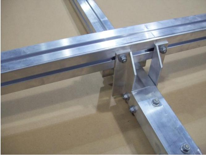
Attach the cradle bracket to the tongue section aligning the angles with the pencil marks on either side of the tongue section. Align the angles with the pencil marks on the cradle holder. The cradle holder bracket should rest against the tongue splice plate as shown.
