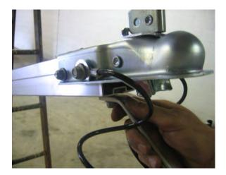
Slide the rear of the skid into the bottom slot in the front tongue section. Do not install the front of the skid yet.
