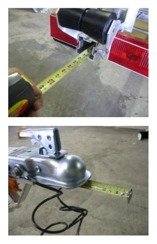
Extend a tape measure inside the tongue from the rear of the trailer until it protrudes at the front of the trailer under the coupler.
