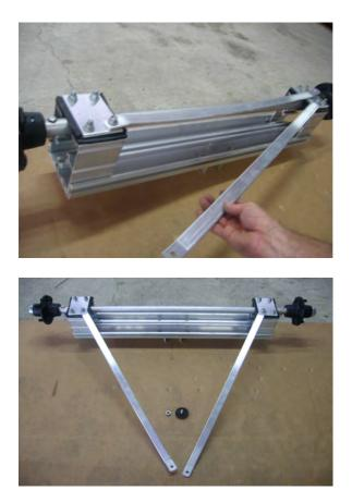
Rotate both tie rods forward.
