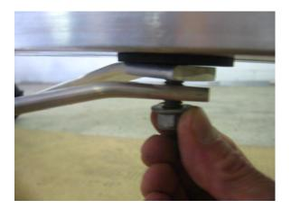
Install the forward ends of both tie rods to the 1 1/8" T-bolt. This will ensure that the axle assembly is perpendicular to the tongue.
