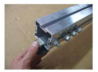
Locate the 1 1/8" T-bolt that was previously removed. Put it into the bottom slot at the back of the rear tongue section, slide it forward approximately 72" and leave it there.
