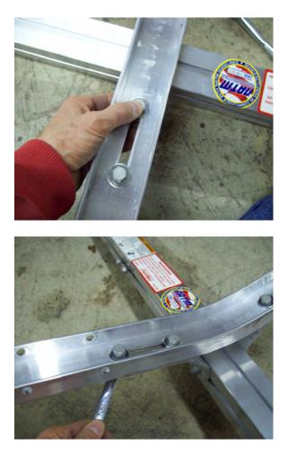
Slide the bolts out to the ends of the slots and tighten the nuts.
