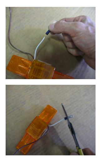
Install the ring terminals by crimping the terminal onto the bare wire.
