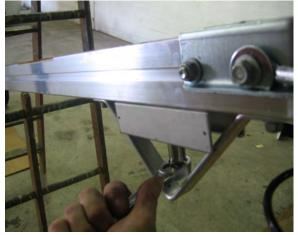
Tighten the nuts for the skid and running light bracket in the location shown.
