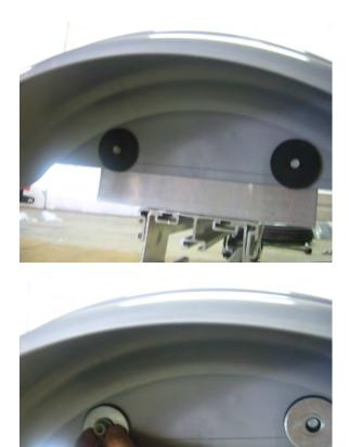
Install the remaining (2) rubber washers, (2) steel washers, and (2) lock nuts as shown. Repeat for the other fender.
