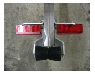
Loosen the tail light brackets, slide them to the rear as far as possible and tighten the nuts. (Roll may not always be used)
