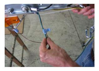
Measure 22" back from the front plug on the green/brown wire and pass the brown wire through the open slot in the second light blue connector at this location. The green wire will rest just outside the connector. Insert the brown wire from the running lights into the closed side of the connector and close the spade and cover as previously described. This will make the connection from the main harness to the running lights.
