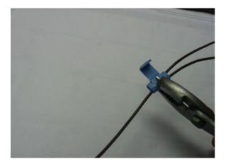
(Illustration) Use pliers to push the metal spade down until it is flush with the plastic. This is what makes the electrical connection between the two wires.
