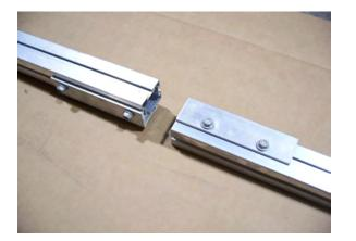
Lay the tongue sections end to end with the splice plates adjacent to each other. Loosen 4 nuts on each splice plate.
