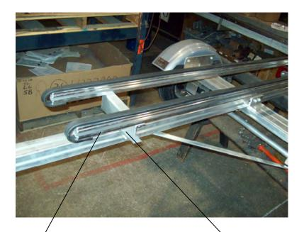
Front bracket. With "T" bolt in center of tongue take "C" channel bracket first then nut Tighten, then locate with drawing above.
