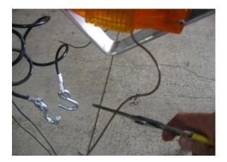
Cut 6" off of the brown wire on the left (driver's side) running light. Do not strip the wire.
