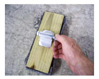
Remove the bolt from the pivot plate.
