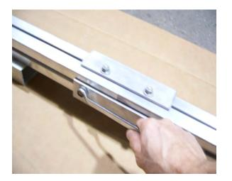
Tighten all 8 nuts making sure that the tongue sections are as tight as possible to one another. Set the tongue aside.
