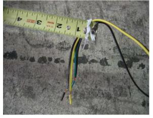
Attach both wires of the harness to the end of the tape measure using the ties provided with the harness.
