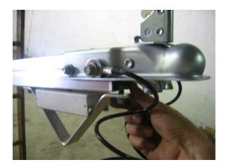
Slide the front of the skid into the bottom slot in the front tongue section.
