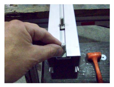
Slide 2 T-bolts on the underside of the front tongue section that has the serial number on it.
