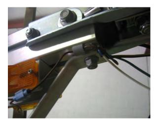
Install it as shown and run the brown wire from the running lights through it.
