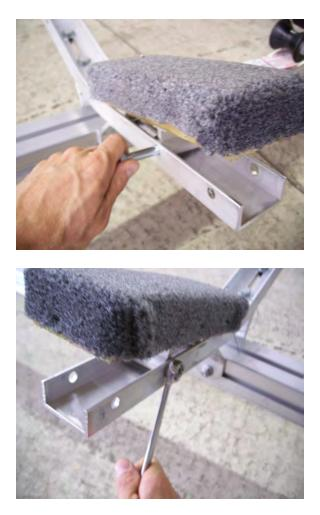
Install the padded cradle (inner position shown – this may vary depending on the width of the hull). Final angle will be determined when the trailer is fitted to the boat.
