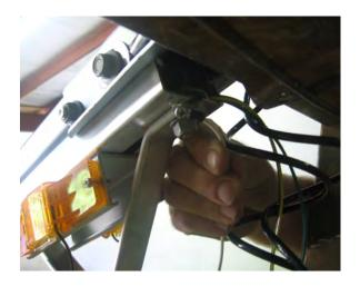
Install the ground wire into the pre-drilled hole located under the tongue just behind the <u>coupler</u>.
