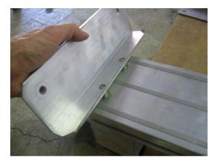
Install the fender brackets onto the bolts.
