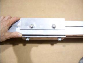
Slide each plate over the adjacent tongue section until the plates are centered over the gap between the tongue sections.
