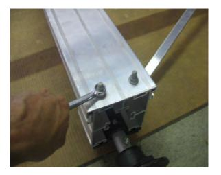
Remove the nuts from the top of the axle assembly.
