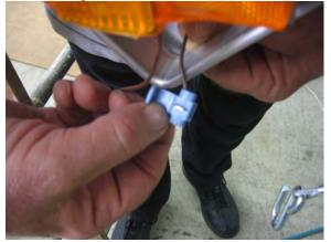
Insert the brown wire from the left (driver's side) running light into the hole in the connector closest to the hinge. This hole does not pass all the way through. The wire should go in about  $\frac{1}{2}$ ".
