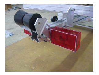
Repeat this procedure to install the right tail light onto the right tail light bracket. (Roll may not always be used)
