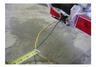
Retract the tape measure until it comes out of the back of the tongue with both wires attached.
