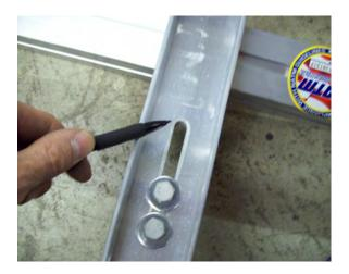
Make sure the slots in the cradle holder line up with the slots in the holder bracket.
