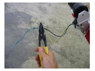
Cut the excess wire at the rear of the trailer leaving 12" exposed.
