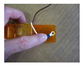
Align the ring terminals with the screw hole nearest the wire on the back of the running light. Make sure the wire is routed through the gap on the back of the light so it does not become pinched when the light is installed.
