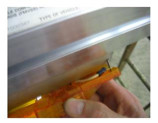
Install the running lights into the pre-drilled holes in the running light bracket using a Philips screwdriver. Be sure the screw is through the ring terminal on the back side of the lights. This will supply a ground to the lights. <u>DO NOT OVER TIGHTEN</u>.
