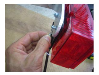
Install the white ground wire from the tail light onto the carriage bolt.
