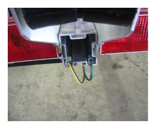
Install adhesive backed clamps in the locations shown and route the wires through them.
