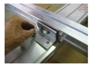
Loosely re-install the cross member attaching angle that was removed previously. Do not completely tighten the nuts yet.
