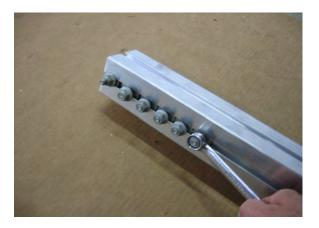
Remove the nuts from the two forward most T-bolts located on either side at the end of the rear tongue section. Slide them forward to the pencil marks approximately 42".
