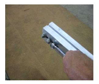
Remove the nuts from the forward most T-bolts located at the end of the rear tongue section.
