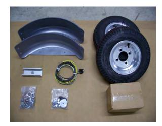
Fenders, tires, light kit, wiring harness, running light bracket, fasteners.
