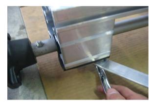
Important! Tighten the nuts at <u>both</u> ends of the tie rods.
