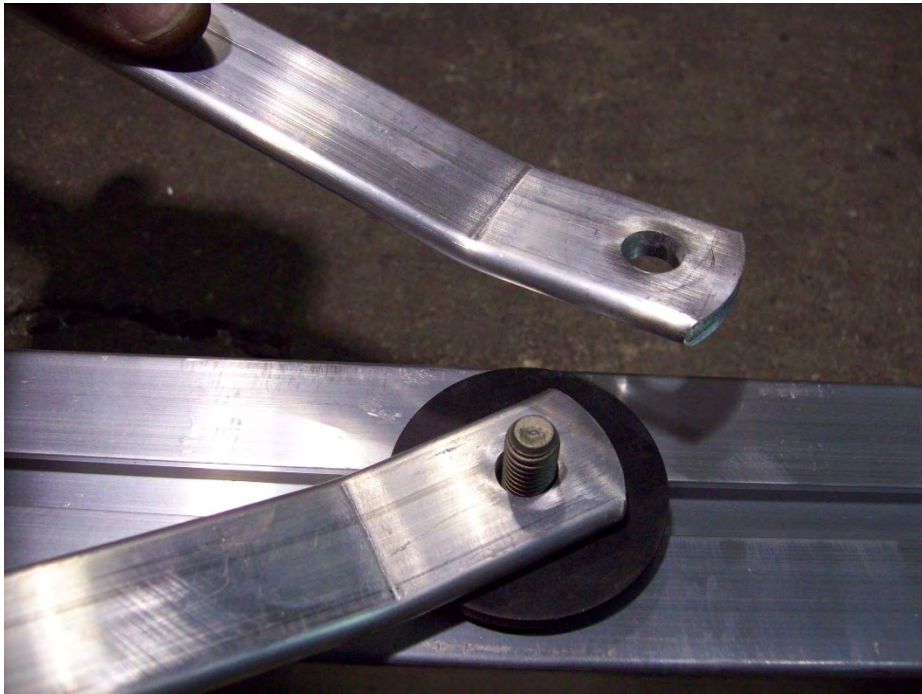
Shown upside down Lift both tie rod ends off the T-bolt.
