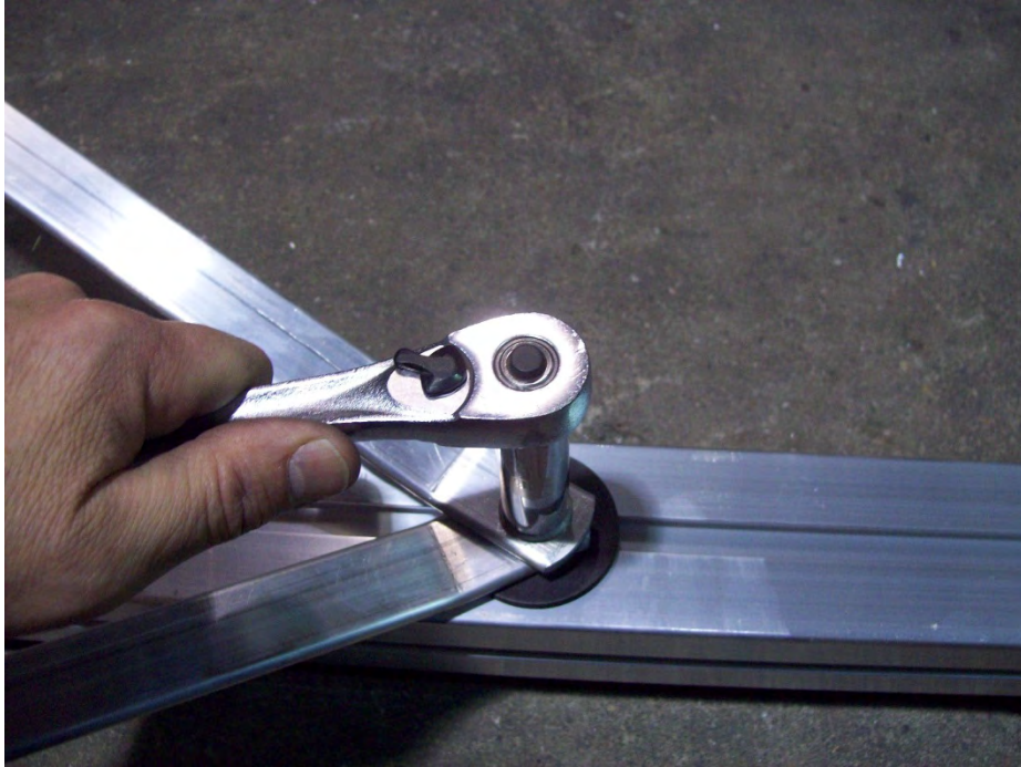
Shown upside down Remove the nut from the tie rod ends.
