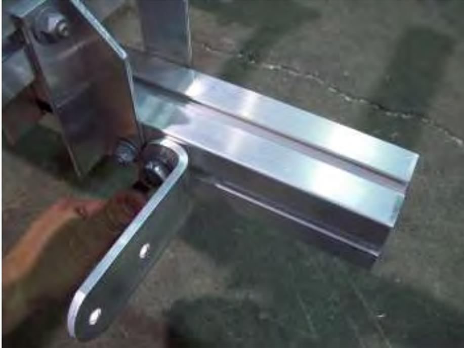
Install nuts and tighten.
