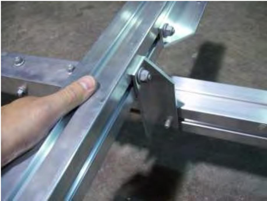
Install angle brackets over T-bolts as shown.
