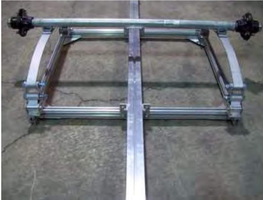
Locate the axle and install it on the springs as shown. Make sure the locating studs on the springs are in the holes on the axle's spring seat. Face the axle's serial plate toward the rear of the trailer to protect it from debris.
