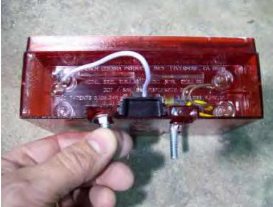
The light with the yellow wires is for the left (drive's side) of the trailer. Slide the carriage bolts into the slots in the back of the tail lights.
