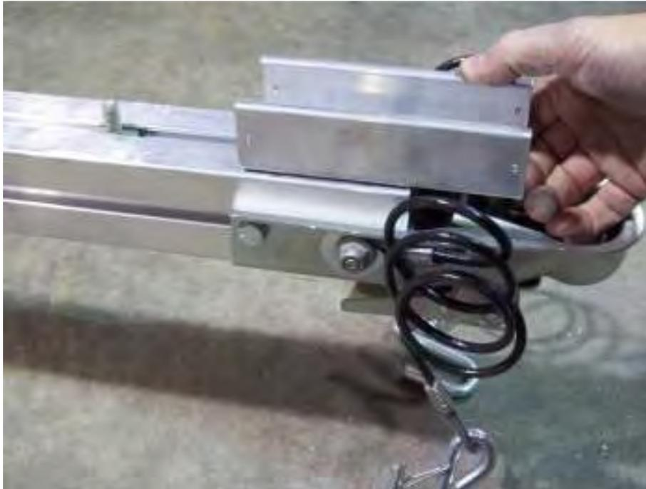
Slide the running light bracket into the slot in the front tongue section.
