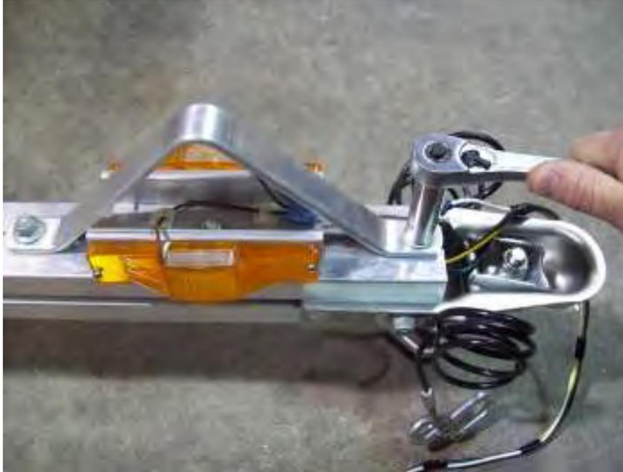
Re-install nut and tighten in position.
