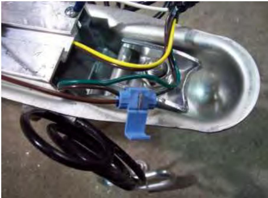
Pass the brown wire through the open slot in the second blue connector at this location. The green wire will rest just outside the connector. Insert the brown wire from the running lights into the closed side of the connector and push the spade down and close cover as previously described. This will make the connection from the main harness to both running light.
