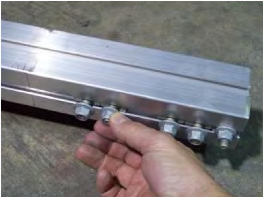
Slide the next two forward facing T-bolt on either side of the rear tongue section to the pencil marks.
