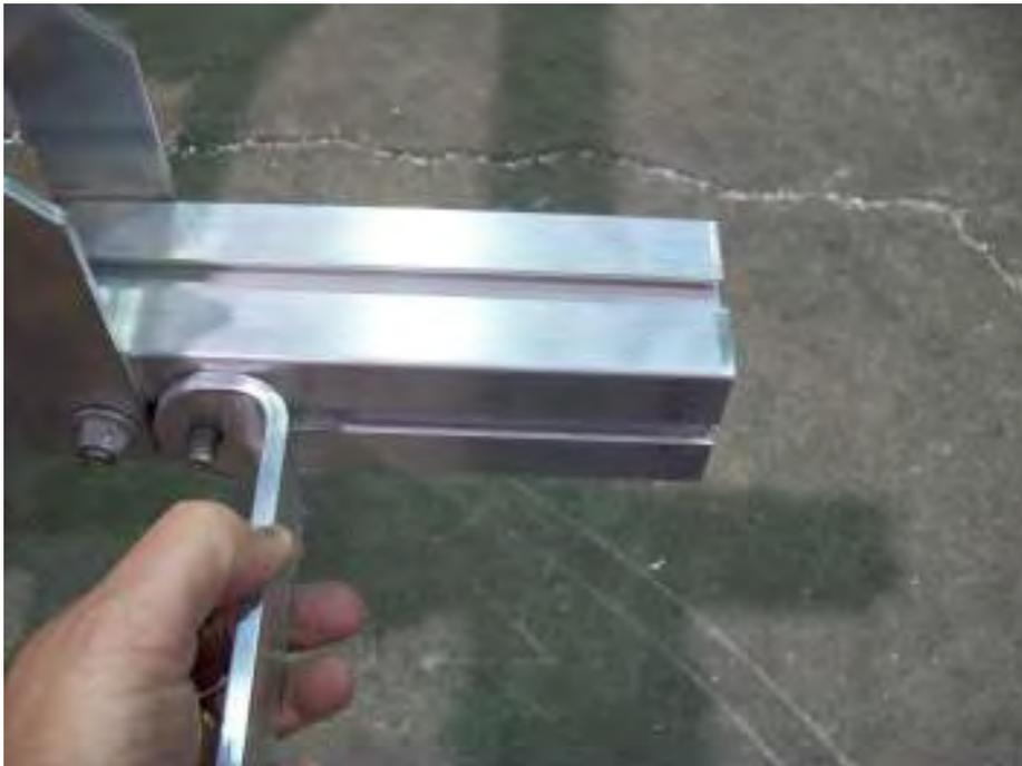
Install taillight brackets over T-bolts and butt up against angle brackets.
