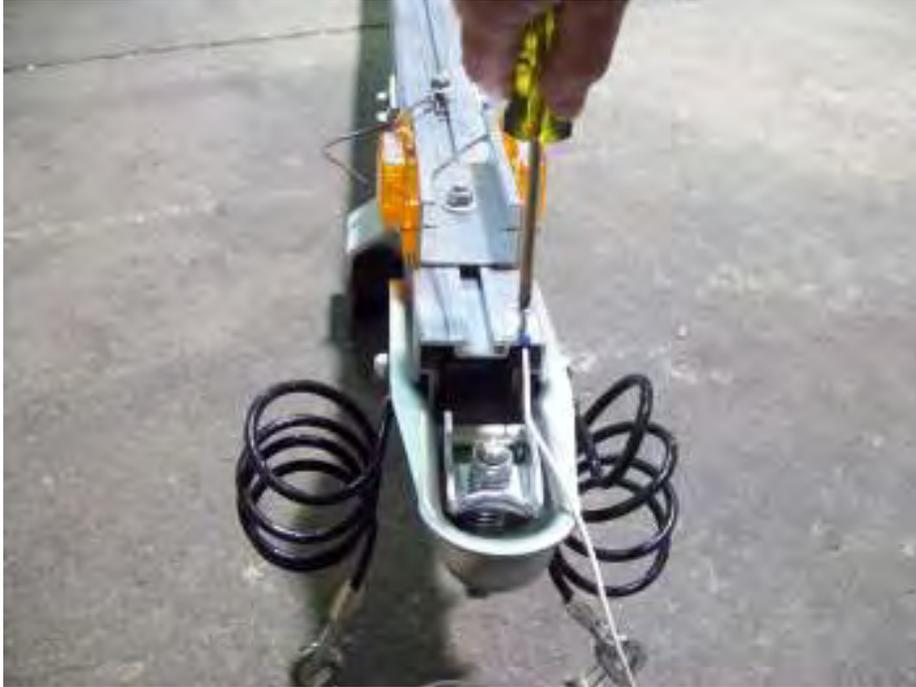
Install Philips screw through the ground wire into the pre-drilled hole located under the tongue just behind the coupler.
