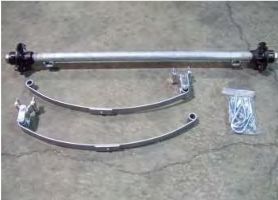
Locate the axle, spring assemblies and U-bolt kit.
