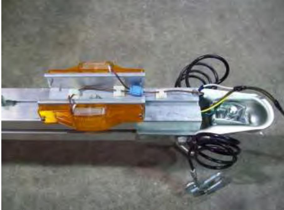
Locate the adhesive backed clamps. Install them as shown and run the brown wire from the running lights through them. Tuck the excess harness inside the tongue.
