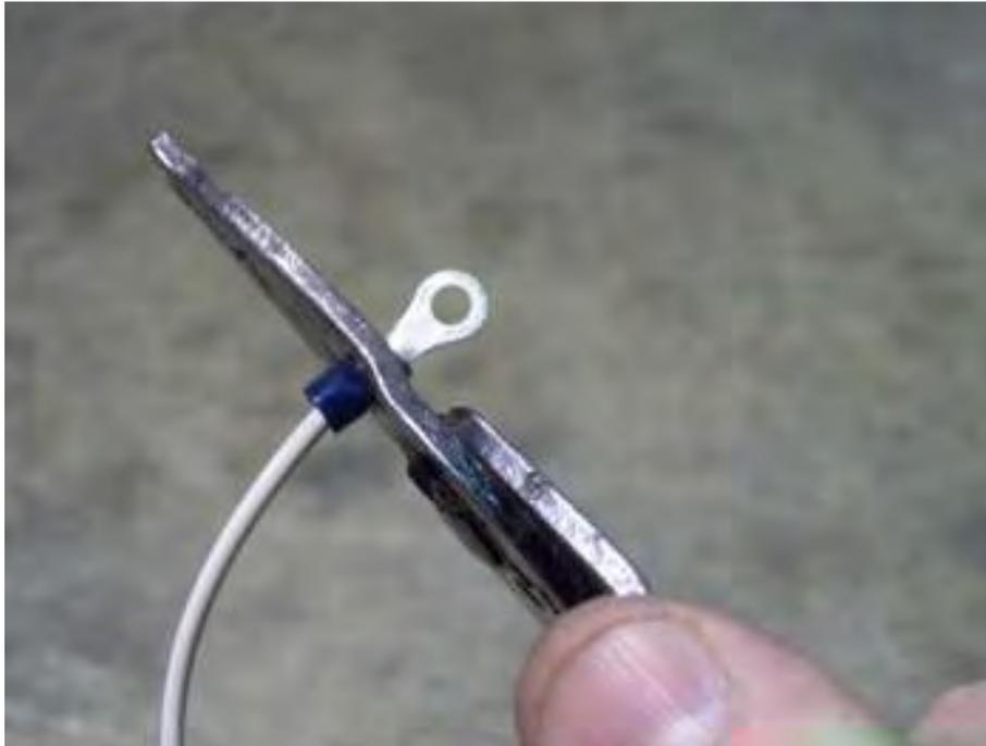
Take the white wire from the harness and strip a ¼” of the insulation from the wire. Install ring terminal by crimping it onto the bare wire.
