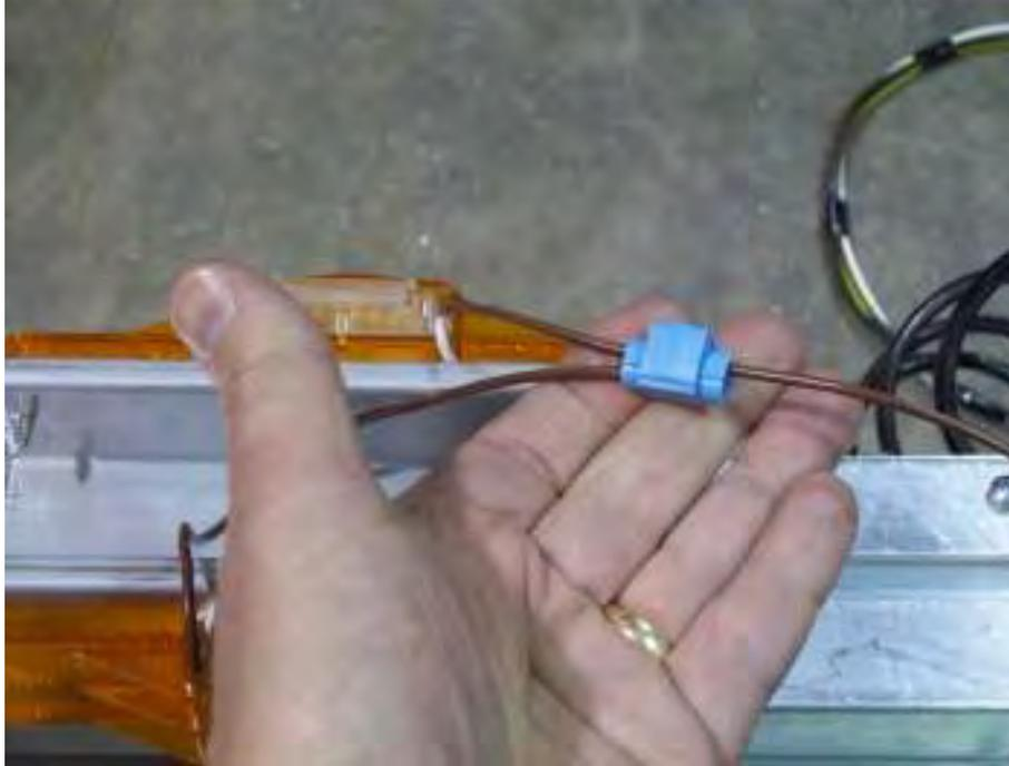
Close the plastic cover of the connector over the spade until it snaps into position.
