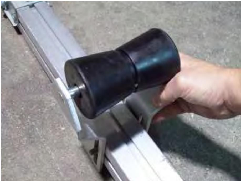
Pull the bracket over top of the other T-bolts to get in place.
