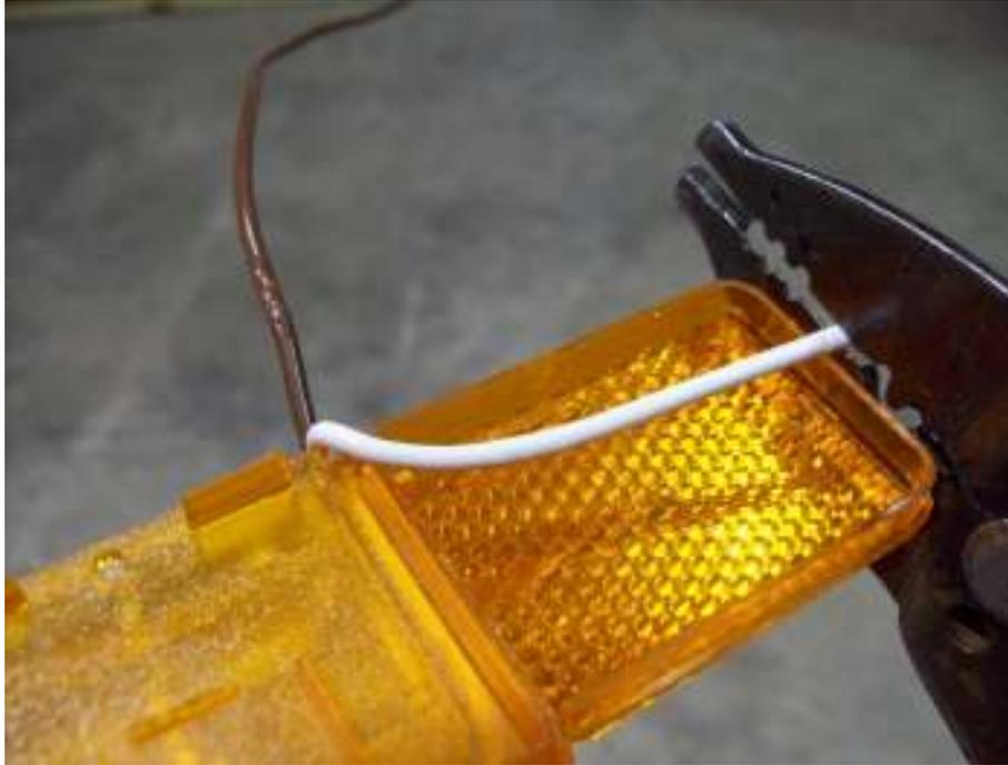
Cut approximately 8 ½” off of the white wires on both running lights.
