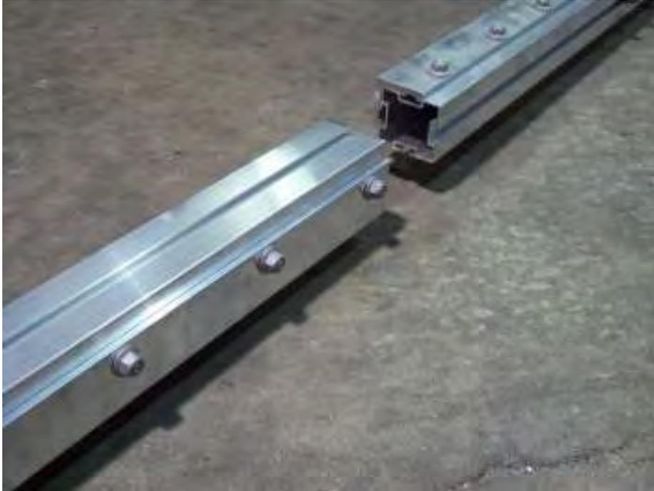
Lay the tongue sections end to end with the splice plates adjacent to each other.
