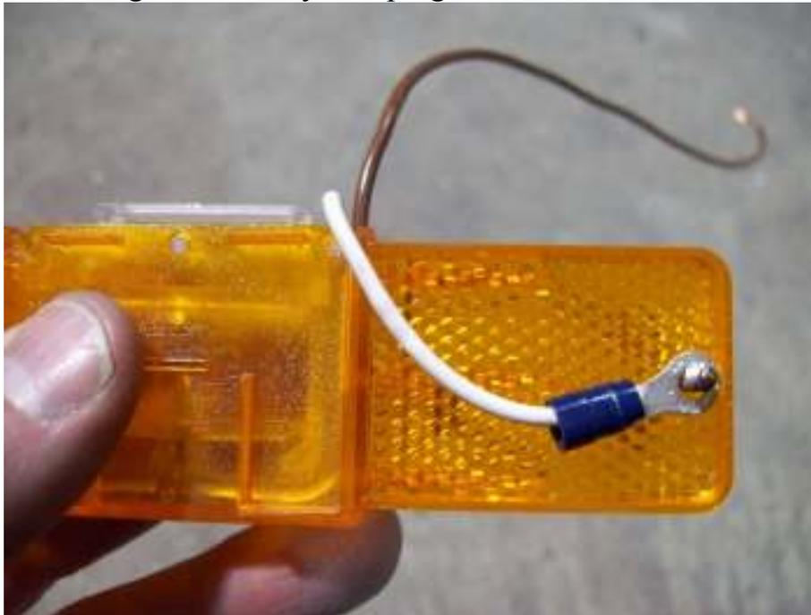
Align the ring terminals with the screw hole nearest the wire on the back of the running lights. Make sure the wire is routed through the gap on the back of the light so it does not become pinched when the light is installed.
