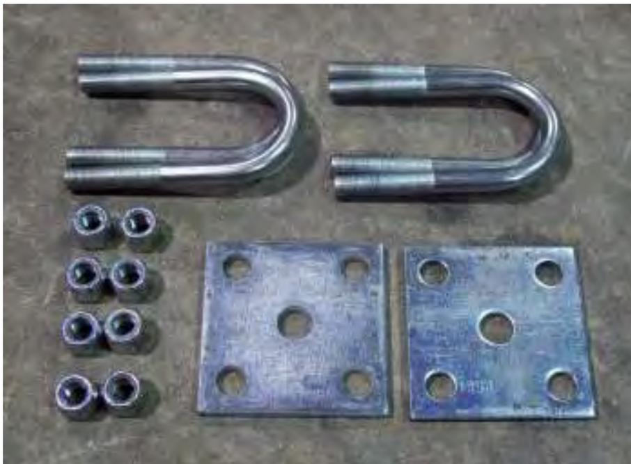
Locate the U-bolts, nuts and tie plates.
