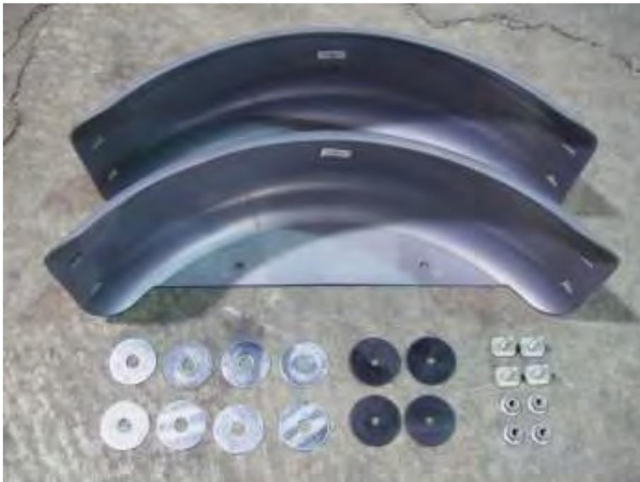
Locate the fenders, 8) large steel washers, 4) rubber washers, 4) 1 1/8" T-bolts and 4) nuts.
