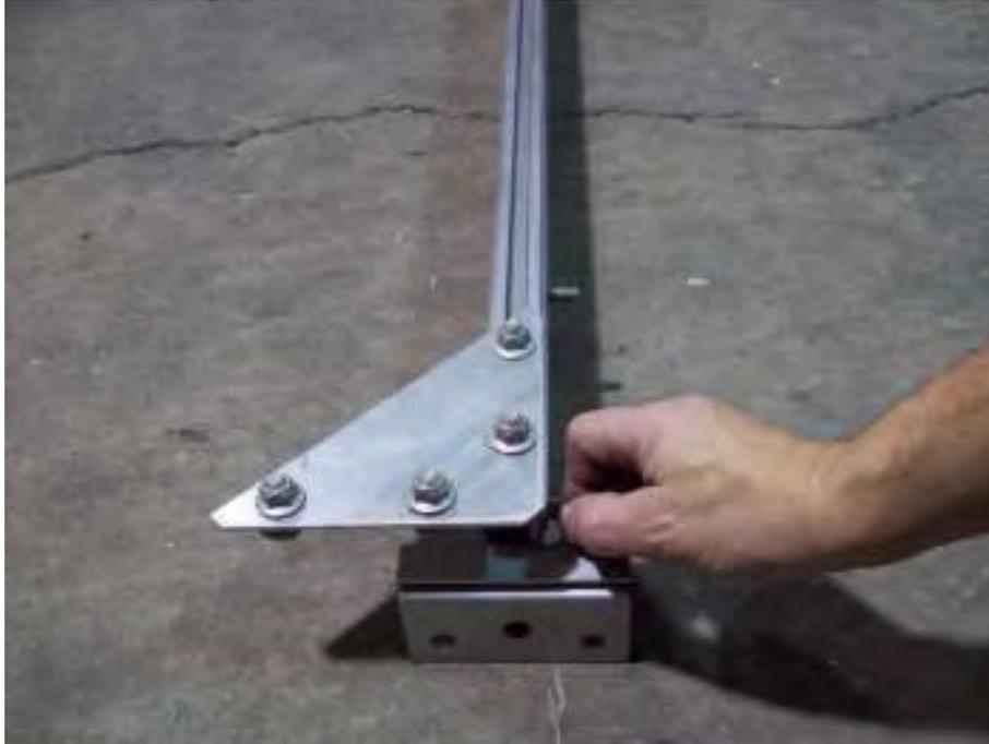
Install 2 T-bolts into the rear side of the rear cross member as shown.
