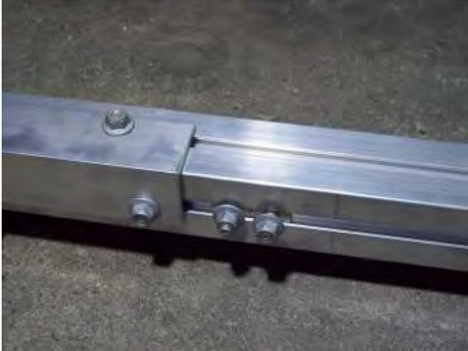
These T-bolts will be used to attach the front cradle holder later.
