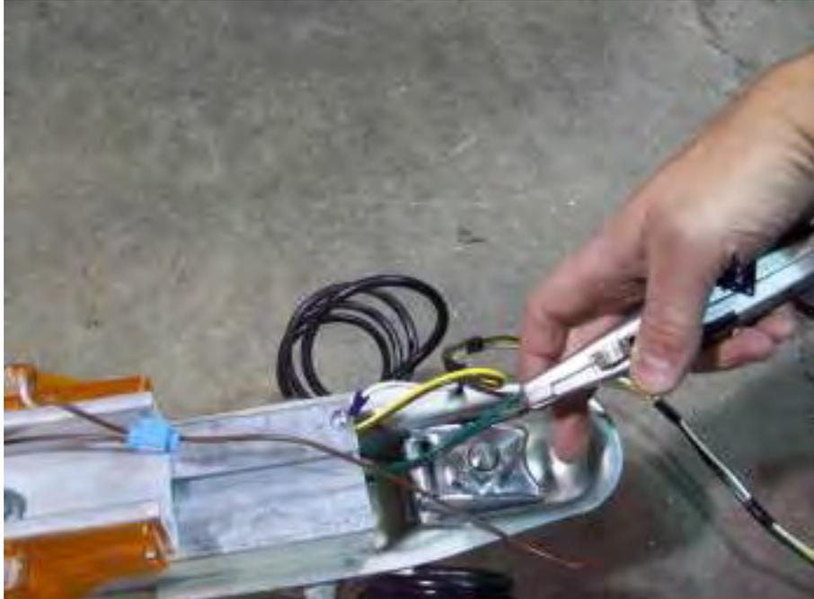
Measure 34" back from the front plug on the green/brown wire and separate the wires with a knife. Be sure not to cut through the casing.
