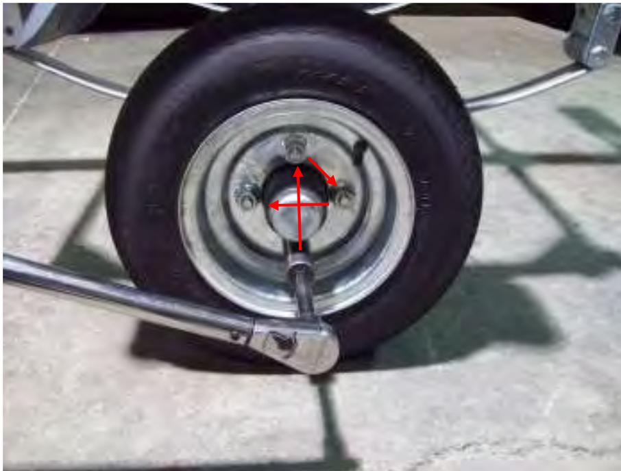
Tighten to 80 foot pounds in a crossing pattern. Re-tighten after 25 miles.
