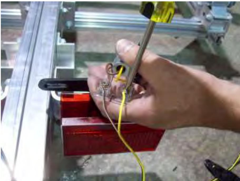
Loosen the retaining screws and install the color matching wires from the harness onto corresponding retaining screws. Tighten screws.
