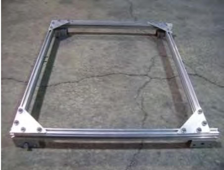
Your frame should look like this. Notice that the side rail extends past the rear cross member. If not assembled properly, the spring assembly will not have enough arch to work correctly.
