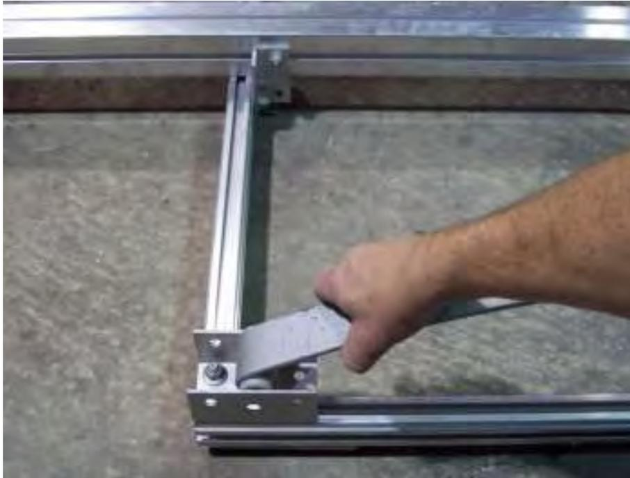
Install bushing into the front leaf spring and insert into the sub rail clip as shown.
