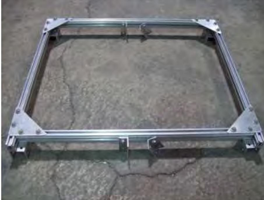
Your frame should look like this, with the angle brackets attached to the rear side of each cross members.
