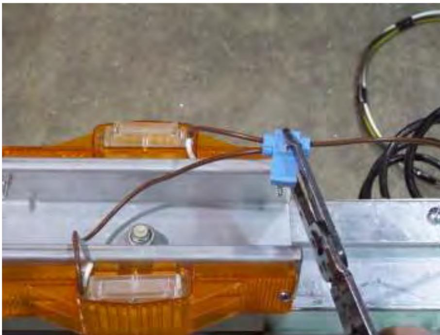
Use pliers to push the metal spade down until it is flush with the plastic. This is what makes the electrical connection between the two wires.
