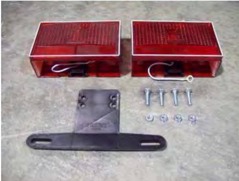
Locate the tail lights, license plate bracket, 4) carriage bolts and 4) nuts inside the light kit box.
