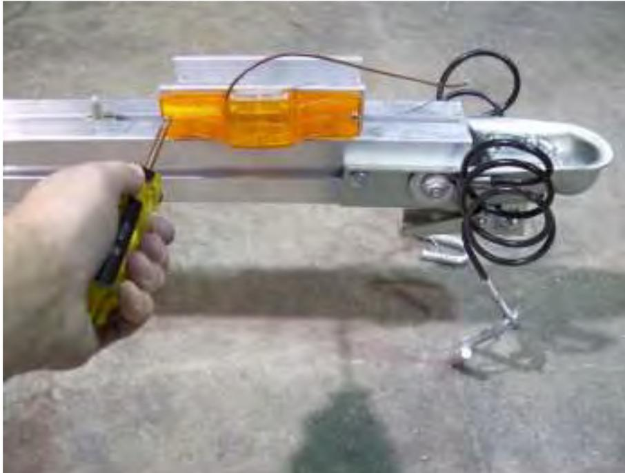
Install the running lights into the pre-drilled holes in the running light bracket using a Philips screwdriver. Be sure the screw is through the ring terminal on the back side of the lights. This will supply a ground to the lights.
