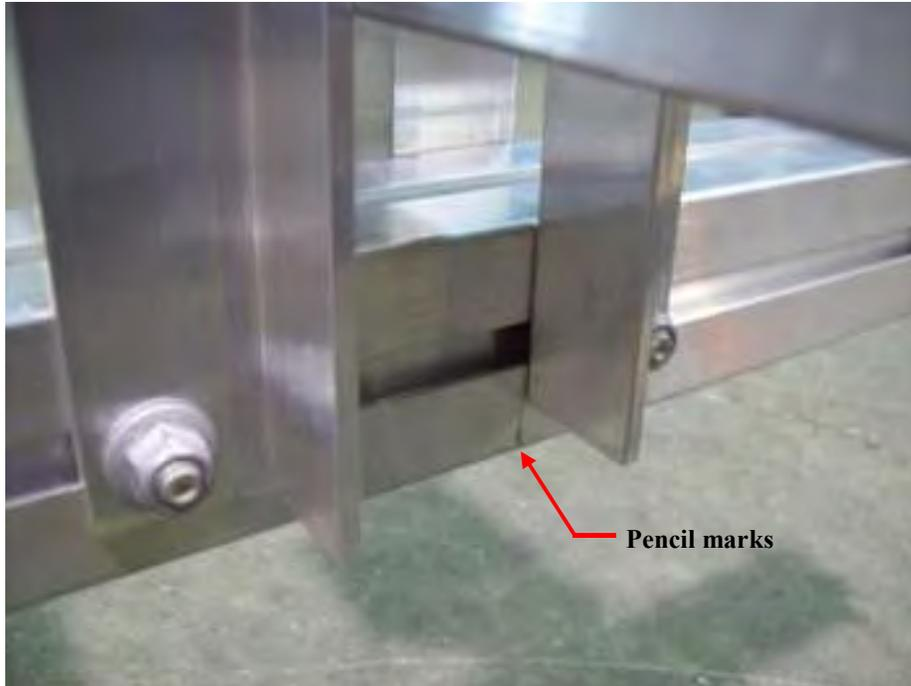
Make sure to align the back edge of the rear angle bracket with the pencil marks on the tongue. Once brackets are in position tighten nuts.
