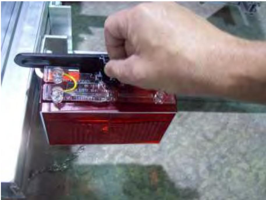
Move the tab toward the rear of the trailer and pull up, releasing the bulb assembly from the light housing.
