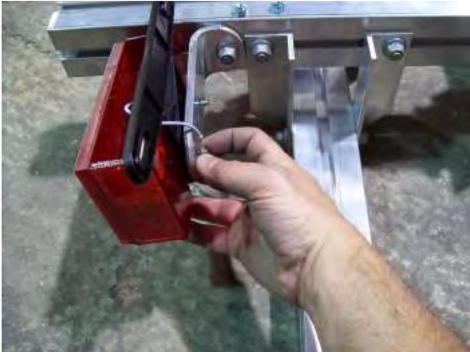
Install the white ground wire from the tail light onto the carriage bolt.
