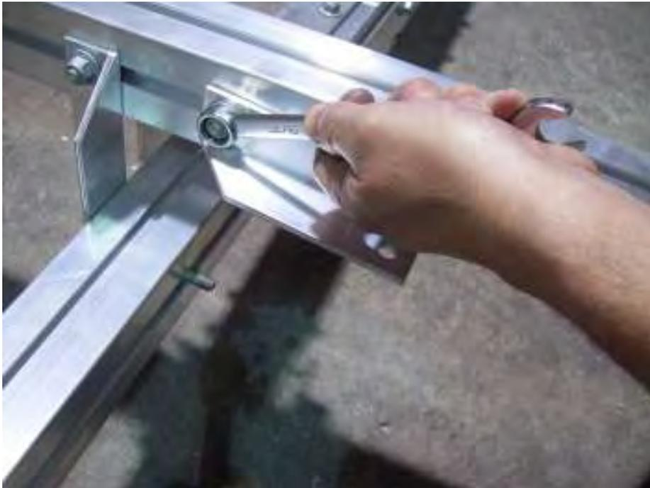
Loosen nuts on other side now and drop the angle brackets down over T-bolts.
