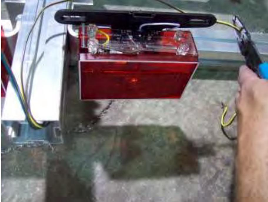
Trim off excess wire, leaving some for adjustment. Strip about a ½” of casing from the harness.
