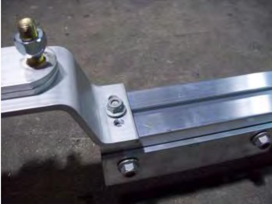
Loosen the T-bolts and nuts on spare tire carrier. Insert into the underside of the front tongue at the rear. Once T-bolts are in channel slide towards the coupler.
