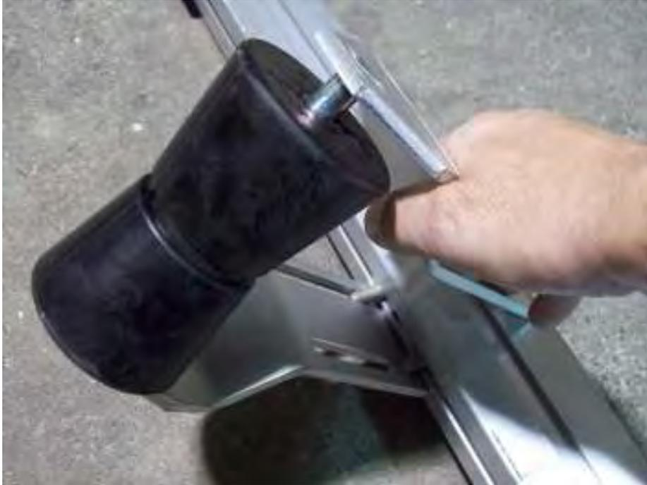
Tilt roller assembly to insert T-bolts into bracket as shown.
