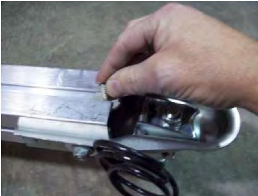
Insert the T-bolt into the slot at the front of the tongue section and slide out of the way. This will be used later to install the skid.
