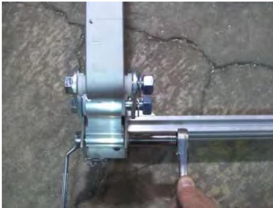
Remove the two bolts from the shackle holder at the rear of the spring and install the shackle holder into the rear sub rail clip, with the nuts toward the inside of the trailer. These nuts can be tightened at this time.
