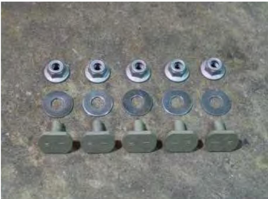
Locate 5)  $\frac{3}{4}$ " T-bolts, 5)  $\frac{3}{8}$ " flat washers, and 5) large flange nuts these are in the same bag with the web strap clips.
