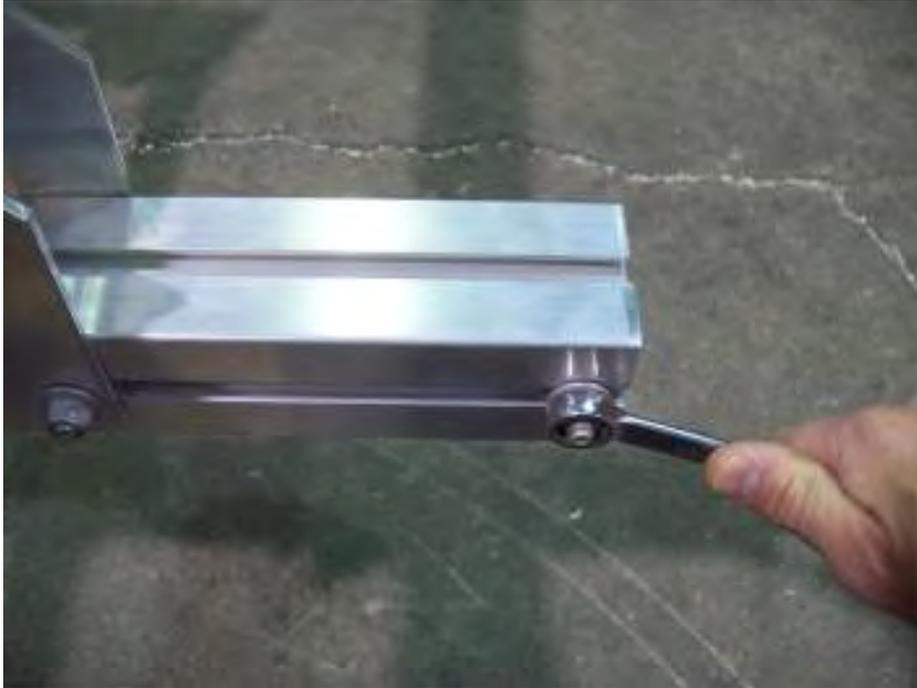
Loosen the last nuts on each side of the tongue section and slide them all the way to the angle brackets.
