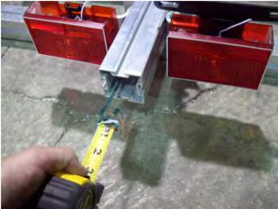
Retract the tape measure until it comes out the back of the tongue with both wires attached.
