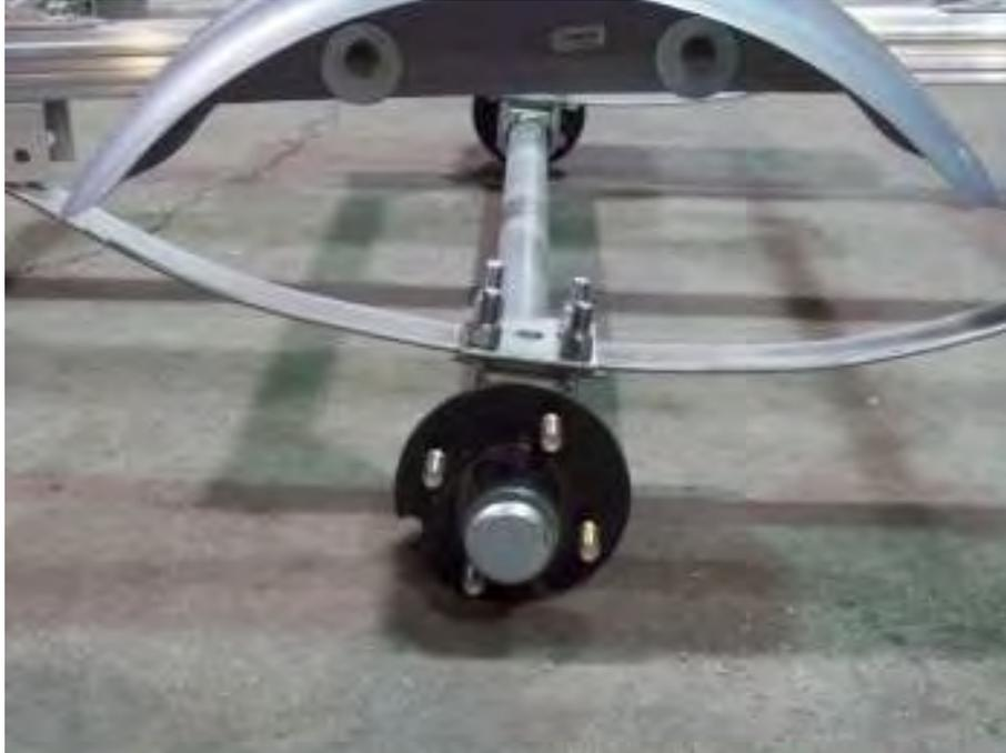
Install the fender, two more steel washers, and nuts, center the fender over the axle and tighten the nuts. Repeat for the other side.
