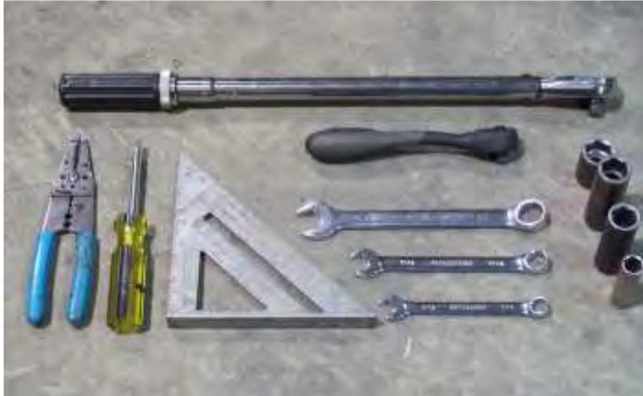
Torque wrench, carpenters square, wire cutters, Phillips screwdriver, 7/16, 9/16, and 3/4" combination wrenches, ratchet, 9/16, 3/4, 13/16", and 7/8" sockets.
