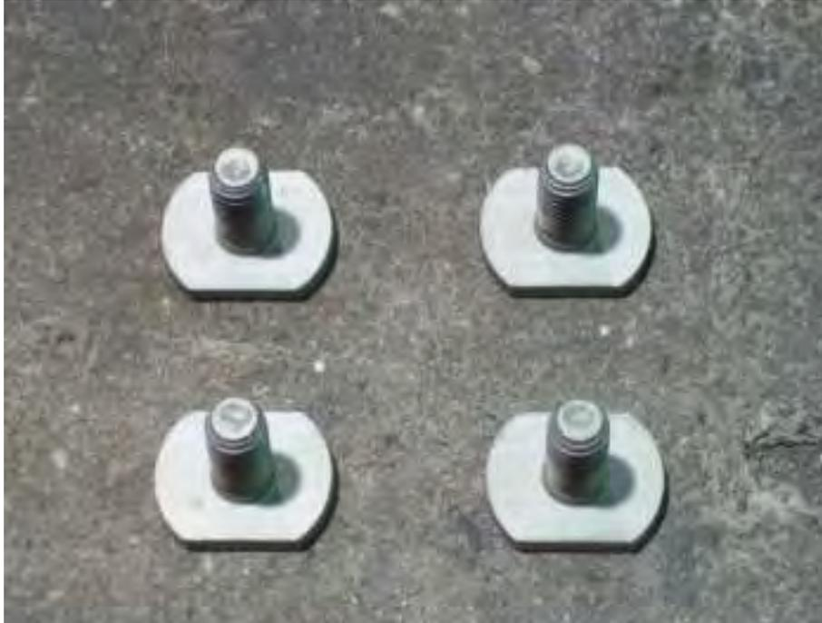
Remove 4 T-bolts from the hardware bag with the angle brackets.
