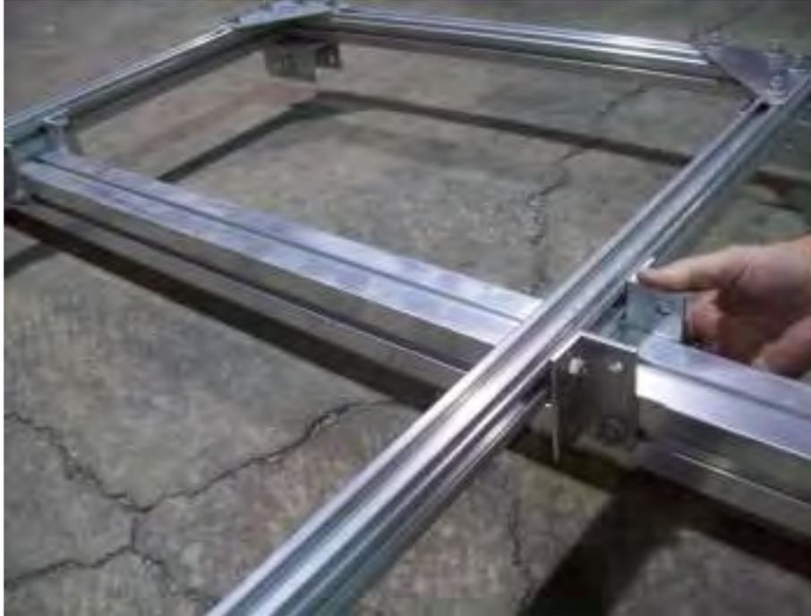
Slide the angle brackets from the right side over and install nuts.
