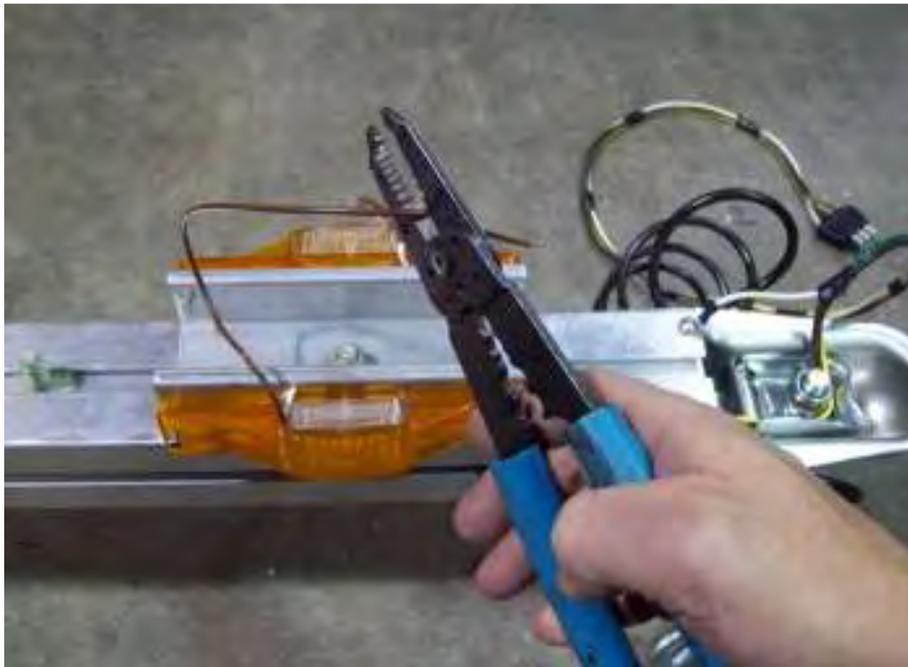
Cut about 2" off the brown wire on the left (driver's side) running light. Do not strip the wire.
