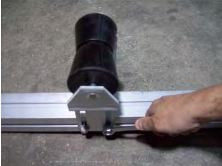
Reinstall nuts and tighten.
