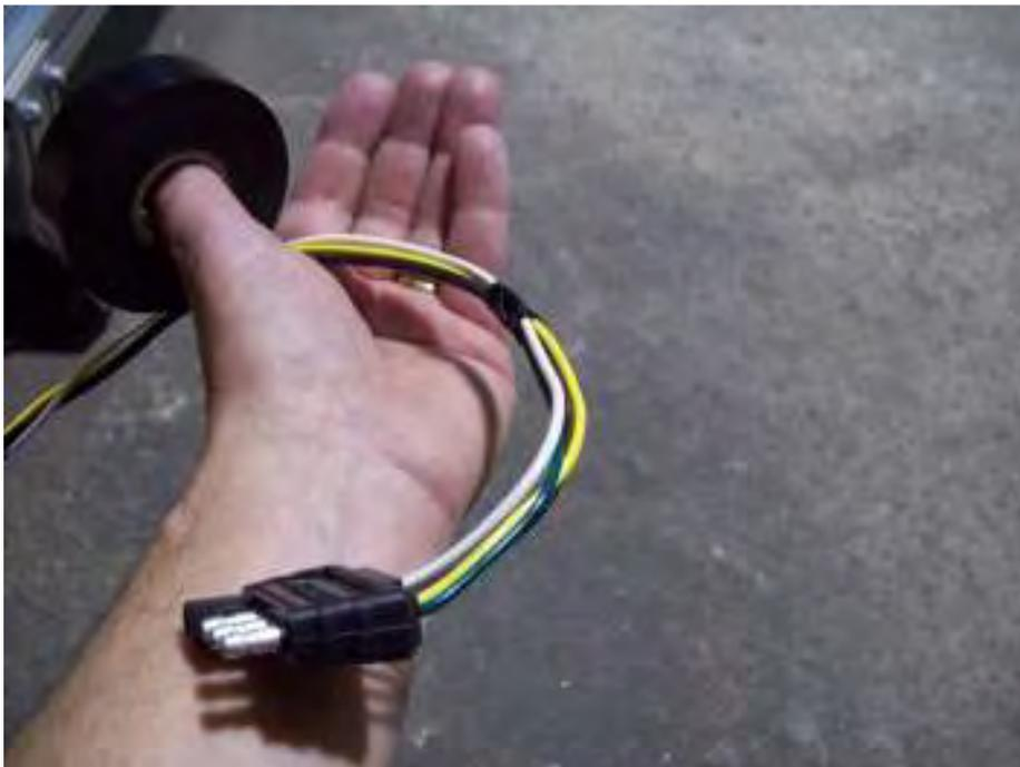
Start taping harness just past the four way connector with electrical tape and work your way down the ground wire to the tongue of the trailer. Usually space the tape about a hands length apart.
