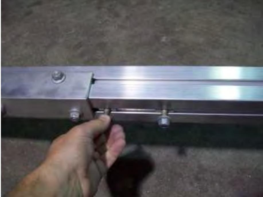
Remove the nuts from the T-bolts next to the splice plates on both sides of the tongue section.
