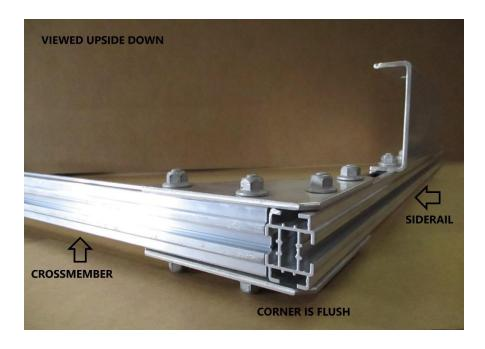
Next, slide the siderail, into the L-plates and make sure it is flush with the crossmember, as shown.
