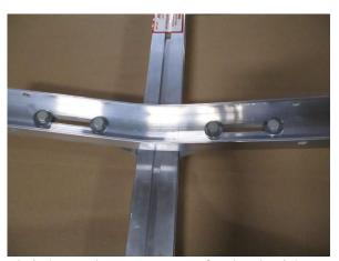
Slide the bolts out to each end of the slot, and tighten them. Repeat for both sides.
