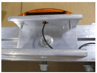
Install the marker light with the screws, as shown. Repeat for the other side.
