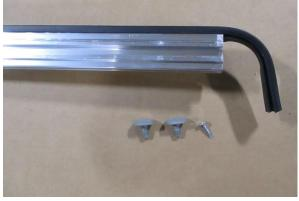
Using a Phillips screwdriver, remove the screw holding the vinyl down from one end of the guide rail and remove both T-bolts.
