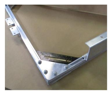
Complete one corner at a time starting with the front crossmember. Square that corner, and tighten the nuts on the top and bottom L-plates before moving on to the other side of the same crossmember. Repeat this process with each corner.
