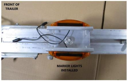
(Underside view of marker lights installed)
