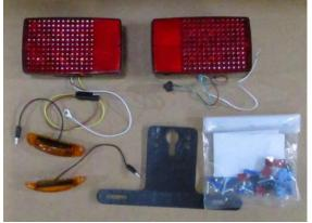
Locate the tail light kit box (**Part Q**), two tail lights, two marker lights, a license plate bracket, and a bag of electrical parts. NOTE: This is a universal tail light kit, some parts in the bag may not be used on your trailer.
