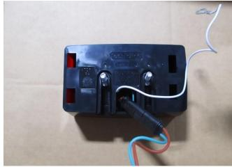
Carefully push the connector and the excess wire into the light before mounting, leave some slack so the wiring harness can go into the tongue once the lights are installed.
