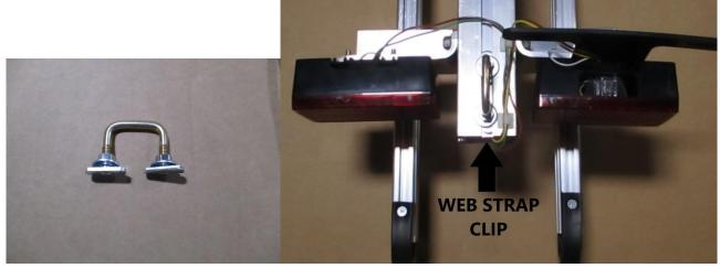
Locate a web strap clip from the hardware bag and install and tighten into the bottom slot of the tongue next to the wires.
