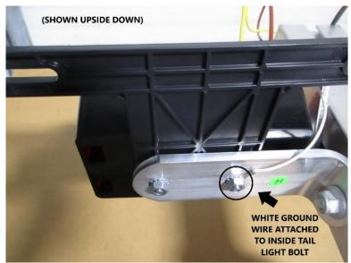
As with the right side, install the white ground wire and tighten the bolts.
