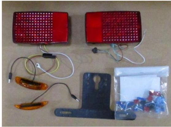
Locate the tail light kit box (**Part Q**), two tail lights, two marker lights, a license plate bracket, and a bag of electrical parts. NOTE: This is a universal tail light kit, some parts in the bag may not be used on your trailer.
