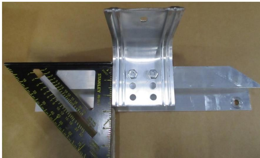
Before installing on the frame, square and tighten the fender braces together.
