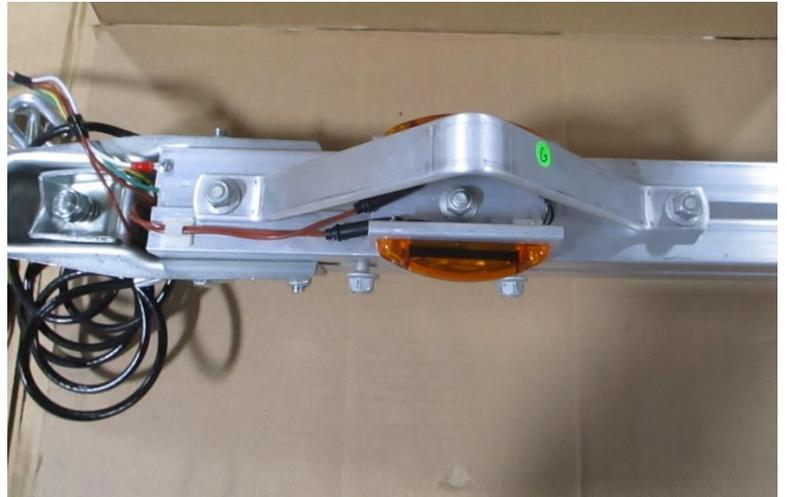
Next, mount the skid onto the tongue. Use the T-bolt installed from the previous step, and the one remaining on the skid. Center it over the marker light bracket, being careful to avoid the wires, and tighten.
