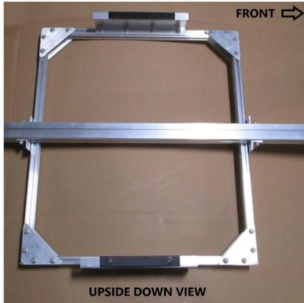
At this point, the trailer should look like this, with the frame mounted and the trailer upside down.
