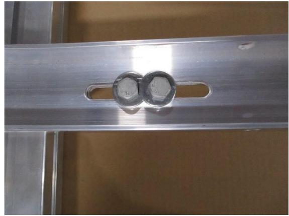
On the top of the cradle holder, make sure the slot is lined up with the bracket underneath.
