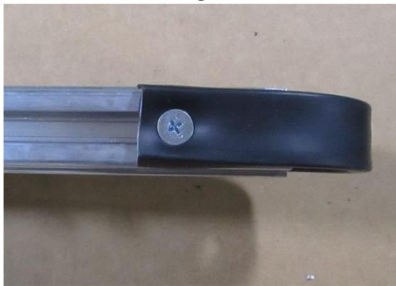
Re-install the vinyl, line up the hole, and re-install the screw. **Do not overtighten.** Repeat for the other guide rail.
