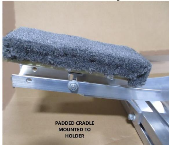
Install the padded cradle inside the cradle holder, slide the 2 3/4" bolt through the cradle holder and the pivot plate on the padded cradle, install the nut and tighten. (Shown mounted to the inner position. The final position will be determined when the boat is fitted to the trailer.)
