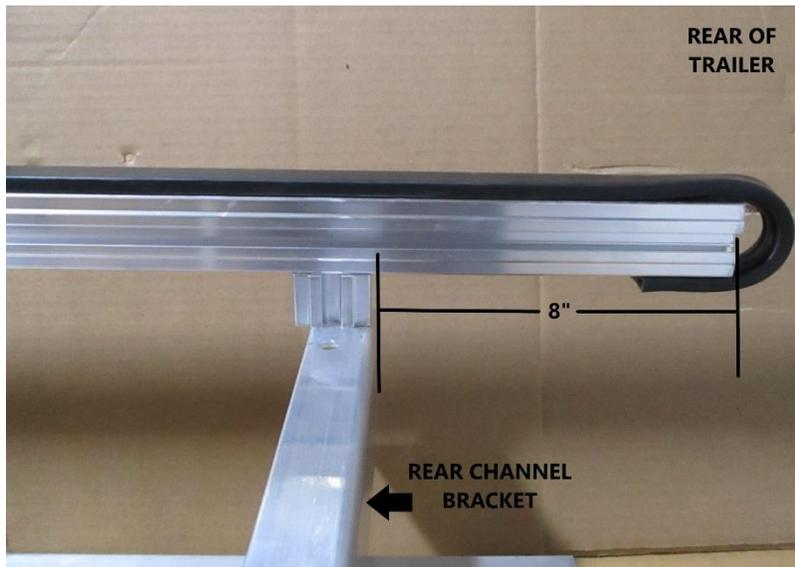
Install the guide rail, in the **outer** holes, 8" away from the rear of the rear channel bracket. Repeat for the other side, then tighten the guiderails to the front and rear channel brackets.
