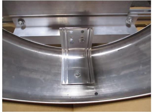
Mount the bolt through the fender and brace as shown.
