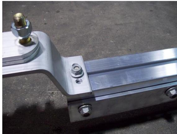
Loosen the T-bolts and nuts on the spare tire carrier. Insert into the underside of the front tongue section, at the rear. Once the T-bolts are in the channel, slide it toward the coupler.
