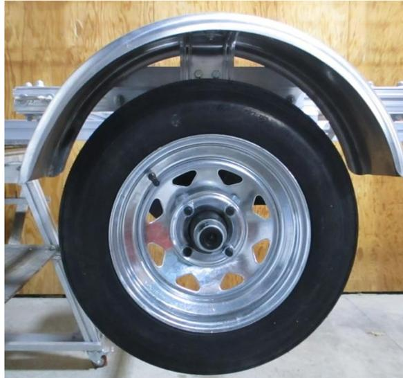
Install the tires and wheels with the valve stems facing out. Install the lug nuts with the tapered side toward the wheel.
