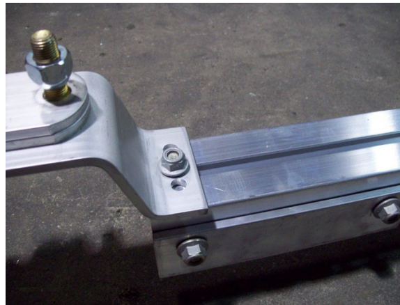
Spare Tire Carrier for SUT Trailers
