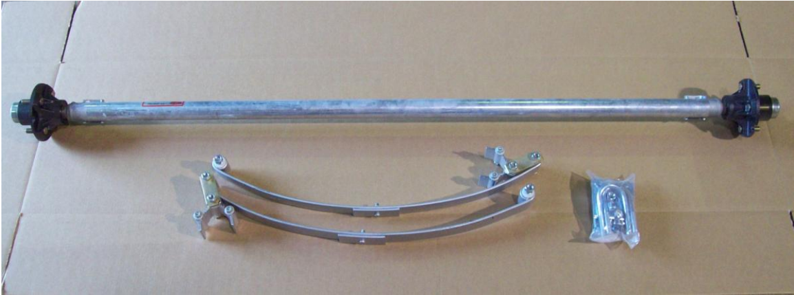
Axle assembly, springs and U bolt hardware.
