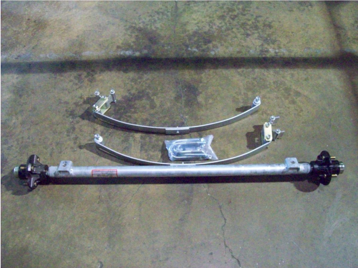
Axle assembly, springs and U bolt hardware.
