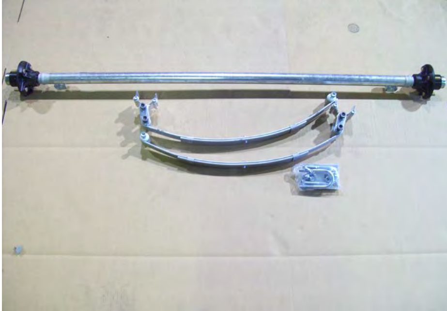
Axle assembly, springs and U-bolt hardware.
