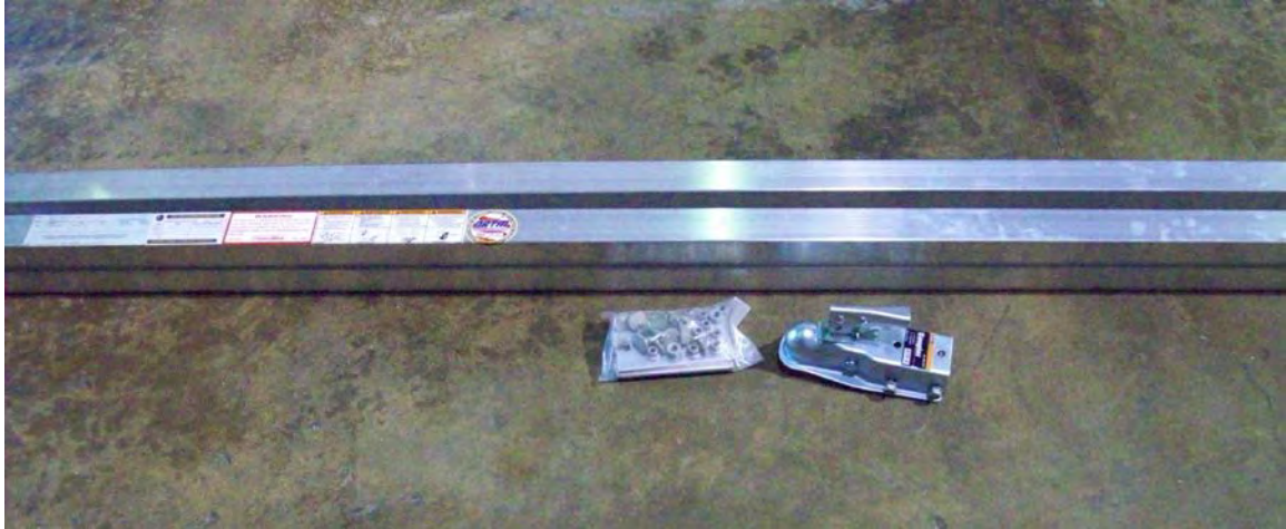
Tongue sections, splice plates, and coupler.
