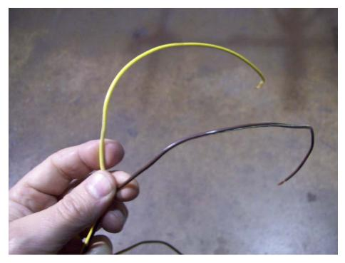
Take the left over wire from the harness that was cut off and separate the two wires. The brown wire will be used to connect the clearance light to the tail light.
