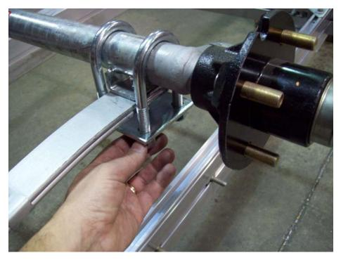
Install the U-bolts and tie plates as shown.
