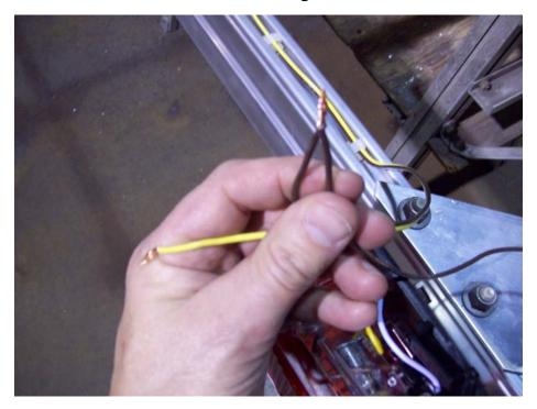
Twist the brown harness wire and the brown clearance light wire together.
