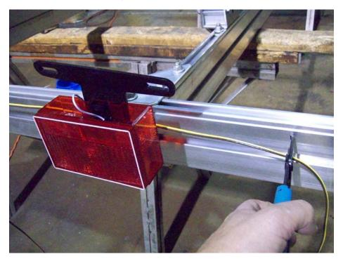
Trim off excess wire leaving some for adjustment. Keep the excess wire. It will be used later to connect the clearance lights.
