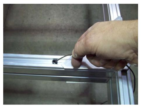
Run the wire from the clearance light down the cross arm to the side rail. Insert the wire into hole in the side rail and push wire towards the rear hole.
