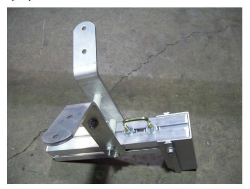
Bow stop should look like this when installed on the winch post.
