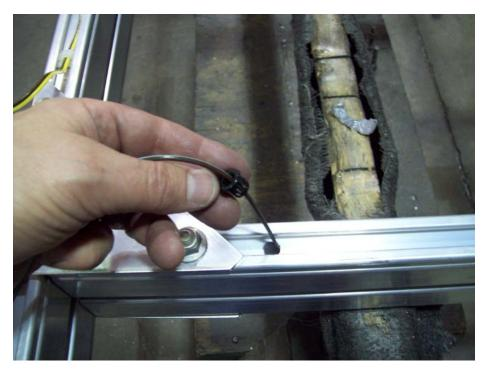
Insert wire through snap bushing and push into hole.
