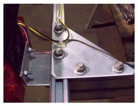
Reinsert housing and tuck wires in. Add adhesive clip to hold wires down on triangle plate.
