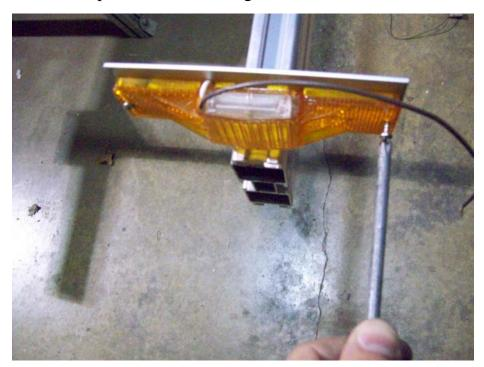
Install the running lights into the pre-drilled holes in the bracket using a Philips screwdriver. Be sure the screw is through the ring terminal on the back side of the lights. This will supply a ground to the lights. <u>DO NOT OVER TIGHTEN.</u>
