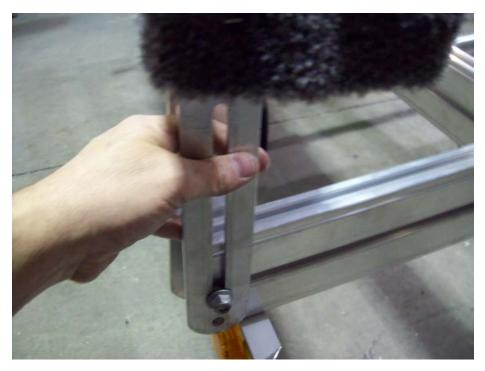
Insert T-bolt from slotted bracket into the front and rear cross arm. Slide cradle assembly towards the side rails.
