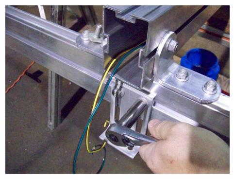
Center the slotted bracket under the tongue section and tighten nuts.
