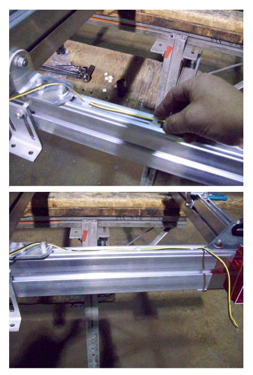
Insert adhesive clips in the rear cross arm as shown, and run harness towards the light. Repeat the process for other side.
