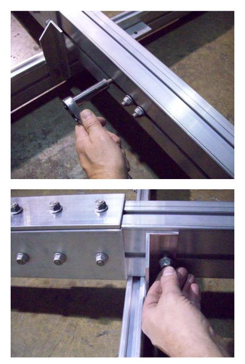
Remove the rearmost nut in the front tongue section and insert the T-bolt into the angle bracket. Reinstall nut and tighten.
