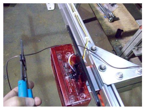
Remove excess wire for the clearance light, and trim off a <sup>1</sup>/<sub>4</sub>" of casing.
