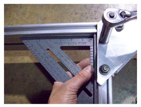
Square up the side rail and rear cross arm then tighten all the nuts. Repeat this process for the other side.
