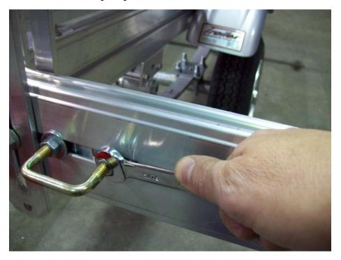
Slide all the way over to the slotted bracket, and tighten nuts.
