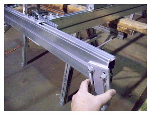
Install the slotted bracket into the back side of the rear cross arm.
