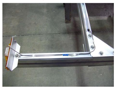
Insert adhesive clips into the cross arm and run harness through them as shown.
