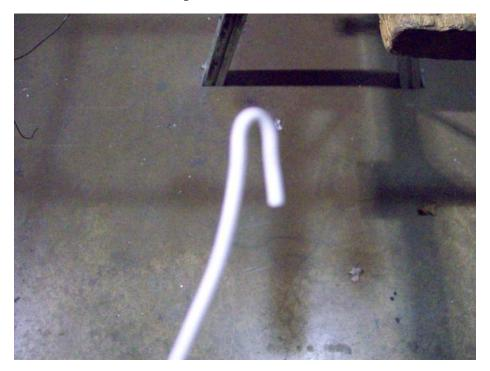
Using scrap wire, make a hook to pull the wire through the rear hole.
