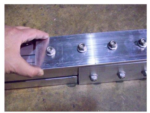
Align the rear tongue section with splice plates to the back edge of the front tongue section. Once in position, slide the bottom splice plate over and center it.
