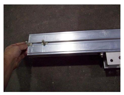
On the outward part of the side rail insert two 1 1/8" T-bolts. These will be used later to install the fenders.
