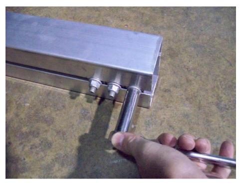
Loosen nuts on both sides of the front tongue section and slide them forward. These will be used later in the assembly process. There should be three on each side.
