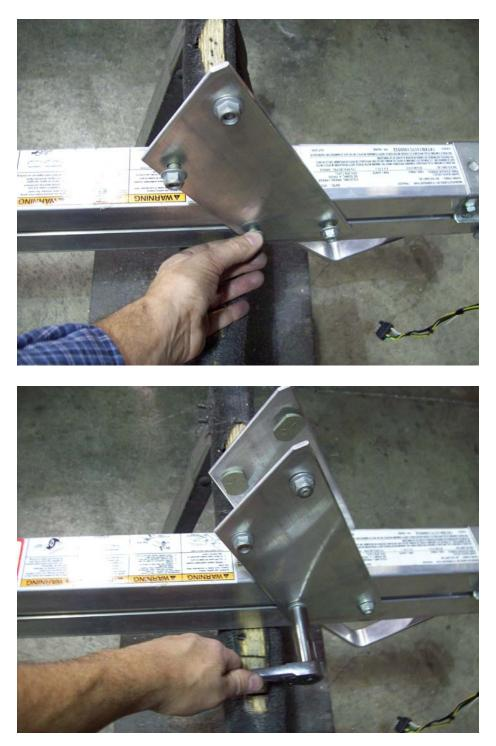
Install winch post diagonal braces on each side of the tongue section. Reinstall nuts and tighten. Final positioning will be made later to accommodate your boat.
