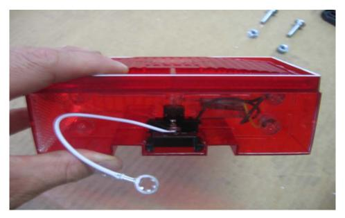
The light with the yellow wires is for the left (driver's side) of the trailer.
