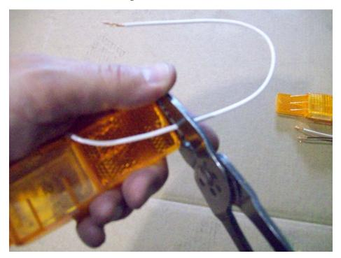
Cut approximately 8 <sup>1</sup>/<sub>2</sub>" off of the white wires on both running lights.
