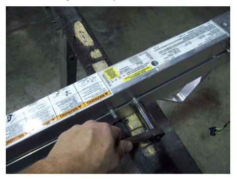
Slide the two remaining T-bolts on each side of the tongue section towards the coupler. Remove nuts on both sides.
