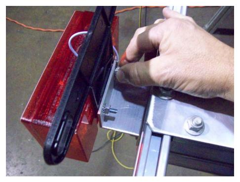
Install the left tail light with the license plate holder between the light and the bracket. Repeat for the other side. Make sure to tighten nuts but don't over tighten them. (Pictured from the bottom)
