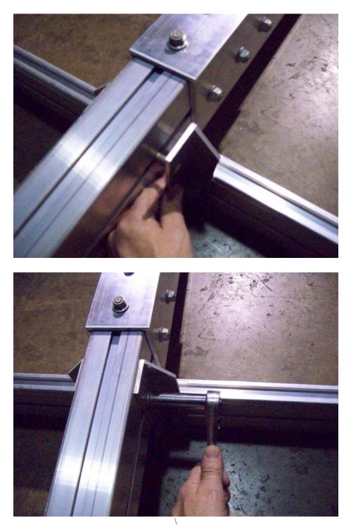
Loosen the other angle bracket, slide over and install on tongue section. Square up and tighten nuts.
