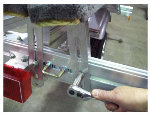
Install the outer cradle assembly, position and tighten nuts. Final adjustments will be made when the boat is fitted to the trailer.
