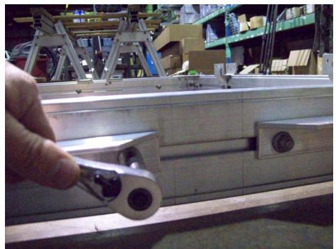
**Frame shown upside down** Turn frame upside down and loosen angles on front cross arm.
