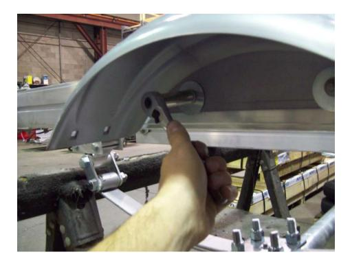
Tighten the nuts and repeat process for the other side.
