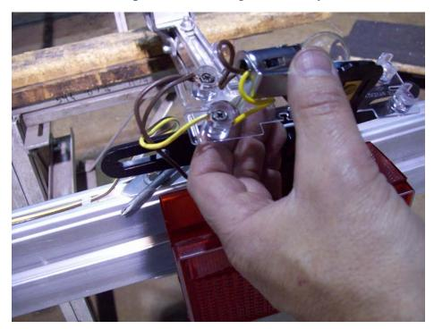
Once out of housing, color match wires with the ones on the terminals as shown.
