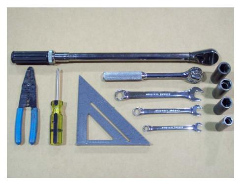
Torque wrench, carpenters square, wire cutters, Phillips screwdriver, 7/16, 9/16, and 3/4" combination wrenches, ratchet, 9/16,3/4,13/16", and 7/8" sockets.
