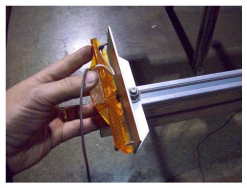
Align the ring terminal with the screw hole nearest the wire on the back of the running light. Make sure the wire is routed through the gap on the back of the light so it does not become pinched when the light is installed.
