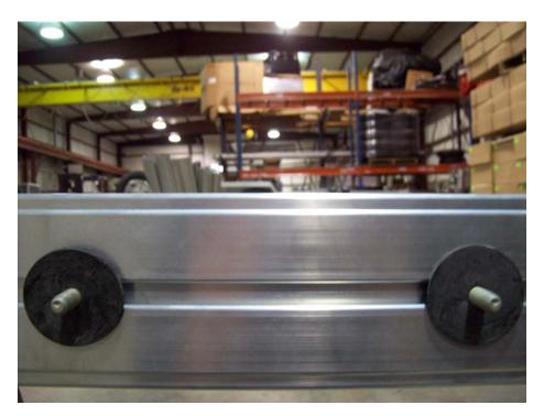
Return the trailer right side up. Slide the 1 1/8" T-bolts installed previously on page 9 into position over the axle and install two rubber washers as shown.
