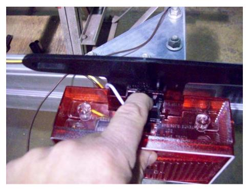
Pull black tab on the underside of the light towards the back of the trailer and up. This will release the internal portion of the light assembly.
