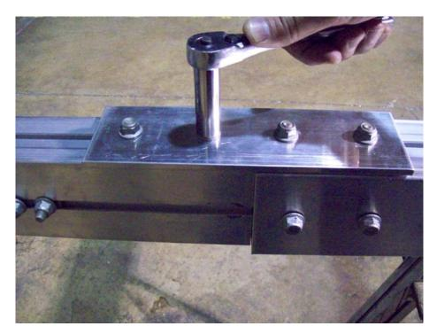
Tighten nuts on the bottom splice plate. Also, make sure there is no gap between the two tongue sections.
