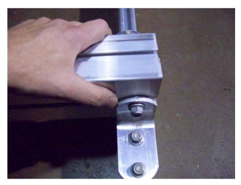
Insert rear tongue section into the angle brackets on the rear cross arm as shown.
