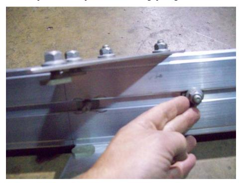
Locate the rear cross arm. On each side there are two T-bolts and nuts. Remove the outer nuts on both ends. The two inside T-bolts are extra to be used when inner bunk brackets are moved closer together.
