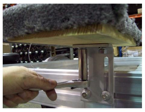
Install transom board on slotted bracket, reinstall hardware and tighten nuts.
