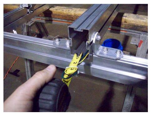
Retract the tape measure until it comes out the back of the tongue with both wires attached. The wiring will be completed later. Trailer is still upside down.
