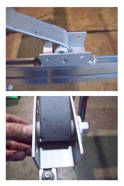
Remove the bolt from the front spring eye and install the spring into the spring hanger in the center hole with the nut toward the inside of the trailer. Do not tighten yet.
