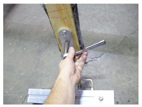
Install the bow pads on the mounting brackets. Reinstall nuts and lock washers and tighten nuts.
