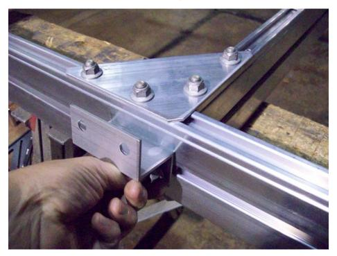
Insert the tail light brackets over the two T-bolts and install nuts.
