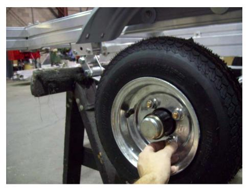
Install the wheels with the valve stems facing out. Install the lug nuts with the tapered side facing the wheel.
