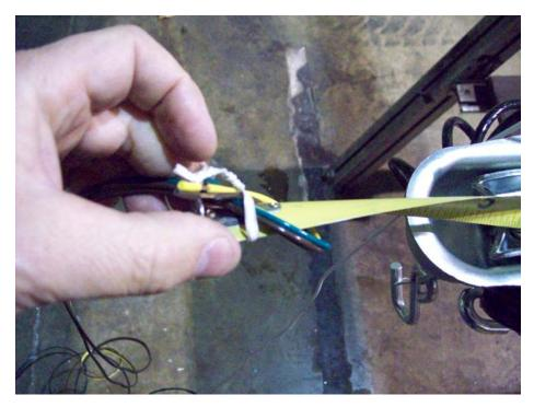
Attach both wires of the harness to the end of the tape measure with either tape or a tie.
