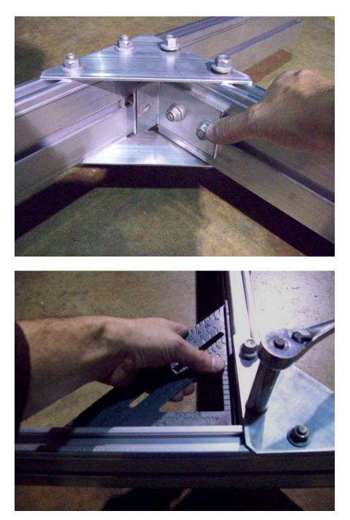
Insert the front cross arm into both of the side rails. Make sure the side rail and front cross arm are square and tighten nuts.
