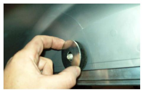
Install the fender, rubber washer, steel washer, and nut, over each bolt. Center the fender over the axle.
