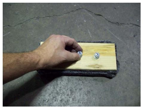
Remove the nuts and lock washers from the bow stop.
