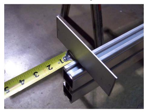
Insert bracket into front cross arm and position 1" from the end
