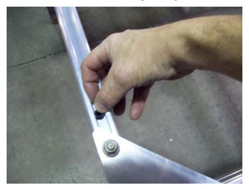
Insert the snap bushing in the hole at the front of the side rail.
