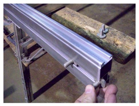
Install two T-bolts on each side of the back side of the rear cross arm.
