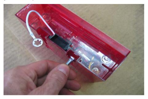
Slide the carriage bolts into the slots in the back of the tail lights.
