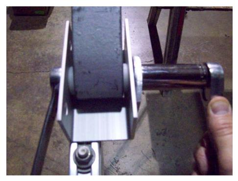
Go back and tighten all of the spring mounting nuts that were left loose previously. Do not over tighten the bolt on the rear shackle as this will not allow the suspension to move properly.
