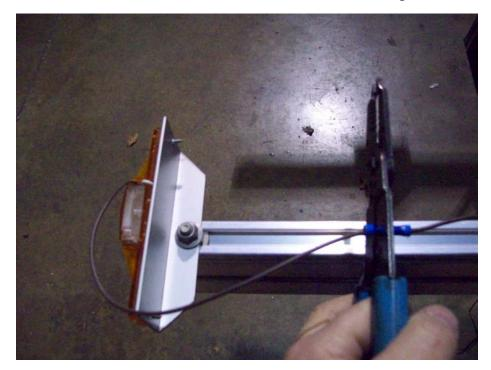
Before attaching the brown wire to the running light make sure it will reach the rear tail light. Trim a 1/4" of casing off both ends of the wires and crimp a butt connector on.
