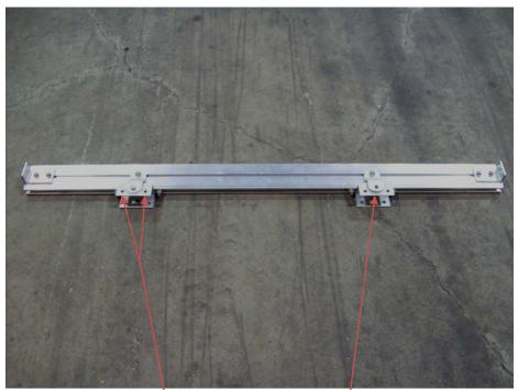
**Rear sub rail clip** Inside of side rail shown Front sub rail clip Rear sub rail clip has two outer holes to accept the shackle assembly. In the front sub rail clip, the center hole is open to accept the spring bolt.
