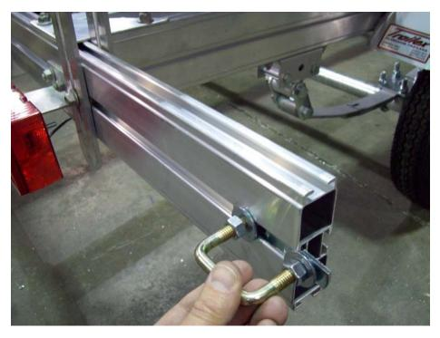
Insert web strap clips on each side of the rear cross arm.
