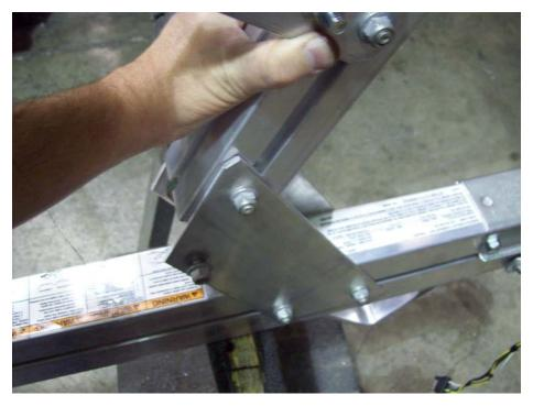
Insert winch post assembly into the T-bolts in the diagonal braces as shown.
