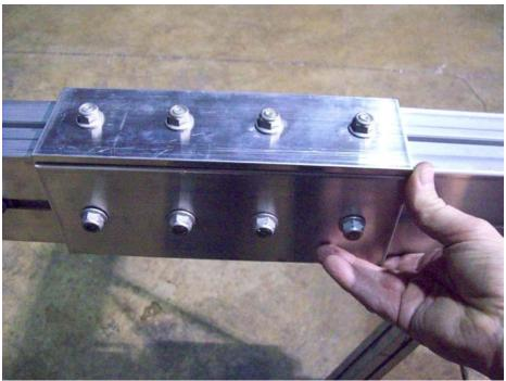
Shown up side down At this point slide both side splice plates over and center.
