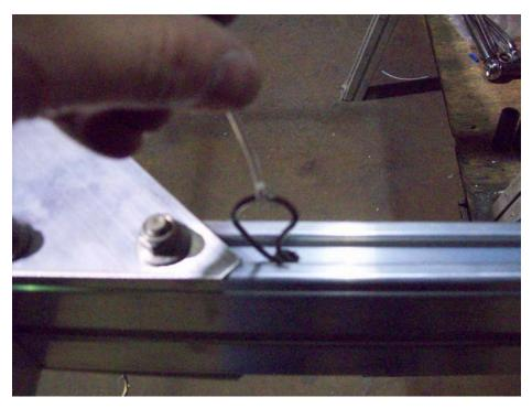
Hook the wire at the rear hole and pull it through.
