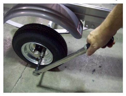
Tighten to 80 foot pounds in a crossing pattern. Re-tighten after 25 miles.
