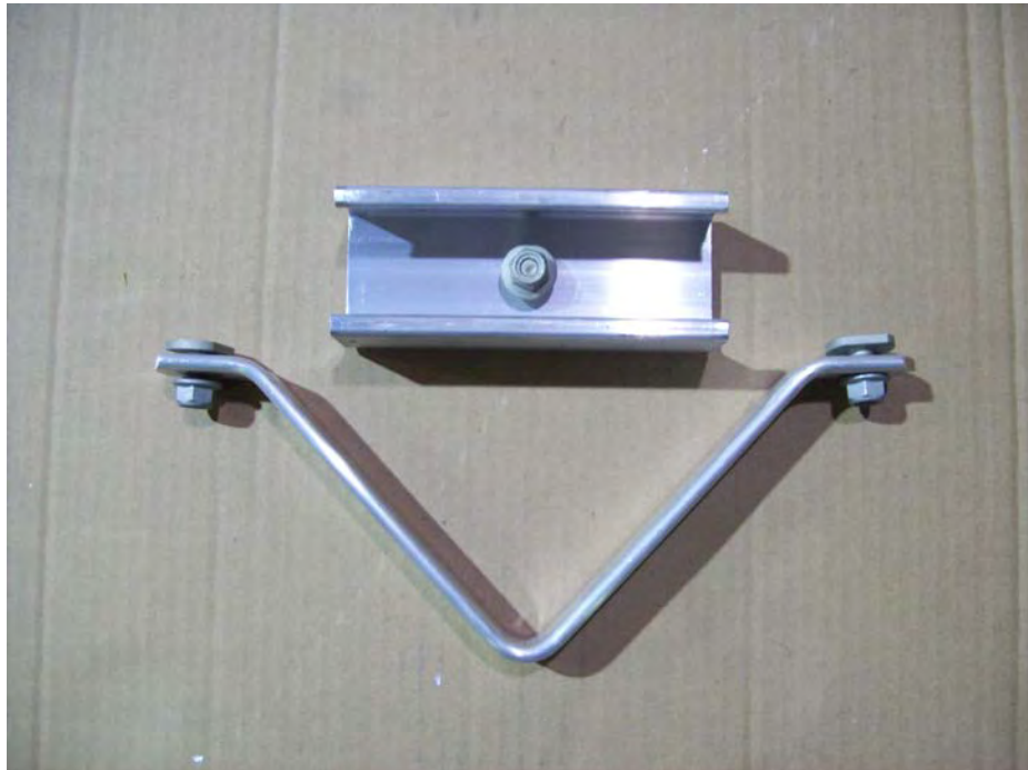
Skid and side marker light bracket
