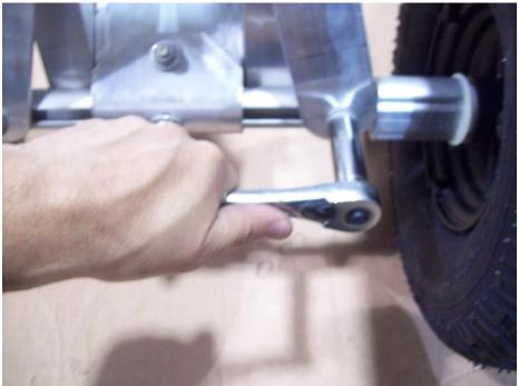
Slide axle struts towards the tires to take up any slack in the assembly then tighten nuts.
