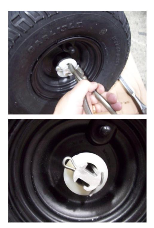
Bend the ends of the cotter pin up with a pair of pliers as shown. Then repeat this process for the other side.
