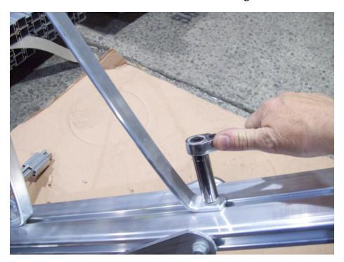
Position the back of the skid with the tongue struts as shown.
