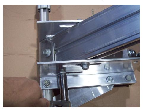
Once in position tighten the nuts on both sides and the U plate.
