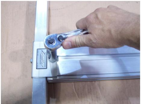
Install handle into tongue section then tighten nuts.
