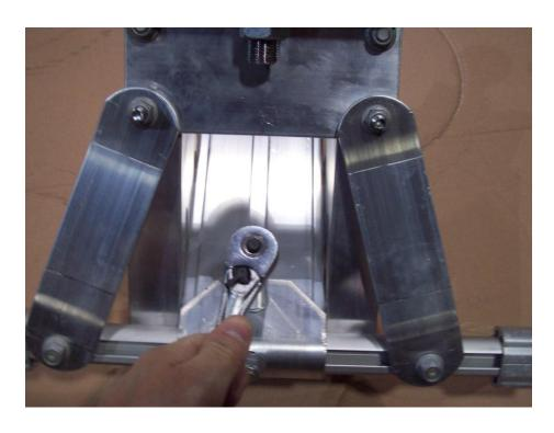
Also, be sure to tighten the nut on the front side of the U-plate.
