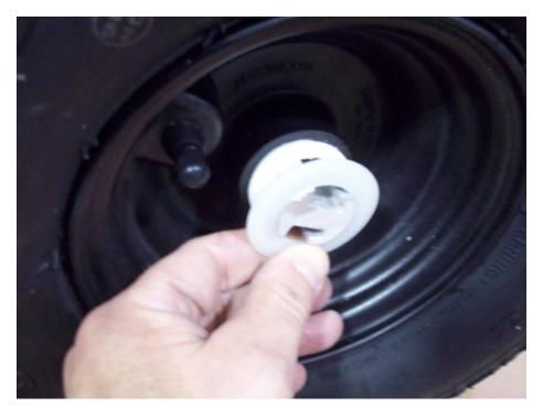
Install the tire on axle then insert the grooved side of bushing facing inward.
