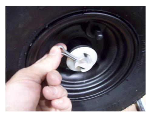
Insert cotter pin through hole on the axle.
