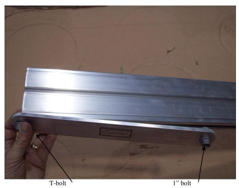
Install the tongue strut with the T-bolt at the one end into the tongue as shown. The 1" bolt at the other end will attach to the angle brackets at the front of the dolly.
