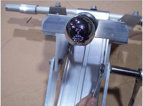
Install the tongue strut on assembly as shown then repeat for the other side. When finished go back and tighten nuts.
