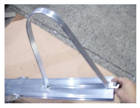
Insert the skid on the underside of the tongue as shown.
