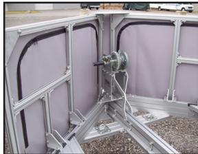
Winch, Front Shield, Recessed "D" Rings
