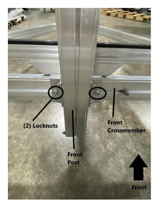
With the (2) arm brackets installed, the (2) locknuts holding the front post will need to be tightened. Tighten the (2) locknuts using a 9/16" wrench.
