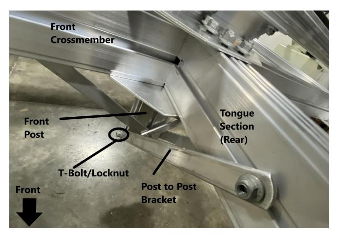
The front post will have (2) T-bolts and locknuts installed in the side grooves. Remove the (2) locknuts using a 9/16" wrench. Install the (2) post to post brackets to the front post as shown, using the T-bolts installed in the side grooves of the front post. Replace the (2) locknuts and tighten using a 9/16" wrench. Once complete, tighten the (2) locknuts holding the (2) post to post brackets to the rear tongue section using a 9/16" wrench.
