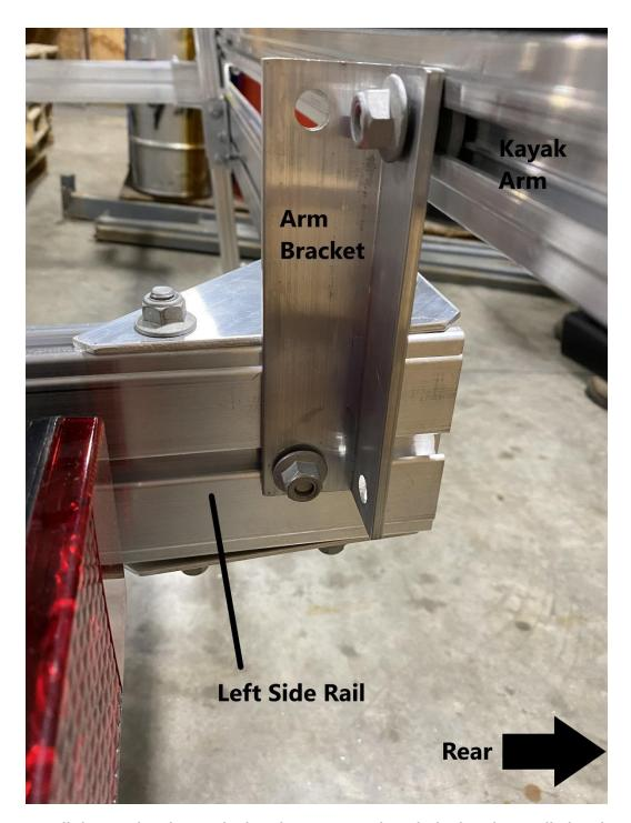
Install the arm bracket to the kayak arm, using the T-bolt already installed in the arm bracket. After the arm bracket has been installed to the kayak arm, install the arm bracket to the left side rail, using the T-bolt already installed in the arm bracket. Tighten both locknuts using a 9/16" wrench. Repeat this process for the other side.
