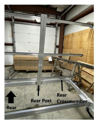
With the (2) arm brackets installed, the (2) locknuts holding the rear post will need to be tightened. Tighten the (2) locknuts using a 9/16" wrench.
