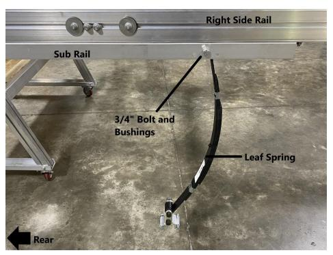
Install the leaf spring to the sub rail as shown. With the (2) bushings in the leaf spring, replace the ¾" bolt through the sub rail, bushings, and leaf spring. Replace the nut but do not tighten yet.
