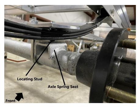
Place the locating stud of the leaf spring into the axle spring seat.
