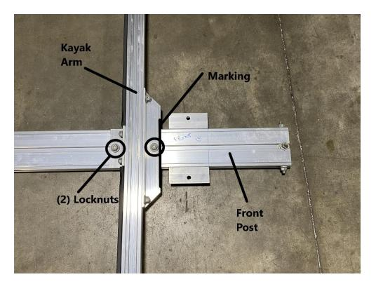
The front post will have (3) markings to show where each kayak arm should be installed. Lineup the kayak arm with the markings as shown. When the kayak arm is in position, tighten the (2) locknuts using a 9/16" wrench. Use a square to ensure that the kayak arm is straight. Repeat this process for all three kayak arms.
