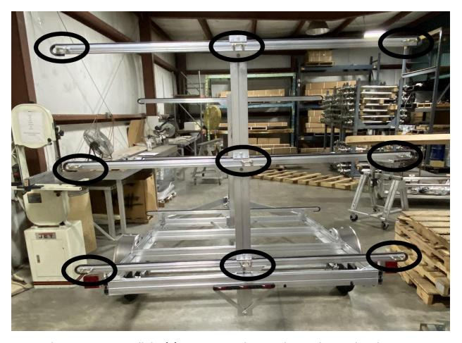
Repeat the process to install the (9) remaining web strap clips to the rear kayak arms.
