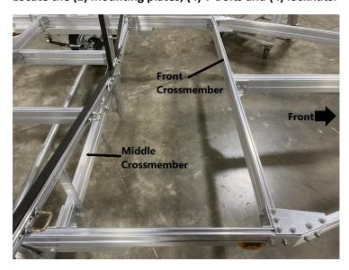
Locate the area between the middle crossmember and the front crossmember. This is the location the storage box will be installed.
