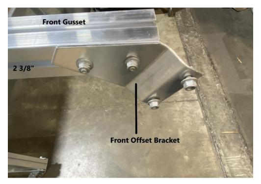
Install (1) front offset bracket to the 2 3/8" side of the front gusset as shown. Tighten the nuts using a 9/16" wrench.
