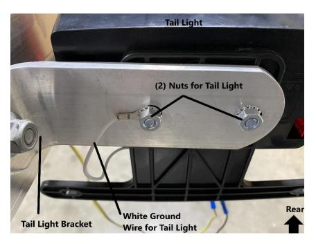
Install the white ground wire of the tail light to the carriage bolt as shown. Install nuts and tighten using 9/16" wrench. Repeat this process on the other side of the trailer to install both tail lights.
