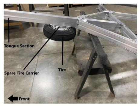
Mount the tire to the spare tire carrier as shown. Replace and tighten the lug nuts.
