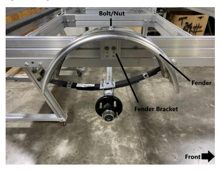
Install the fender to the fender bracket as shown. Replace the bolt and nut that was previously installed on the fender bracket. Tighten using a 9/16" wrench. Do no overtighten as this will damage the fender.
