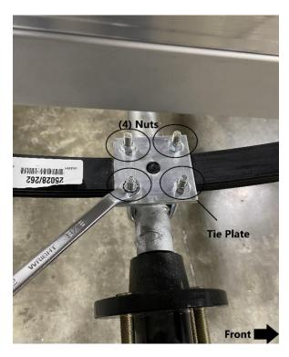
Use a cross pattern to tighten the (4) nuts using a 9/16" wrench. Repeat this process for this other side.
