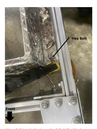
Place (4) hex bolts into the (4) drilled holes.
