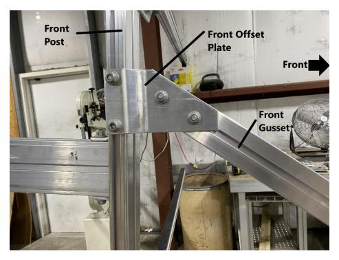
Install the second front offset bracket to front gusset and front post as shown. Replace the (4) locknuts and tighten using a 9/16" wrench.
