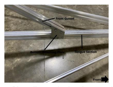
Install the second bottom attaching plate as shown. Remove the (3) locknuts from the (3) T-Bolts in the tongue section. Insert (2) T-Bolts into the front gusset and install the bottom attaching plate. Replace the locknuts and tighten using a 9/16" wrench.
