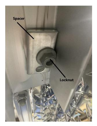
Install the (4) spacers and (4) locknuts to the (4) hex bolts. Tighten the locknuts using a 9/16" wrench.
