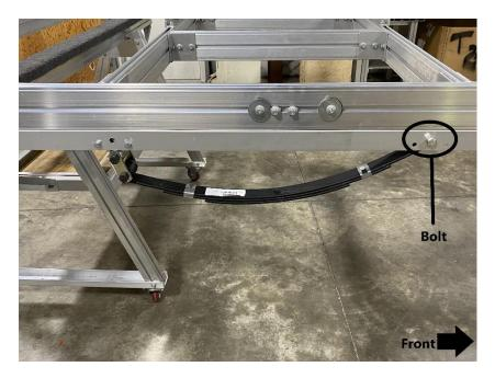
Tighten the bolt using a ¾" ratchet and wrench. Repeat this process for the other side.
