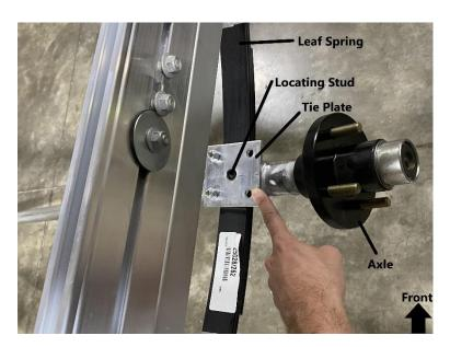
Install the axle to the leaf spring as shown. Slide the tie plate over the leaf spring until the center hole of the tie plate lines up with the locating stud of the leaf spring.
