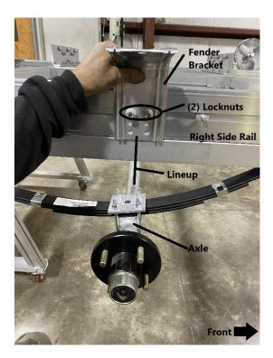
Locate the (4) T-bolts installed earlier in the right side rail. Install the fender bracket to the right side rail as shown. Use the (2) center T-bolts to install the fender bracket to the right side rail. Lineup the center of the fender bracket to the axle. Replace the locknuts and tighten using a 9/16" wrench.
