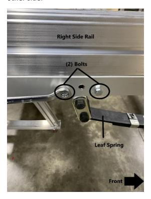
With the axle now installed the bolts of the leaf spring will now need to be tightened. Tighten the (2) bolts shown using a 9/16" ratchet and wrench. Repeat this process for the other side.
