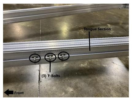
Locate the (3) T-bolts and locknuts installed in the tongue section. Remove the locknuts using a 9/16" wrench.
