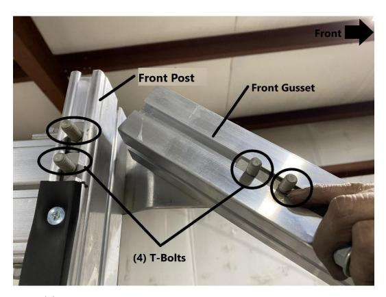
Install (4) T-Bolts to the front gusset and front post as shown.
