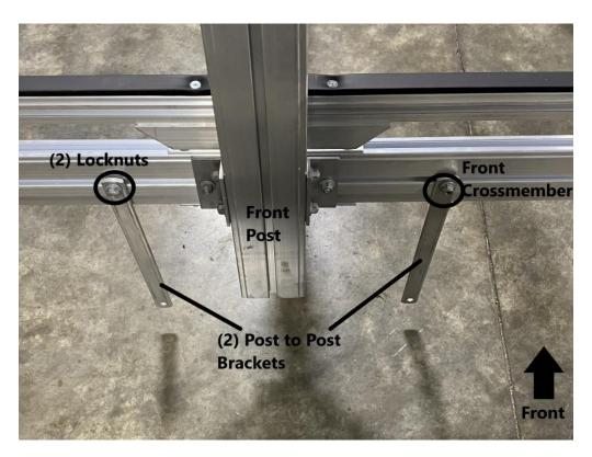
Install (2) post to post brackets using the remaining (2) T-bolts installed in the front crossmember. Replace the (2) locknuts but do not fully tighten yet.
