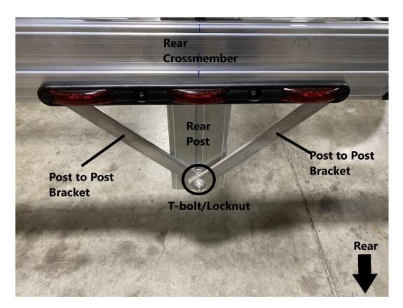
Move to the outside of the trailer. Place a T-bolt into the groove of the rear post. This will be a longer T-bolt (1 1/8") that was originally installed in the rear post. Install the (2) post to brackets to the T-bolt as shown. Install a locknut on the T-bolt and tighten using a 9/16" wrench.
