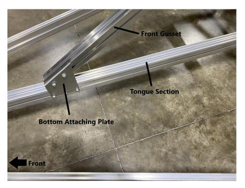
Install the bottom attaching plate and front gusset to the tongue section as shown. Replace the locknuts and tighten using a 9/16" wrench.
