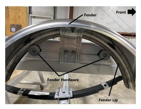
Install the fender hardware as shown, placing a rubber and metal washer behind the fender lip, then a metal washer and locknut in front of the fender lip. Tighten the locknut using a 9/16" wrench. Repeat this process to install both fenders.
