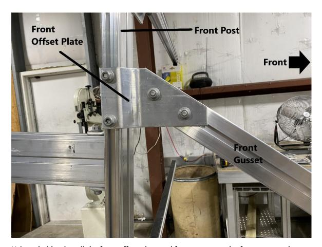
Using a ladder, install the front offset plate and front gusset to the front post as shown. Tighten the locknuts using a 9/16" wrench.
