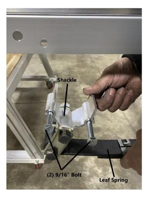
Remove the (2) 9/16" bolts from the shackle installed on the leaf spring.
