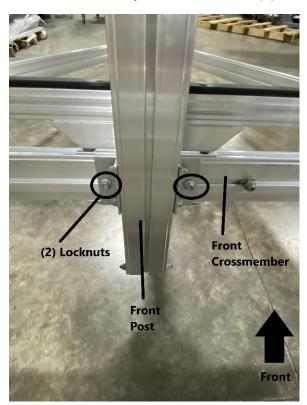
Two people will be necessary to install the front post. Install the front post to the (2) center T-bolts as shown. Replace the locknuts but do not fully tighten yet.
