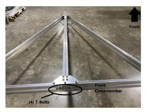
Locate the (4) T-bolts installed in the front crossmember. The (2) center T-bolts will be used to install the front post. Remove the (2) locknuts using a 9/16" wrench.
