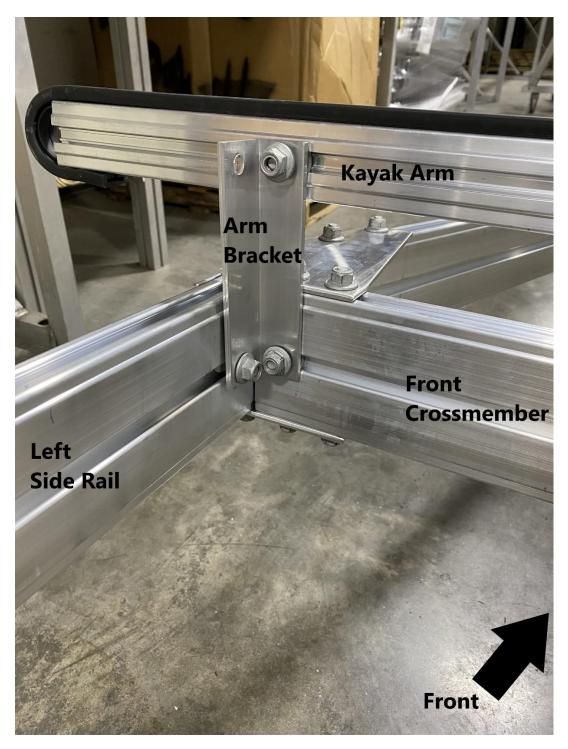
The left side rail and front crossmember will each have a T-bolt and locknut installed. Remove the locknuts using a 9/16" wrench. Install the arm bracket to the kayak arm, using the T-bolt already installed in the arm bracket. After the arm bracket has been installed to the kayak arm, install the arm bracket to the T-bolts installed in the left side rail and front crossmember. Tighten all (3) locknuts using a 9/16" wrench. Repeat this process for the other side.
