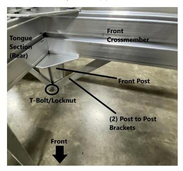
Move to the outside of the trailer. Place a T-bolt into the groove of the front post. This will be a longer T-bolt (1 1/8") that was originally installed in the front post. Install the (2) post to brackets to the T-bolt as shown. Install a locknut on the T-bolt and tighten using a 9/16" wrench. Tighten the (2) earlier locknuts using a 9/16" wrench.
