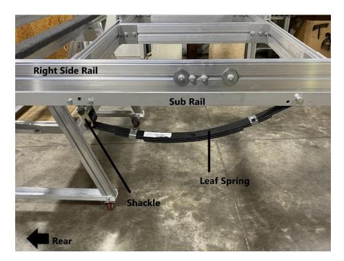
Install the shackle of the leaf spring into the sub rail as shown. Replace the 9/16" bolts. Replace the nuts but do not tighten yet. Repeat this process to install a second leaf spring on the left side rail.
