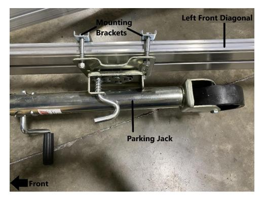
Install the parking jack to the left (driver's side) front diagonal of the trailer as shown. Place the (2) bolts on top of the left front diagonal, with the parking jack facing outside of the trailer.
