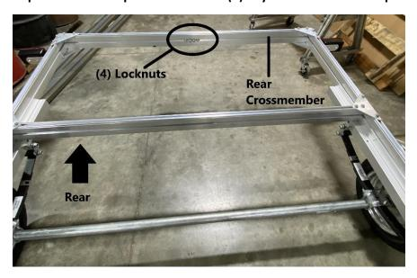
Locate the (4) locknuts installed on the rear crossmember. The two center locknuts will be used to install the rear post. Remove the (2) center locknuts using a 9/16" wrench.
