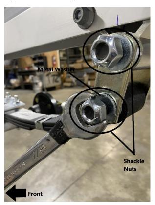
Tighten the rear shackle nuts with 7/8" ratchet and wrench. Ensure that the metal washers are not moving. However, do not over tighten as this will not allow the suspension to move properly. Repeat this process for the other side.
