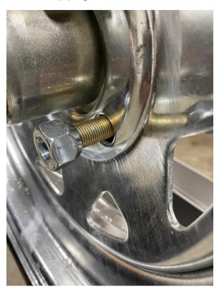
Install the lug nuts with the tapered side facing the wheel.
