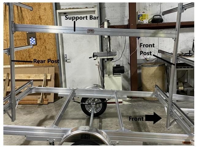
Install the support bar to the trailer as shown. Two people will be necessary to install the support bar. A ladder will also be required. Follow all safety requirements while using the ladder. Slide the (4) T-Bolts installed on the (4) angles into the grooves of the front and rear posts. Tighten the (4) locknuts using a 9/16" wrench.
