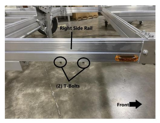
Install (2) T-Bolts to the right side rail as shown.
