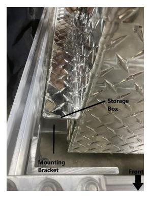
Confirm that the edge of the mounting bracket is flush with the end of the storage box. Tighten the (2) locknuts on each mounting brackets using a 9/16" wrench.
