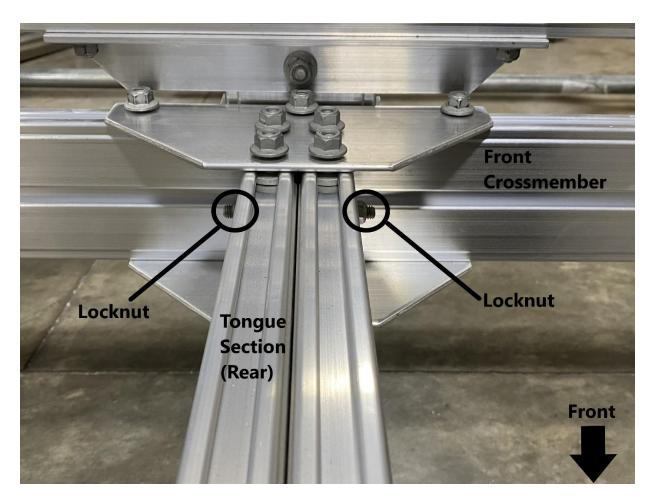
Locate the (2) locknuts installed in the rear tongue section. Remove the (2) locknuts using a 9/16" wrench. Install the remaining (2) post to post brackets to the (2) T-bolts. Replace the locknuts but do not fully tighten yet.
