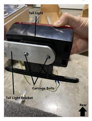
Install the tail light to the tail light bracket as shown.
