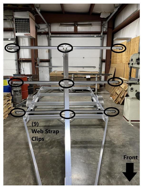
Install (9) web strap clips into the (3) front kayak arms as shown. Slide the tab weld nuts of the web strap clip into the groove of the kayak arms. The rubber vinyl may need pushed to allow access the groove of the kayak arms.
