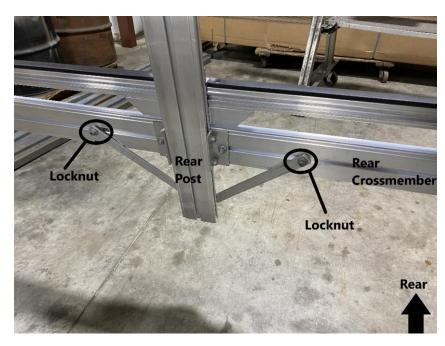
Tighten the (2) earlier locknuts using a 9/16" wrench.
