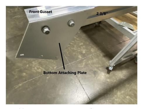
Install (1) bottom attaching plate to the 2 3/8" side of the front gusset as shown. This will be on the same groove that the front offset plate was installed. Tighten the locknuts using a 9/16" wrench.
