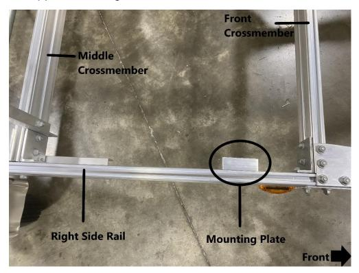
Install the mounting plate to the (2) T-bolts in the right side rail as shown. Loosely replace the (2) locknuts. Repeat this process on the left side rail.
