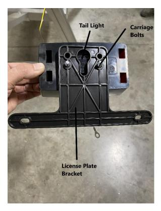
Install the license plate bracket to the tail light as shown. Place the two bottom holes of the license plate bracket on the two carriage bolts installed on the tail light.
