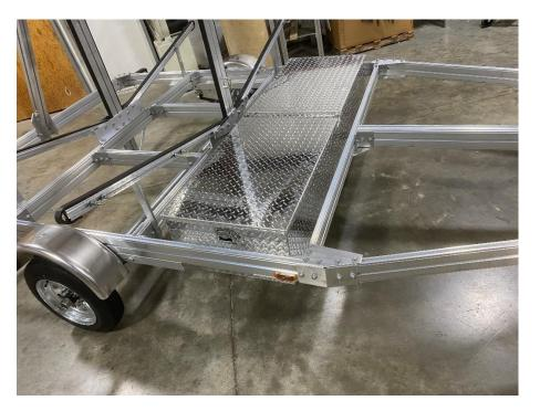
Place the aluminum storage box on the trailer as shown.
