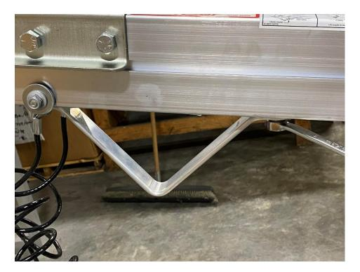
Re-install the skid bracket if necessary.
