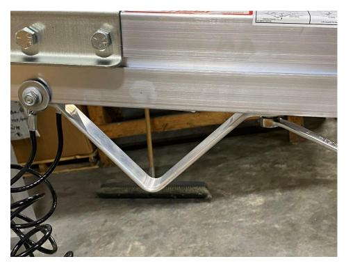
Re-install the skid bracket if necessary.
