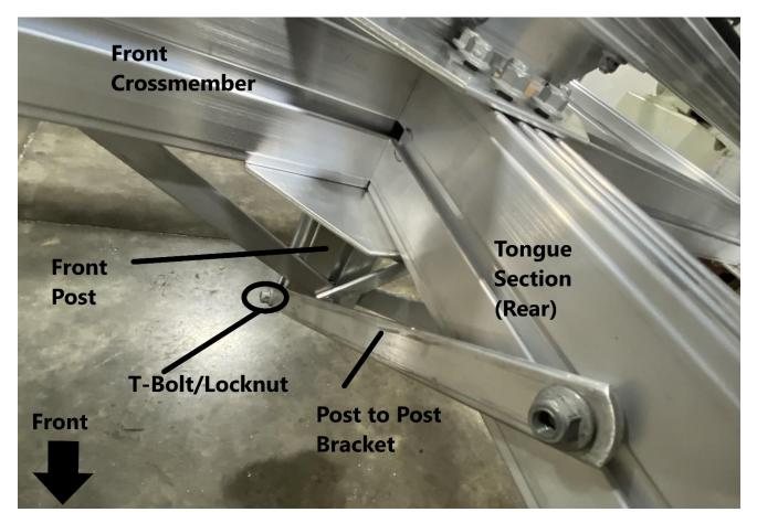
The front post will have (2) T-bolts and locknuts installed in the side grooves. Remove the (2) locknuts using a 9/16" wrench. Install the (2) post to post brackets to the front post as shown, using the T-bolts installed in the side grooves of the front post. Replace the (2) locknuts and tighten using a 9/16" wrench. Once complete, tighten the (2) locknuts holding the (2) post to post to post brackets to the rear tongue section using a 9/16" wrench.
