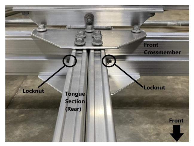
Locate the (2) locknuts installed in the rear tongue section. Remove the (2) locknuts using a 9/16" wrench. Install the remaining (2) post to post brackets to the (2) T-bolts. Replace the locknuts but do not fully tighten yet.
