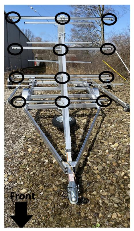
Install (12) web strap clips into the (4) front kayak arms as shown. Slide the tab weld nuts of the web strap clip into the groove of the kayak arms. The rubber vinyl may need pushed to allow access to the groove of the kayak arms.
