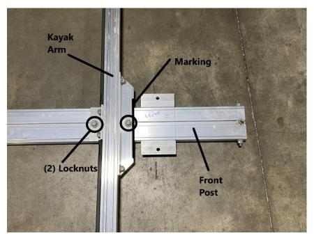
The front post will have (4) markings to show where each kayak arm should be installed. Lineup the kayak arm with the markings as shown. When the kayak arm is in position, tighten the (2) locknuts using a 9/16" wrench. Use a square to ensure that the kayak arm is straight. Repeat this process for all three kayak arms.
