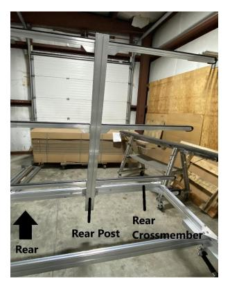
With the (2) arm brackets installed, the (2) locknuts holding the rear post will need to be tightened. Tighten the (2) locknuts using a 9/16" wrench.
