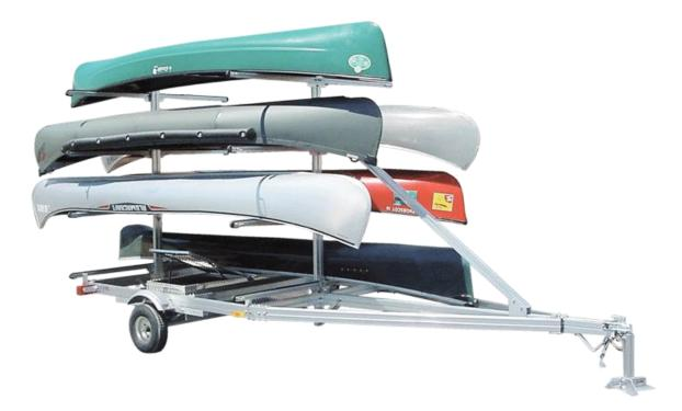
The trailer is now assembled. Connect the flat four prong harness to the tow vehicle and confirm that all lights are in working order. Connect the safety cables to the tow vehicle in a crossing pattern. Connect the coupler to the hitch ball and confirm that the size of the coupler matches the hitch ball. Use a lock to confirm the coupler is locked in place. Torque the lug nuts after 20 miles to 80 foot pounds.
