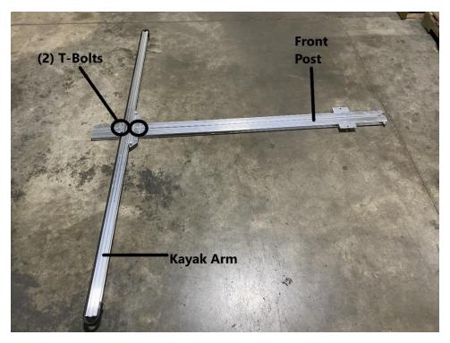
Slide the (2) T-bolts installed on the kayak arm into the groove of the front post as shown. Continue sliding kayak arms into the groove of the front post until a total of (4) kayak arms have been installed.
