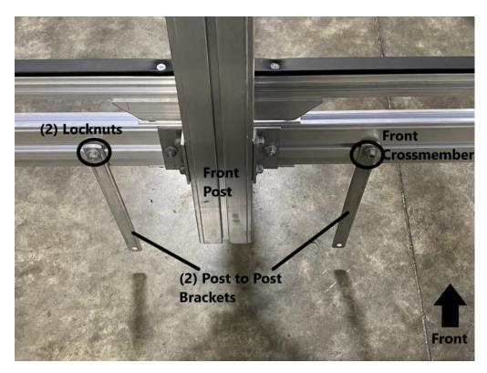
Install (2) post to post brackets using the remaning (2) T-bolts installed in the front crossmember. Replace the (2) locknuts but do not fully tighten yet.
