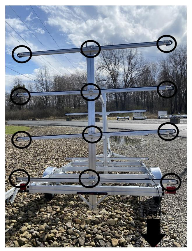
Repeat the process to install the (12) remaining web strap clips to the rear kayak arms.
