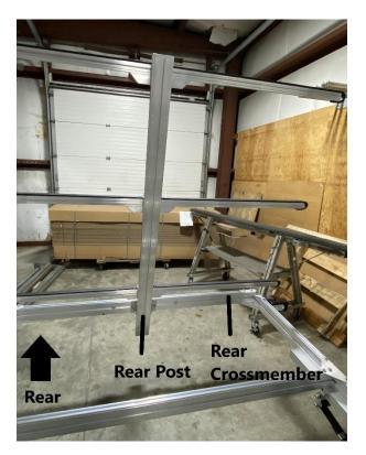
Two people will be necessary to install the rear post. Install the rear post to the (2) center Tbolts as shown. Replace the locknuts but do not fully tighten yet.
