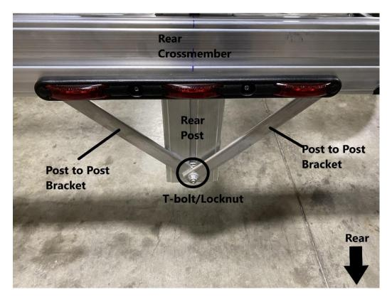
Move to the outside of the trailer. Place a T-bolt into the groove of the rear post. This will be a longer T-bolt (1 1/8") that was originally installed in the rear post. Install the (2) post to brackets to the T-bolt as shown. Install a locknut on the T-bolt and tighten using a 9/16" wrench.
