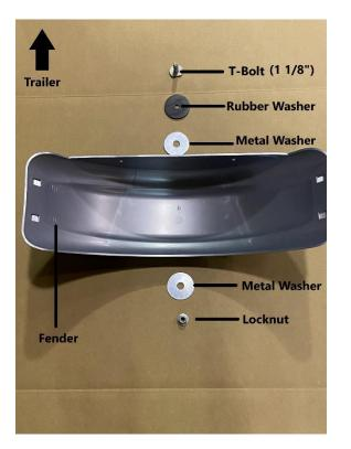
Note the ordering of the fender hardware in the above picture.
