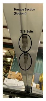
Place the (2) T-bolts that were removed from the spare tire carrier into the groove on the bottom of the tongue section.
