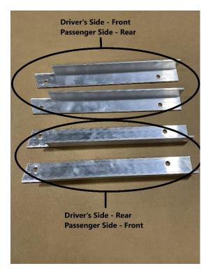
Remove the T-bolts and locknuts from the V-Bar support brackets. See the picture above, this shows where each V-Bar will be used on the trailer.
