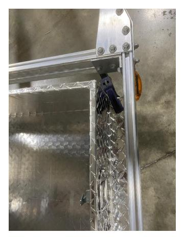
Use "C" Clamps to hold the storage box in place while drilling. Place a "C" Clamp on each side to prevent movement.
