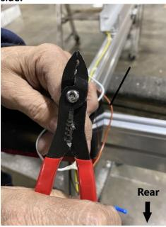
Use a pair of wire cutters to strip the ends of the (4) tail light wires (2 brown, 1 green, 1 yellow), (4) harness wires (2 brown, 1 green, 1 yellow) and (1) LED 3 Light Bar wire/connecting wire. Note that the white ground wire on the tail light will be installed later.
