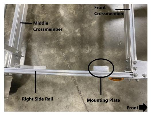
Install the mounting plate to the (2) T-bolts in the right side sail as shown. Loosely replace the (2) locknuts. Repeat this process on the left side rail.
