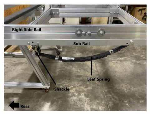
Install the shackle of the leaf spring into the sub rail as shown. Replace the 9/16" bolts. Replace the nuts but do not tighten yet. Repeat this process to install a second leaf spring on the left side rail.
