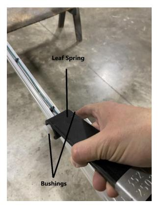
Insert the (2) nylon bushings into the leaf spring.
