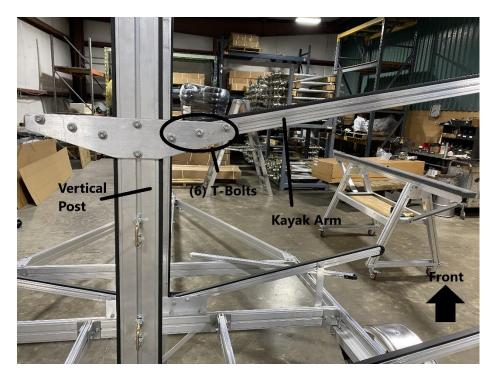
Repeat the process to install a kayak arm to the vertical post as shown. Tighten the (6) T-bolts using a 9/16" wrench.
