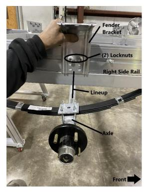
Install the fender bracket to the right side rail as shown. Use the (2) center T-bolts to install the fender bracket to the right side rail. Lineup the center of the fender bracket to the axle. Replace the locknuts and tighten using a 9/16" wrench.
