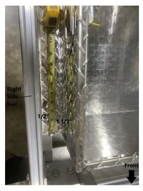
Four holes will now need to be drilled to secure the storage box. Use measuring tape to measure 1 ½" from the edge of the storage box and ½" from the right side rail as shown. Mark the measurements. Repeat this process so there are two marks on the left (driver's side) and two marks on the right (passenger side).
