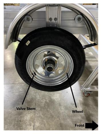
Install the wheel with the valve stems facing out.
