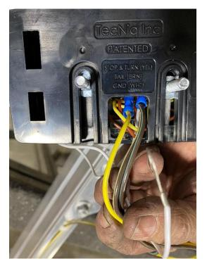
Excess wire can be placed inside the tail light.
