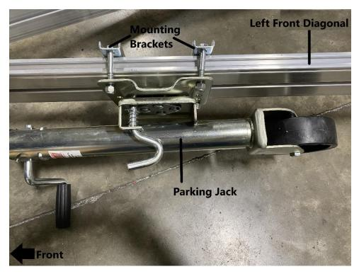
Install the parking jack to the left (driver's side) front diagonal of the trailer as shown. Place the (2) bolts on top of the left front diagonal, with the parking jack facing outside of the trailer.
