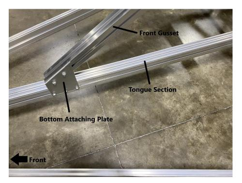
Install the bottom attaching plate and front gusset to the tongue section as shown. Replace the locknuts and tighten using a 9/16" wrench.
