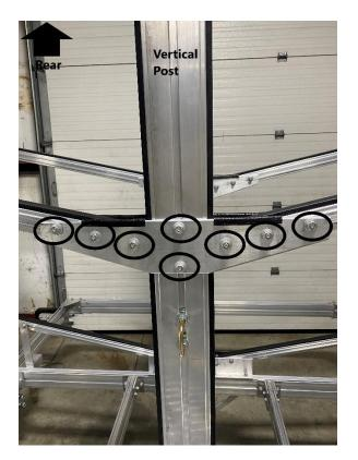
Tighten all the locknuts on the (2) vertical posts using a 9/16" wrench.
