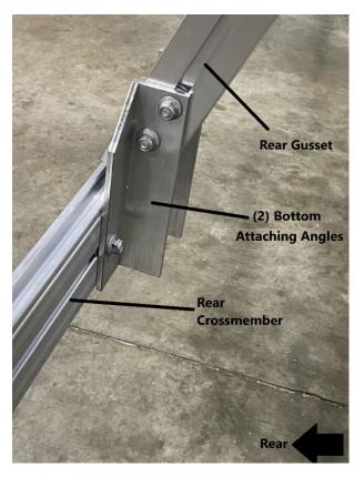
Install the (2) bottom attaching angles to the rear crossmember as shown. Remove the locknuts from the rear crossmember and install the (2) bottom attaching angles. Tighten the locknuts using a 9/16" wrench.
