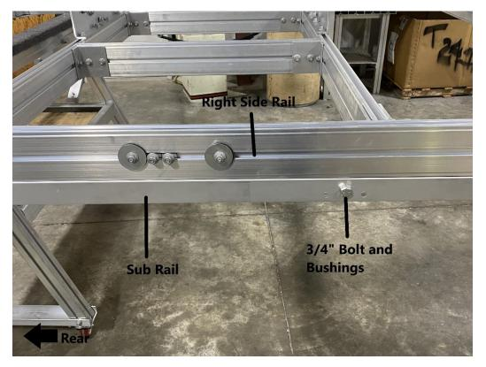
Locate the sub rail installed on the bottom of the right side rail. Remove the  $\frac{34}{7}$  bolt and bushings.
