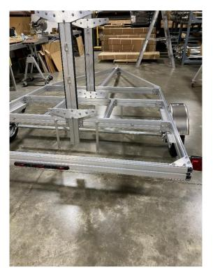
Repeat the process to install the second vertical post to the trailer.
