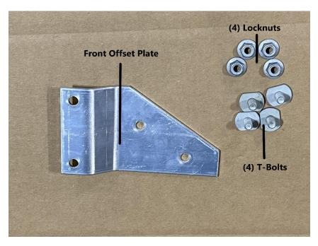
Remove the (4) locknuts and (4) T-Bolts from the remaining front offset plate.
