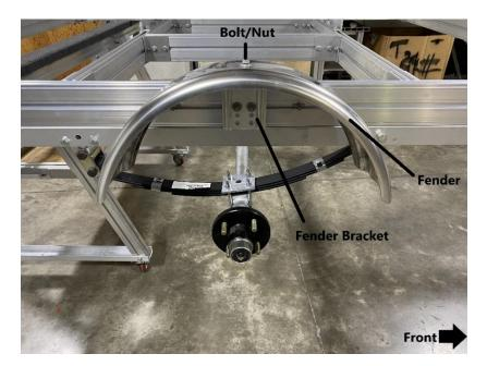
Install the fender to the fender bracket as shown. Replace the bolt and nut that was previously installed on the fender bracket. Tighten using a 9/16" wrench. Do no overtighten as this will damage the fender.
