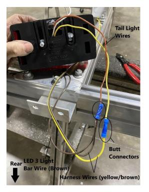
Use butt connectors to connect the tail light and the LED 3 light bar to the wiring harness as shown. Match the brown wire of the harness with the brown wire of the tail light. Same for the yellow wires. Note that both the brown LED 3 light bar wire/connecting wire and the brown harness wire will need to be connected together.
