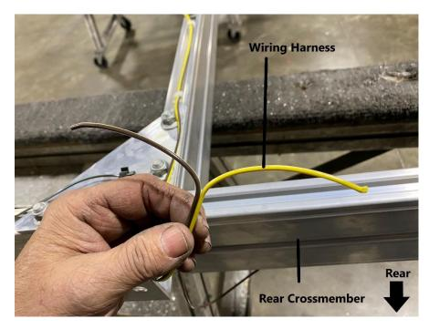
Locate the end of the wiring harness that is hanging underneath the right side rail. Use a utility knife to split the two wires of the wiring harness. Repeat this process for the other side.
