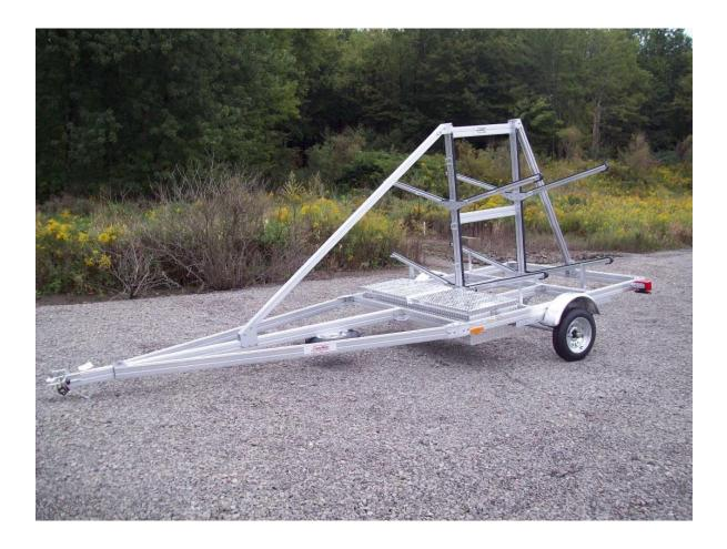
The trailer is now assembled. Connect the flat four prong harness to the tow vehicle and confirm that all lights are in working order. Connect the safety cables to the tow vehicle in a crossing pattern. Connect the coupler to the hitch ball and confirm that the size of the coupler matches the hitch ball. Use a lock to confirm the coupler is locked in place. Torque the lug nuts after 20 miles to 80 foot pounds.
