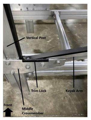
Install trim lock to the middle crossmember as shown. Push the trim lock down onto the top of the middle crossmember. This will prevent rubbing between the middle crossmember and the kayak arm.
