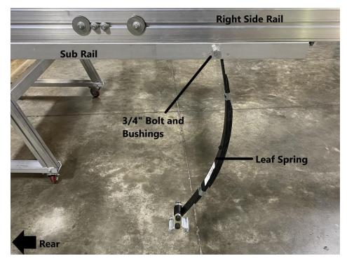
Install the leaf spring to the sub rail as shown. With the (2) bushings in the leaf spring, replace the  $\frac{3}{7}$  bolt through the sub rail, bushings, and leaf spring. Replace the nut but do not tighten yet.
