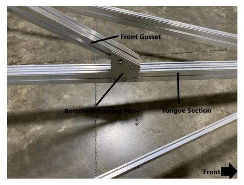
Install the second bottom attaching plate as shown. Remove the (3) locknuts from the (3) T-Bolts in the tongue section. Insert (2) T-Bolts into the front gusset and install the bottom attaching plate. Replace the locknuts and tighten using a 9/16" wrench.
