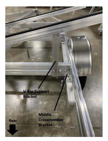
Install the V-Bar Support bracket as shown. Install the V-Bar support bracket to the T-bolt on the middle crossmember and the T-Bolt on the passenger rear kayak arm. Move the V-Bar Support so that it sits next to the middle crossmember bracket. Replace the locknuts and tighten with a 9/16" wrench.
