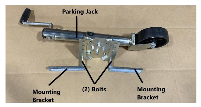
Install the (2) mounting brackets to the parking jack using (2) bolts and (2) locknuts as shown.
