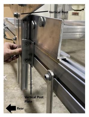
Install the vertical post plate as shown. Install (3) locknuts and tighten using a 9/16" wrench. Repeat this process for the other side of the vertical post.
