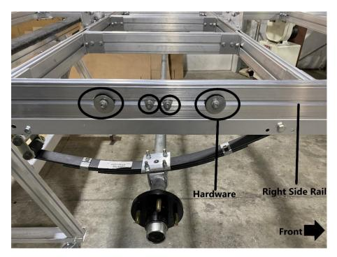
Remove all the hardware from the right side rail using a 9/16" wrench. This will leave 4 T-Bolts in the right side rail.
