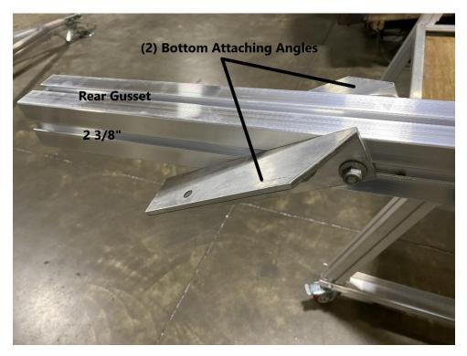
Install the (2) bottom attaching angles to the 2 3/8" side of the rear gusset. Tighten the nuts using a 9/16" wrench.
