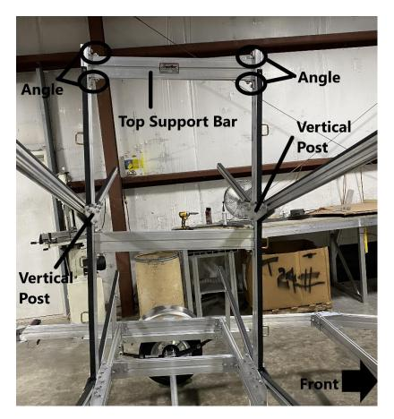
Install the top support bar to the trailer as shown. A ladder will be required for installation of the top support bar. Follow all safety requirements while using the ladder. Slide the (4) T-Bolts installed on the (4) angles into the grooves of the (2) vertical posts. Tighten the (4) locknuts using a 9/16" wrench.
