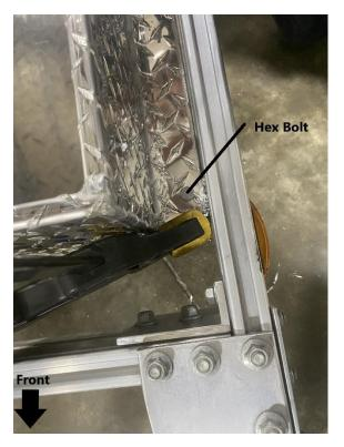
Place (4) hex bolts into the (4) drilled holes.
