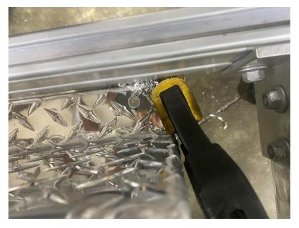
Use a 3/8" drill bit to drill four holes as shown.
