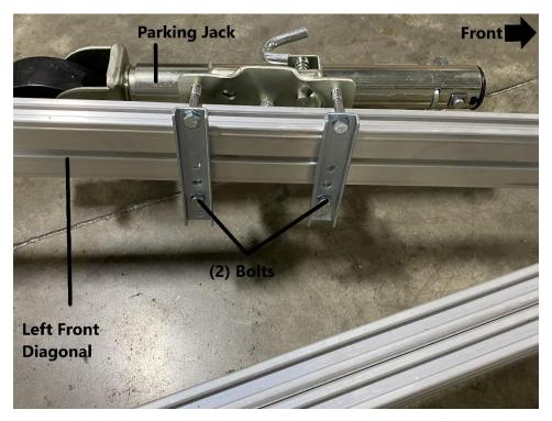
Install the remaining (2) bolts and (2) locknuts to the parking jack. Tighten all locknuts using a 9/16" ratchet and wrench.
