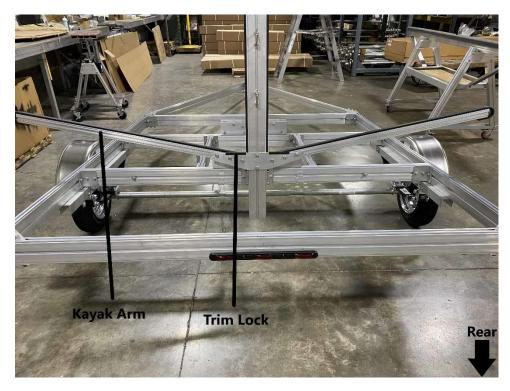
Repeat the process to install a second kayak arm and trim lock to the trailer.
