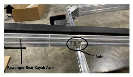
Install a T-Bolt in the groove of the passenger rear kayak arm. This will be the groove that is facing the front of the trailer.
