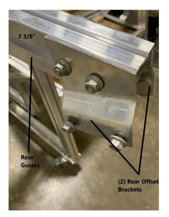
Install the (2) rear offset brackets to the 2 3/8" side of the rear gusset. Tighten the locknuts using a 9/16" wrench.
