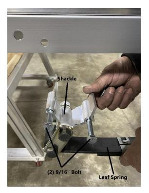
Remove the (2) 9/16" bolts from the shackle installed on the leaf spring.
