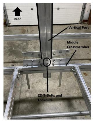
Two people will be necessary to install the vertical post onto the middle crossmember. Locate the (2) T-bolts and locknuts shown in the picture. While holding the vertical post, move the (2) T-Bolts through the groove of the vertical post. Tighten the locknuts using a 9/16" wrench.
