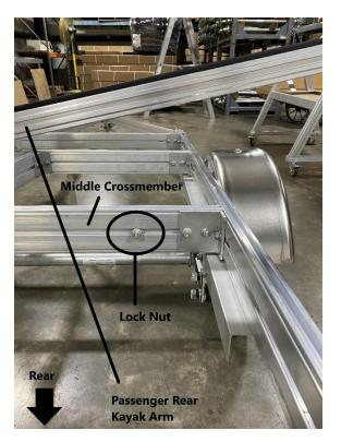
Remove the lock nut on the middle crossmember, underneath the passenger rear kayak arm.
