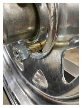
Install the lug nuts with the tapered side facing the wheel.
