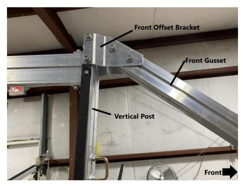
Install the front offset bracket to front gusset and vertical post as shown. Replace the (4) locknuts and tighten using a 9/16" wrench.
