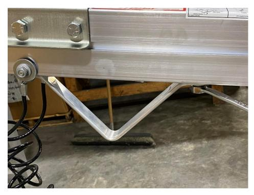
Re-install the skid bracket if necessary.
