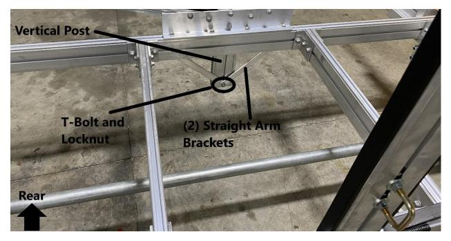
The hanging straight arm brackets will now need to be installed to the vertical post. Install a T-Bolt into the groove of the vertical post. Install both straight arm brackets on T-Bolt. Install a locknut and tighten using a 9/16" wrench. Repeat this process for the second vertical post.
