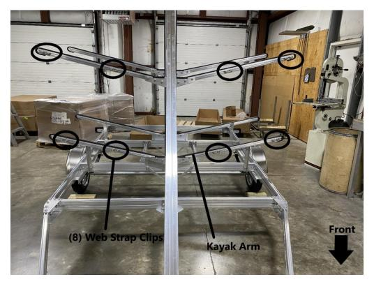
Install (8) web strap clips into the (4) front kayak arms as shown. Slide the tab weld nuts of the web strap clip into the groove of the kayak arms.
