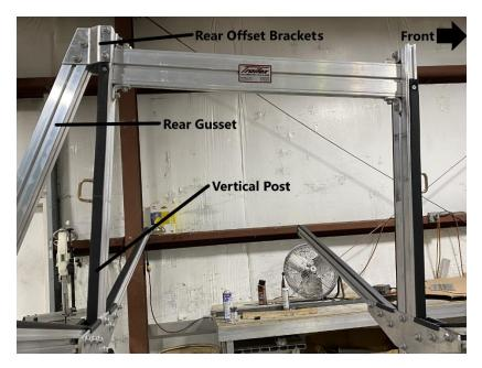
Using a ladder, install the (2) rear offset brackets to the vertical post as shown. Tighten the nuts using a 9/16" wrench.
