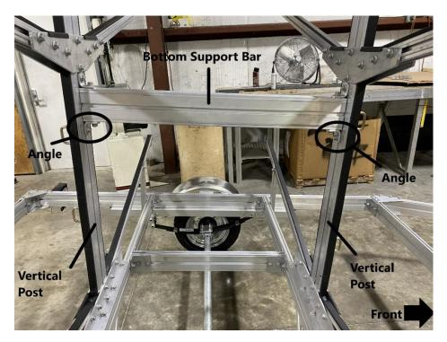
Repeat the process to install the bottom (2) angles of the (2) vertical posts to the bottom support bar.
