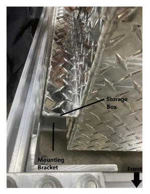
Confirm that the edge of the mounting bracket is flush with the end of the storage box. Tighten the (2) locknuts on each mounting brackets using a 9/16" wrench.
