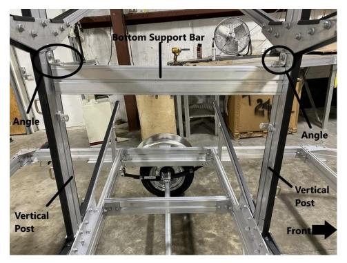
Install the bottom support bar as shown. Locate the (2) angles found on the (2) vertical posts. Place the (2) T-Bolts that were installed on the bottom support bar through the (2) angles of the vertical posts. Install (2) locknuts and tighten using a 9/16" wrench.
