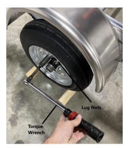
Torque the lug nuts to 80 foot pounds using a X pattern. Repeat the process for the other tire. Note that after 20 miles the lug nuts will need to be re-torqued to 80 foot pounds.
