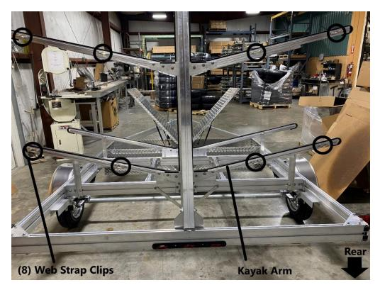
Repeat the process to install the (8) remaining web strap clips to the rear kayak arms.
