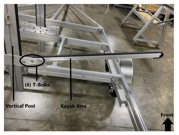
Install the kayak arm to the vertical post as shown. Slide the arm through the (6) T-Bolts, 3 on each side. Tighten the nuts using a 9/16" wrench.
