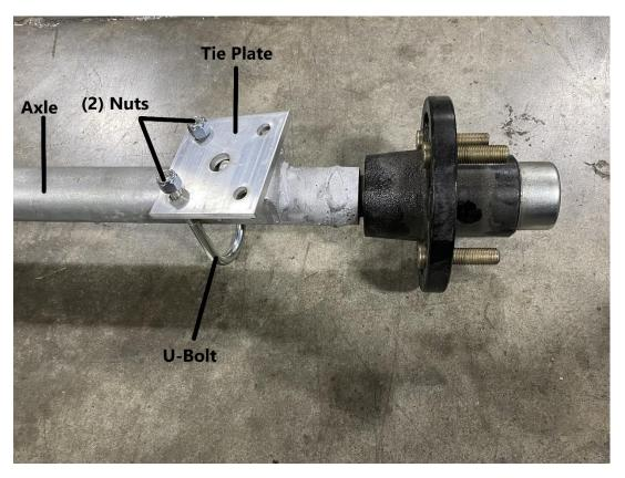
Install the Tie Plate and U-Bolt to the axle as shown. Replace the nuts but do not tighten yet.
