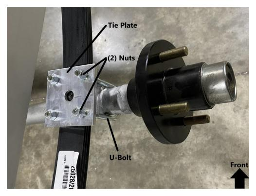
Install the second U-Bolt to the tie plate as shown. Replace the (2) nuts but do not tighten yet. Repeat this process to mount the axle to the leaf spring on the other side of the trailer.
