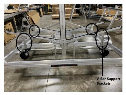
Repeat the process to install all (4) V-Bar Support Brackets.
