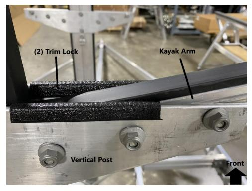
Use (2) pieces of trim lock on the kayak arms that are installed on the upper level of the vertical post.
