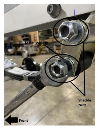
Tighten the rear shackle nuts with 7/8" ratchet and wrench. Ensure that the metal washers are not moving. However, do not over tighten as this will not allow the suspension to move properly. Repeat this process for the other side.
