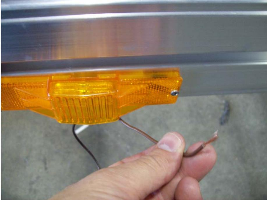
Locate the two drilled holes at the front of the side rail and install the light. Then strip away about a 1/4" of casing off the brown wire from the light.
