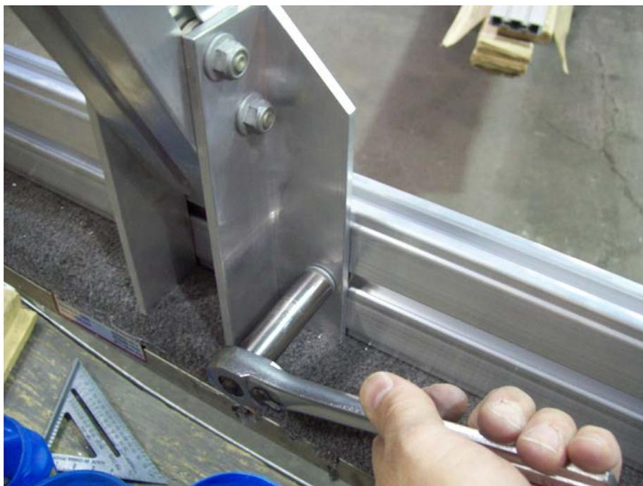
Now go back and tighten nuts on both top and bottom plates.
