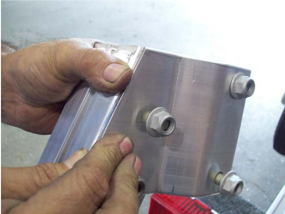
Install both top offset attaching plates to rear gusset and position as shown.
