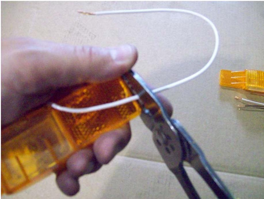
Cut approximately 8 1/2" off of the white wires on both running lights.
