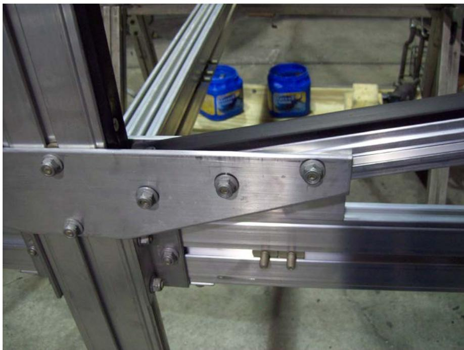
Insert the arm into the T-bolts on the brackets. T-bolts will need positioned to accommodate the arm as it is sliding in toward the post.
