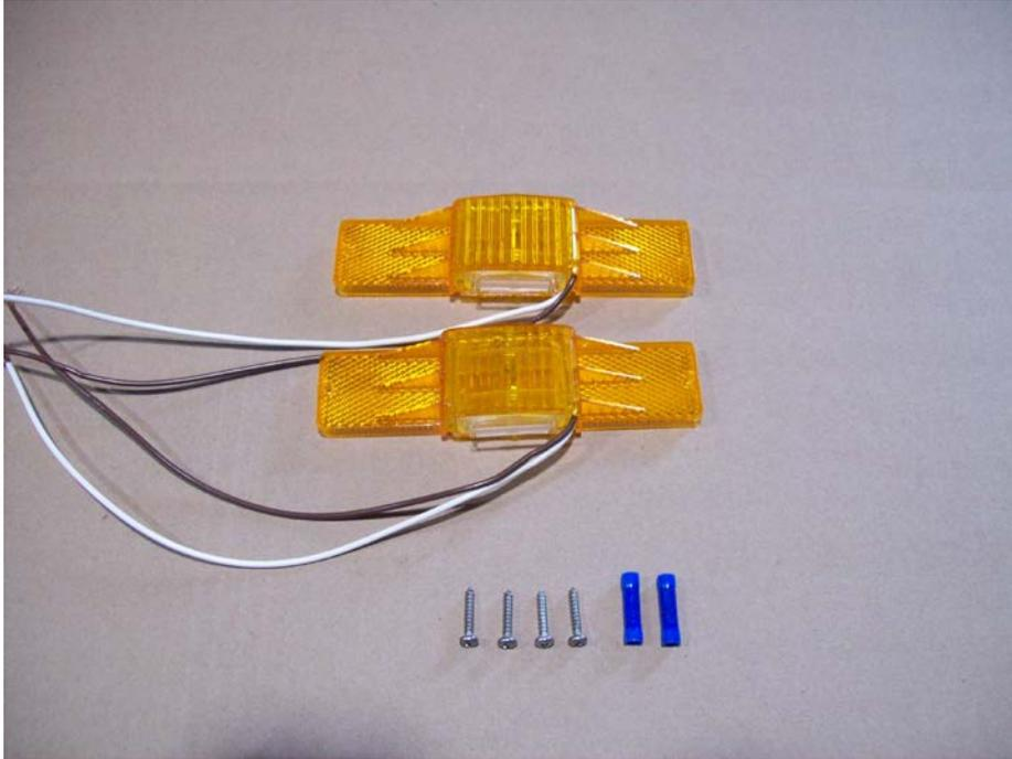
Locate two amber running lights, four small Philips screws, and two butt connectors.
