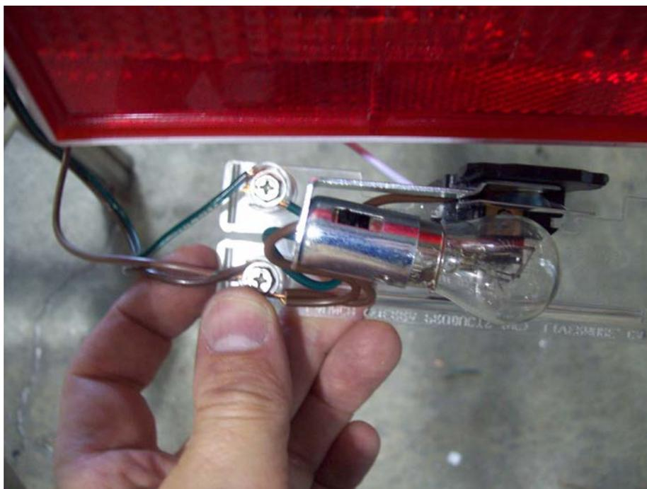
Remove the tail light assembly from the housing. Loosen the wire retaining screws and install the color matching wires from the wire harness onto the corresponding retaining screws. Reinstall into the housing. Repeat process for the other side.
