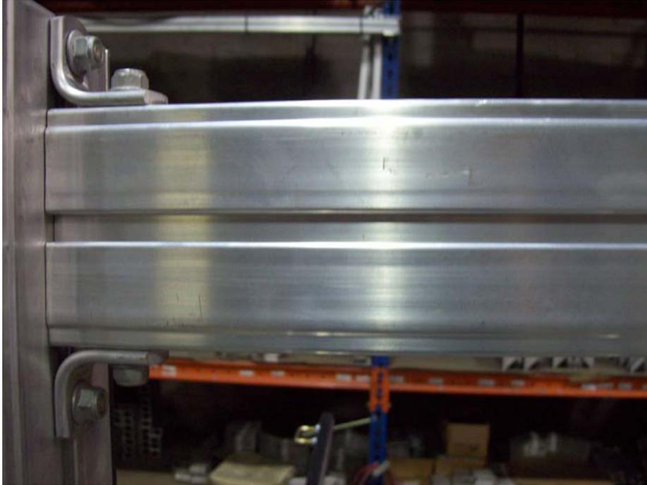
Position the top of both angle brackets on the horizontal bar even with the top of each vertical post.
