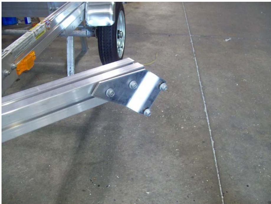
Install only the left side top plate. Position plate and tighten nuts.
