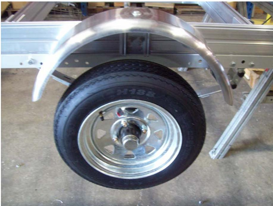
Install the wheels with the valve stems facing out. Install the lug nuts with the tapered side facing the wheel then tighten nuts.
