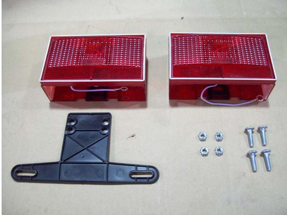
Locate the two tail lights, license plate bracket, 4 nuts, and 4 carriage bolts.
