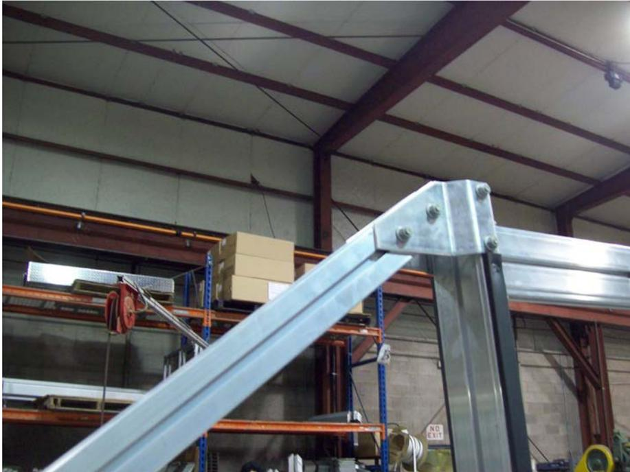
Insert T-bolts from the top offset attaching plates into the vertical post.
