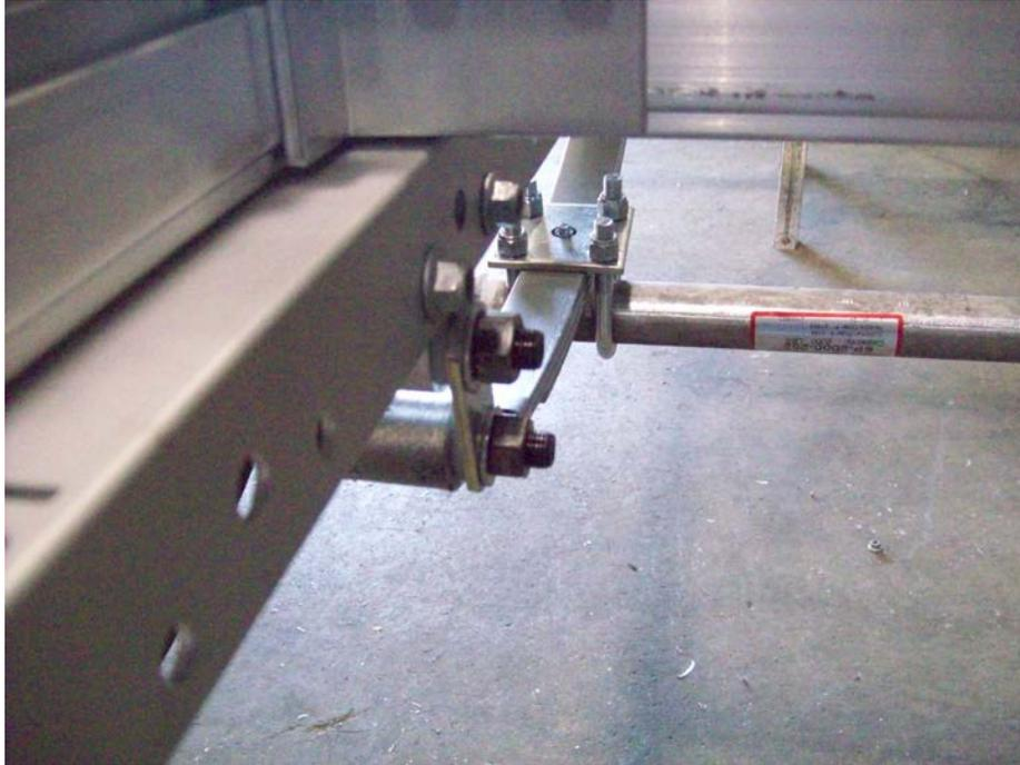
Do not over tighten the shackle nuts as this will not allow the suspension to move properly.
