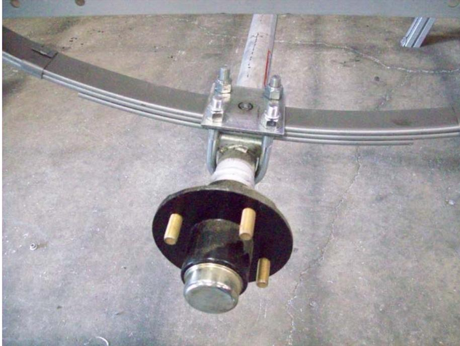
Position the axle and tighten the nuts evenly on the U-bolts.
