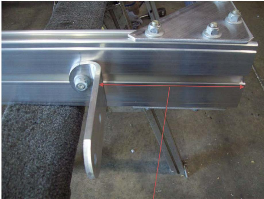
Install tail light brackets on T-bolts that are already on the side rail. Position tail lights 8 inches from the rear cross member as shown.
