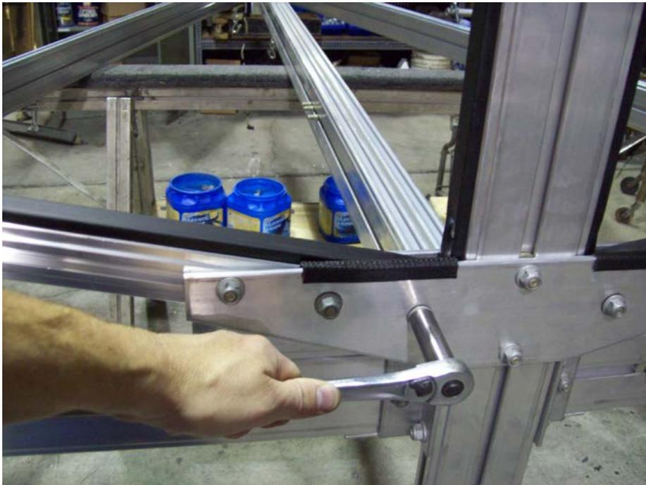
At this point tighten all nuts on arm assemblies.
