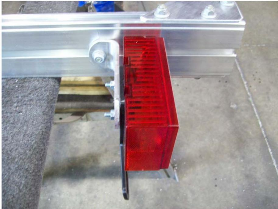
Install the left tail light with the license plate holder between the light and the bracket. Repeat the process for the other side then tighten the nuts on tail lights.
