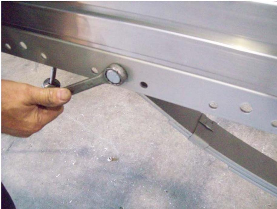
Once the axle is installed, go back and tighten the nuts on the leaf springs.
