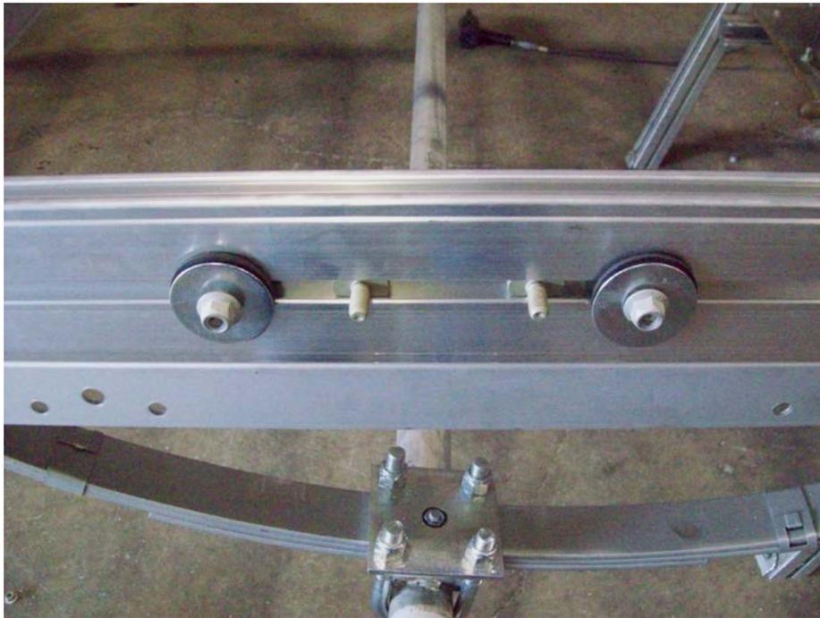
On the side rail of the trailer, locate the T-bolts and washers to mount the fenders.
