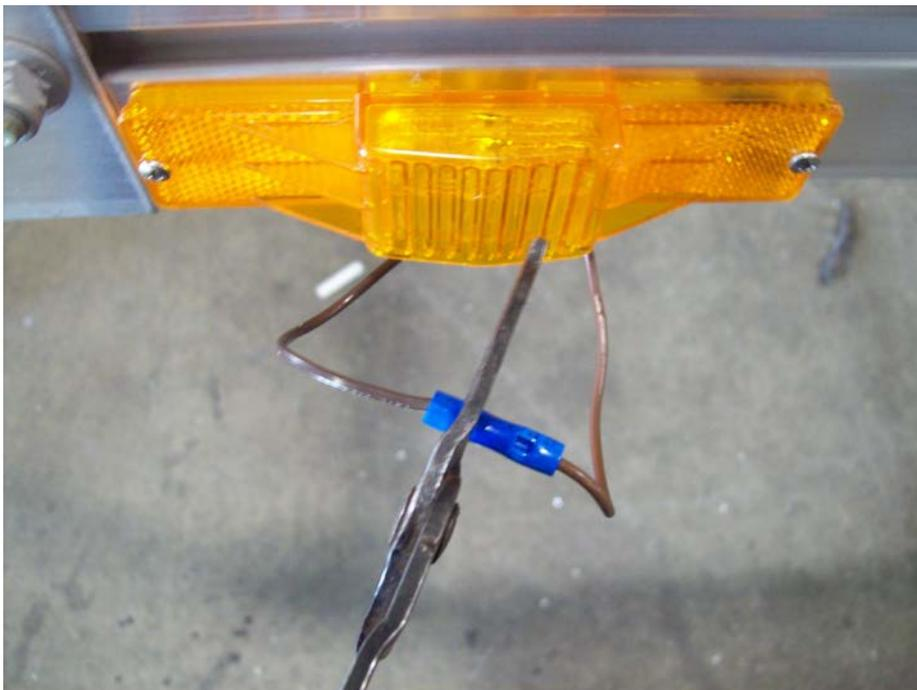
Pull down the brown wire of the main harness from the underside of the frame and strip 1/4" of casing off this wire. Crimp butt connector to both wires.
