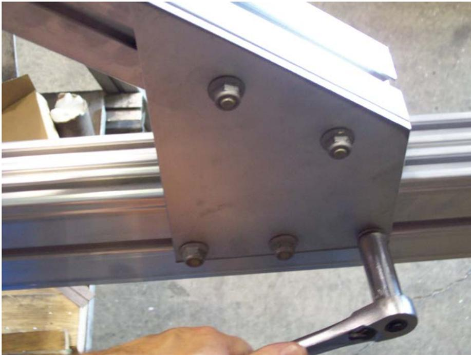
Install the right side bottom attaching plate into the three T-bolts on the tongue section. Now go back and tighten all the nuts on the top and bottom plates.
