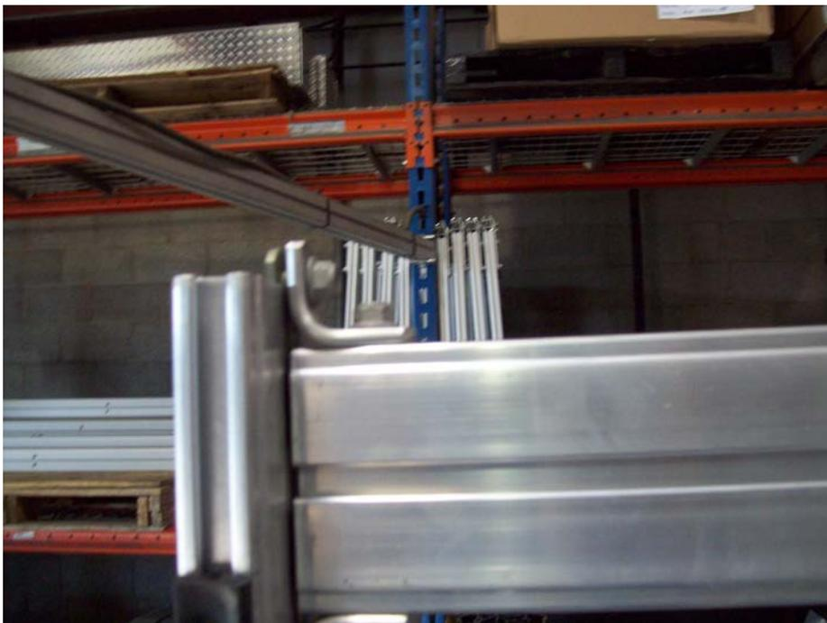
Install the upper horizontal bar into the top of each vertical post.
