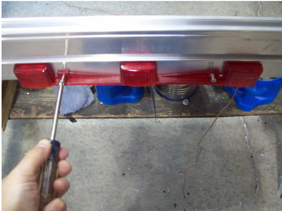
Install the three light bar on the rear cross member in the center where the holes are drilled.
