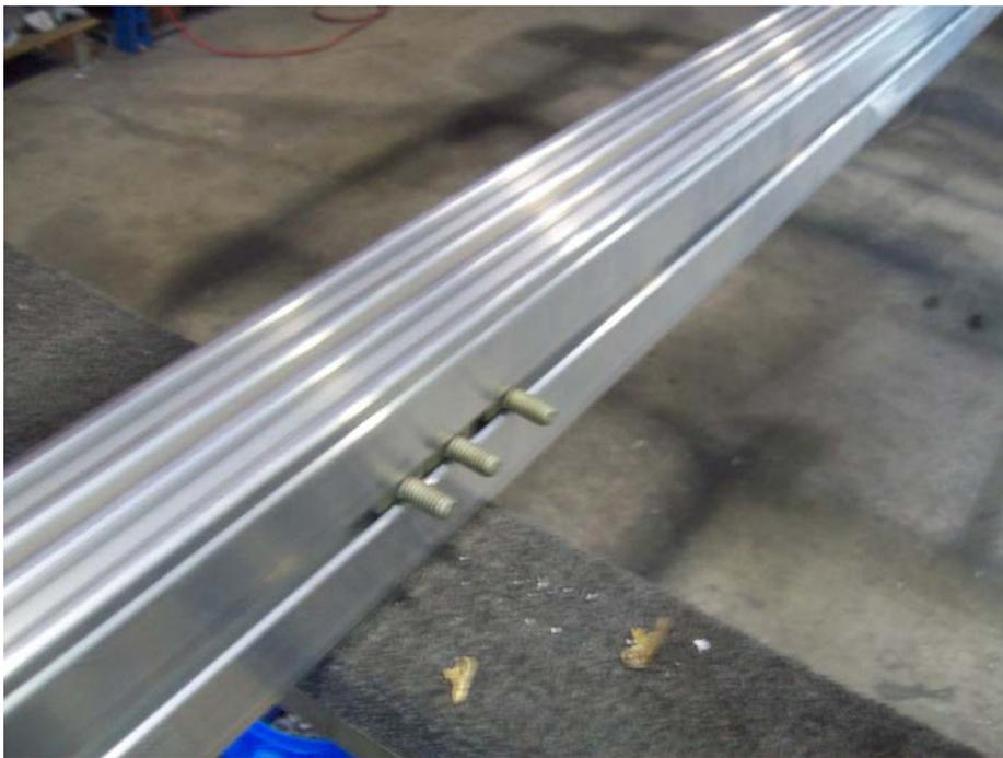
Locate the three T-bolts on the tongue section. Remove nuts and slide them towards the front.
