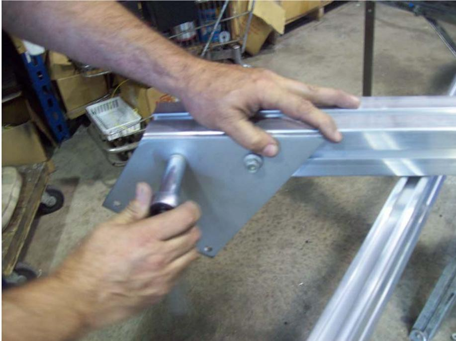
Install the left bottom plate to the gusset. Position plate and tighten nuts.
