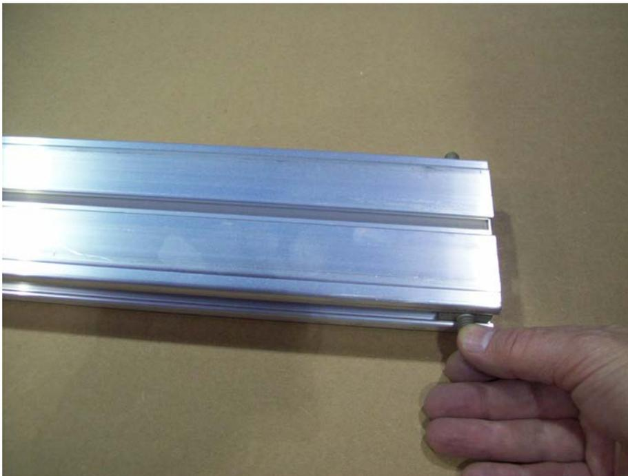
Remove the T-bolts from the angle brackets located halfway up on the back side of the vertical support. Install one T-bolt in each corner of the lower horizontal support.
