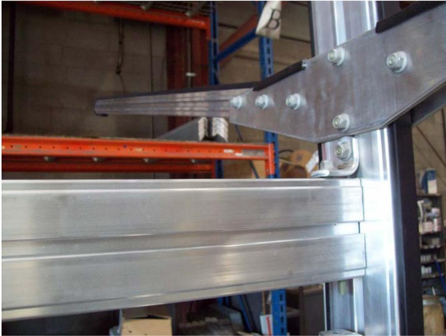
Loosen the lower angle brackets and slide out of the way. Insert top T-bolts into the upper angle brackets as shown and install nuts. Reattach lower angle brackets to underside of the bar. Install nuts and tighten.
