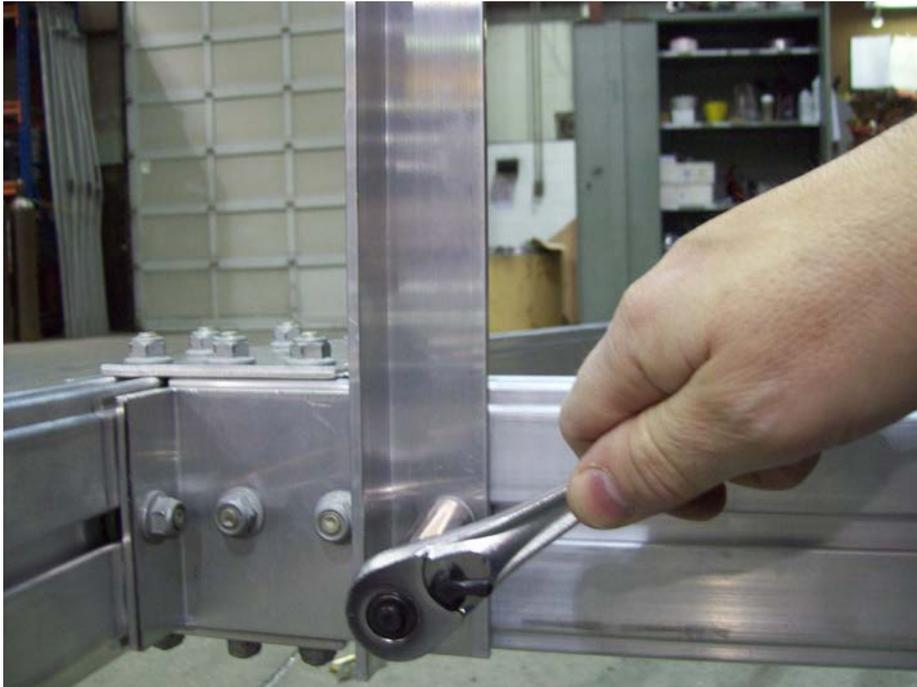
Slide the outer T-bolts in the cross member over to the corner angle bracket. Install support angle bracket over top of T-bolt. Support angle bracket should be flush with corner angle bracket. Tighten nut.
