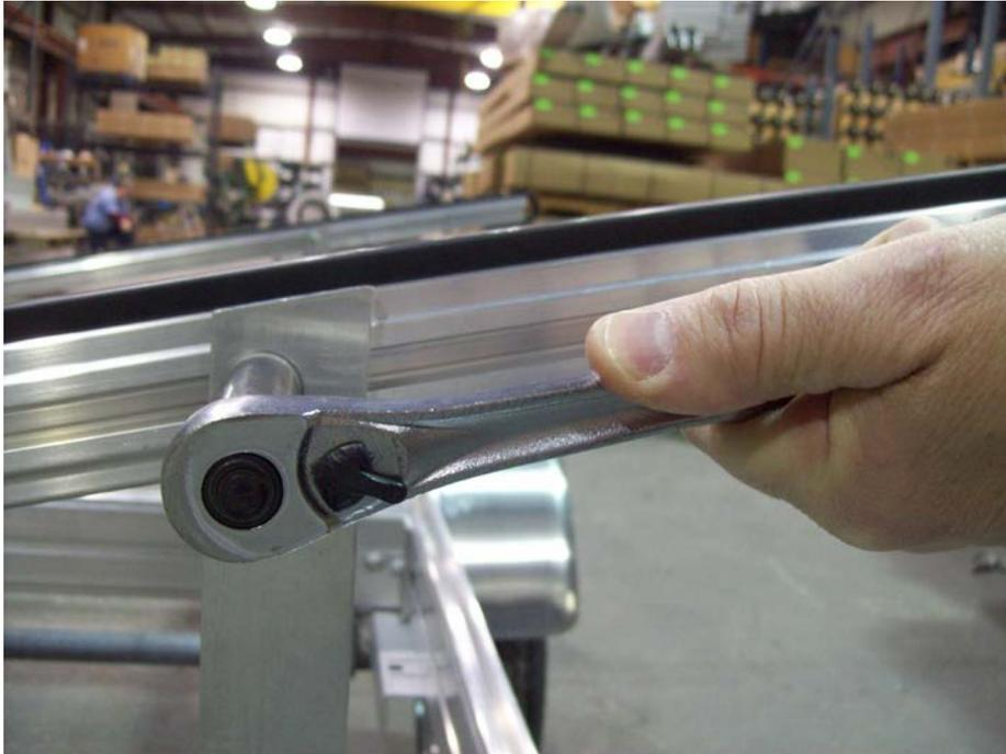
Tighten nut on arm assembly. Repeat this process for all four corners.
