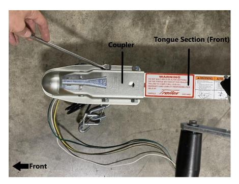
Install the coupler to the tongue section as shown. The tongue section will have pre-drilled holes for the coupler bolts. Replace the bolts and tighten the nuts using a ¾" ratchet and wrench.
