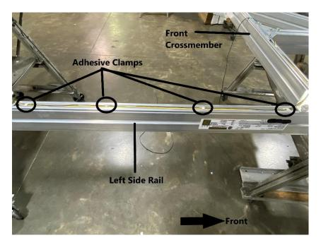
Place four adhesive clamps on the first half of the left side rail as shown. Continue to run the harness through the wire clamps.
