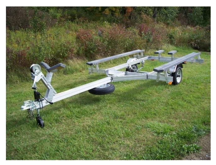
The trailer is now assembled. Connect the flat four prong harness to the tow vehicle and confirm that all lights are in working order. Connect the safety cables to the tow vehicle in a crossing pattern. Connect the coupler to the hitch ball and confirm that the size of the coupler matches the hitch ball. Use a lock to confirm the coupler is locked in place. Torque the lug nuts after 20 miles to 80 foot pounds.
