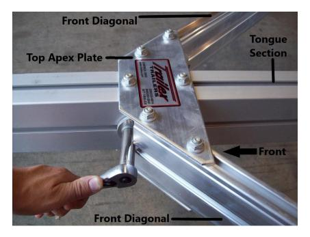
Place locknuts on all ten T-bolts going through the top apex plate (6 total) and triangle plate (4 total). Tighten all nuts connecting the tongue section, top apex plate, triangle plate and front diagonals.
