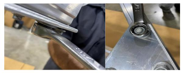
Tighten all locknuts connecting the apex plate to the front diagonals.
