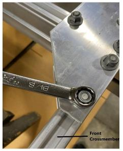
Use a 9/16 wrench to tighten all the T-bolts connecting the side-rails to the front crossmember.
