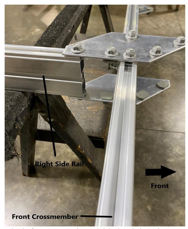
Take the front crossmember and slide the T-bolts in the grooves of the right side-rail
