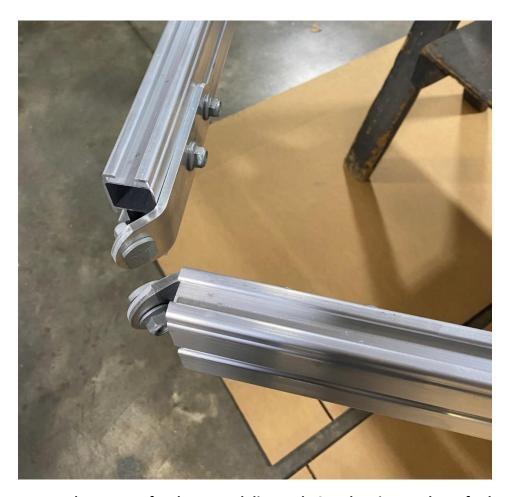
Repeat the process for the second diagonal. See the picture above for how the diagonals should be positioned. The tongue section will later be attached through these diagonals.
