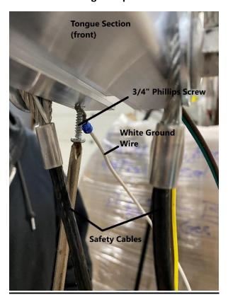
Using a Phillips screwdriver, install the Phillips screw through the ring terminal on the white ground wire into the pre-drilled hole. The pre-drilled hole is located at the bottom of the front tongue section by the safety cables.
