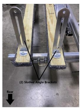
Install (2) slotted angle brackets to the rear end of the long padded bunks as shown. Replace the washers and nuts and tighten with a 9/16" wrench.
