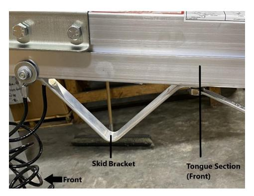
If equipped, the skid bracket will need to be removed before installing the spare tire carrier. Remove the nuts using a 9/16" wrench and then remove the skid bracket from the bottom of the tongue section.
