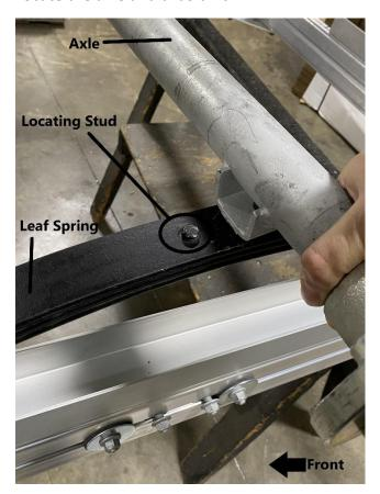
Install the axle on the leaf springs as shown. Make sure the locating studs on the springs are in the holes on the axle's spring seat. Face the axle's serial plate toward the rear of the trailer to protect it from debris.
