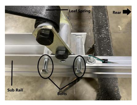
Replace the bolts into the sub rail as shown. Do not tighten the nuts yet. Repeat the process for the other side.
