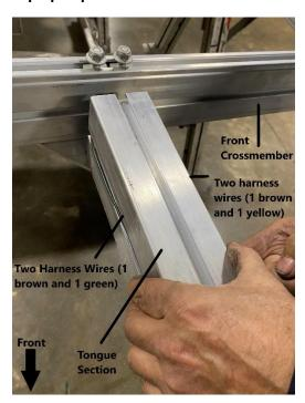
Locate the four wires of the wiring harness and put two wires (brown and green) into the groove on the left side of the rear tongue section. Hold these in place with your hand. Take the remaining two wires (brown and yellow) and place them in the groove on the right side of the tongue section. Also hold these in place with your hand. This will prevent pinching the harness between the tongue and the front crossmember. Once in place, push the tongue section so it is touching the front crossmember.
