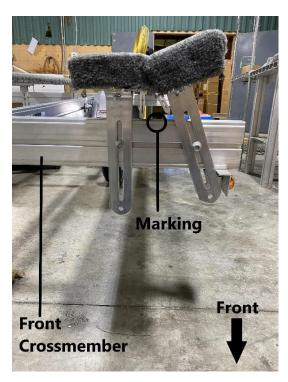
Install the long padded bunks on the front crossmember as shown. Note a marking on the top of front crossmember. This is to be used as a guide to where the long padded bunks should be touching. Tighten all nuts with a 9/16" wrench.
