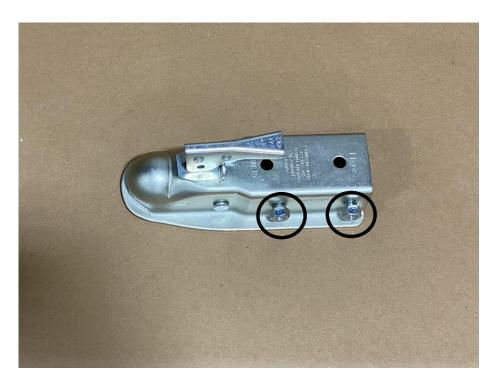
Remove the (2) nuts and (2) bolts from the coupler using a  $\frac{3}{4}$ " ratchet and wrench.
