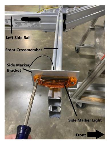
Using a Phillips screwdriver, install the side marker light to the side marker light bracket as shown. The wire will go through the large hole in the center of the bracket. Repeat this process for the other side.
