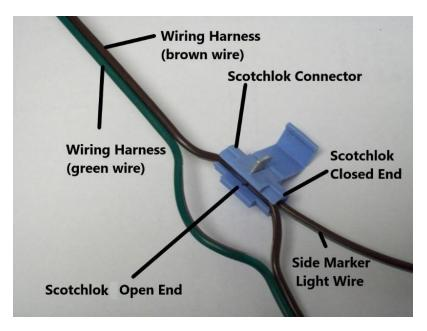
Insert the side marker light wire into the Scotchlok connector. This hole does not pass all the way through. The wire should go in about  $\frac{1}{2}$ ". Pass the brown wire of the wiring harness through the remaining open slot in the connector.
