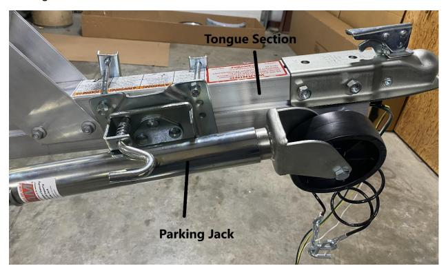
Mount the parking jack on the tongue section of the trailer as shown.
