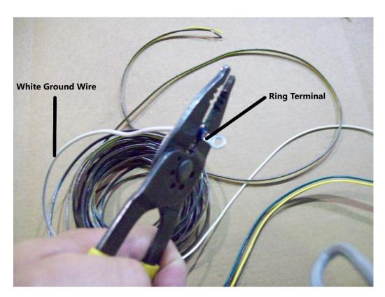
Install the ring terminal to the white ground wire as shown. Strip the end of the white ground wire, place the ring terminal on the end of the white ground wire and crimp the two together.
