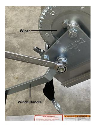
Install the winch handle as shown. Remove the nut on the winch using a ¾" wrench. Install the handle, replace the nut and tighten.
