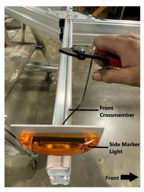
Locate the side marker light. Use wire cutters to strip the end of the side marker light wire. Repeat the process for the other side.
