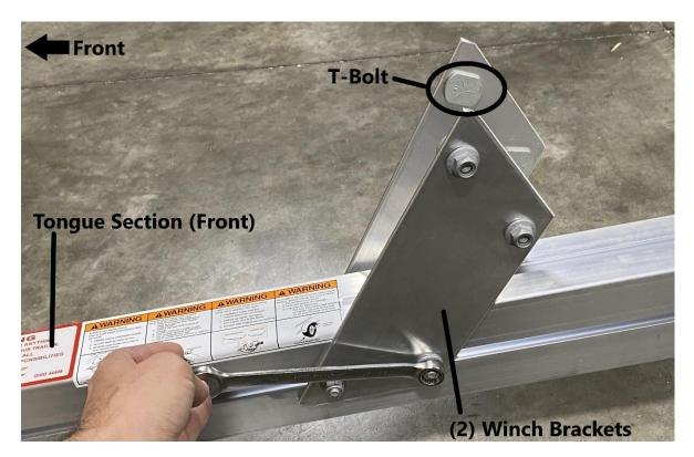
Install the winch brackets as shown. Note the position of the T-bolt pictured. All (4) T-Bolt heads should be facing inside as to later install the winch stand. Tighten the driver's side T-bolts using a 9/16" wrench. Do not tighten the passenger side T-bolts yet.
