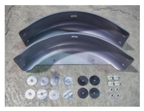
Locate the (2) plastic fenders, (8) large steel washers, (4) rubber washers, (4) 1 1/8" T-bolts and (4) nuts. Refer to the options section at the end of the manual if aluminum fenders were purchased.
