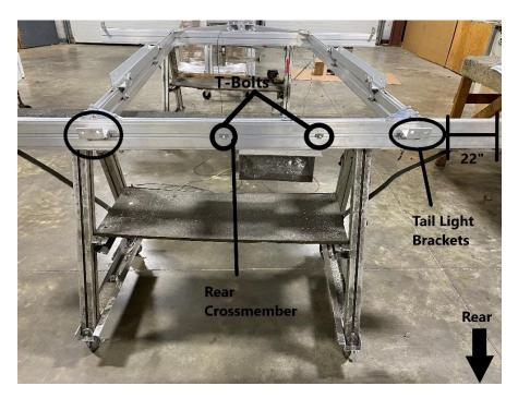
Slide two T-Bolts into the groove of the rear crossmember. These will be used later to install bunks. Slide both tail light brackets in the groove of the rear crossmember. Leave 22" from the bracket to the end of the rear crossmember.
