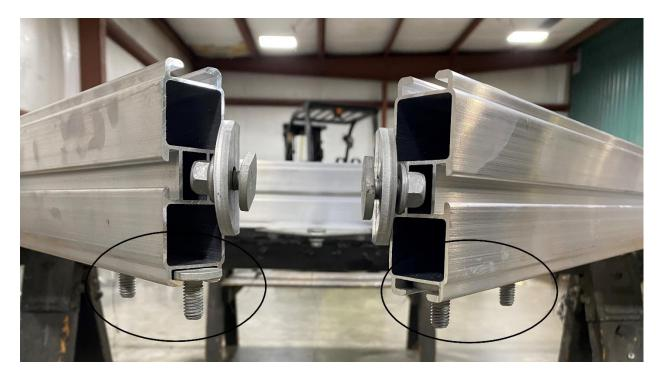
Place 2 T-bolts into each front diagonal as shown above.
