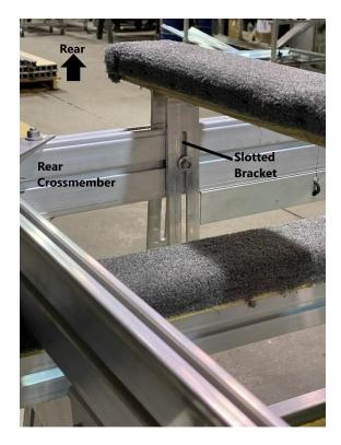
Install slotted angle bracket as shown on the other side of the rear crossmember. Tighten all nuts with a 9/16" wrench. Repeat this process for the other side of the front crossmember.
