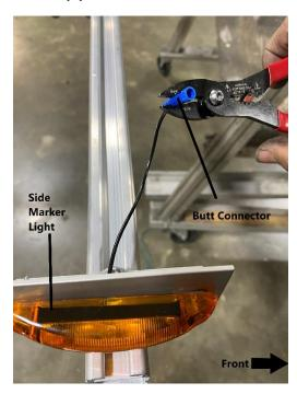
Use wire cutters to crimp the side marker light wire to the butt connector. Repeat the process for the other side.
