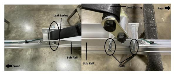
Tighten the (3) sub rail mounting nuts that were left loose previously. Use a 9/16" and  $\frac{3}{4}$ " wrench.
