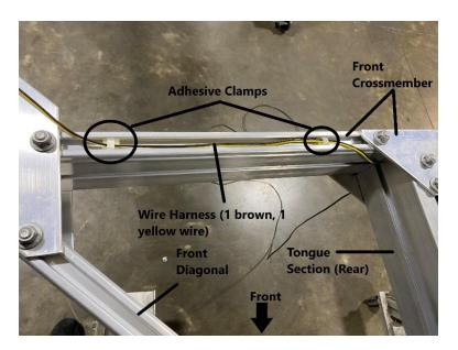
Remove the adhesive backing from the wire clamp and place two clamps into the groove of the front crossmember. Run the wire harness through wire clamps. A standard screwdriver may be necessary to push the clamp fully into the front crossmember.
