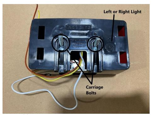
Place the (2) Carriage bolts into the grooves in the tail lights as shown. Note that the back of tail light shows if the light is the left/driver side (LH) or the right/passenger side (RH). It will also show which end is the top of the tail light.
