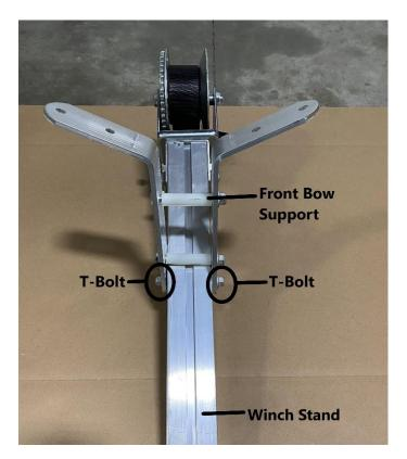
Install the Front Bow Support to the Winch Stand as shown. Remove the bottom (2) nuts from the T-bolts using a 9/16" wrench. Then slide the T-Bolts on the front bow support into the grooves of the winch stand. Replace the nuts and tighten.
