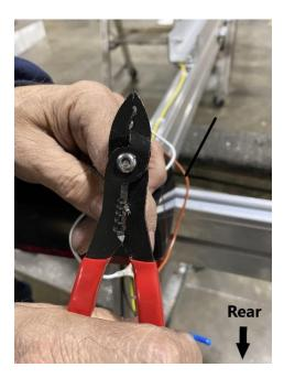
Use a pair of wire cutters to strip the ends of the (4) tail light wires, (4) harness wires and (1) LED 3 Light Bar wire. Note that the white ground wire on the tail light will be installed later.
