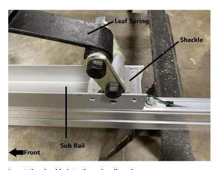
Insert the shackle into the sub rail as shown.
