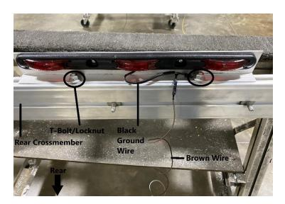
Attach the black ground wire to the T-bolt used to mount the LED 3 light bar to the rear crossmember. Tighten the locknuts using a 9/16" wrench. The brown wire will be used later to attach to the main wiring harness.
