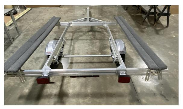
Repeat the process to install long padded bunks on the passenger side of the trailer. Note the angle of the bunks on the passenger side. Once installed, the trailer should look like this.
