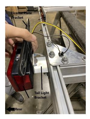
Mount the tail light and license plate bracket to the tail light bracket as shown. Note that the trailer is flipped so the tail light will be mounted upside down. Refer to the back of the tail light for which end is the top.
