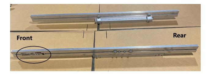
Position the left and the right side-rails as shown. Note the position of the vehicle identification sticker on the left side-rail.
