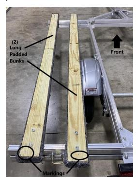
Place (2) long padded bunks on the trailer as shown. Note the markings on the back of the bunks. "F" stands for front of trailer. "R" stands for rear of trailer.
