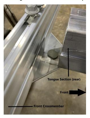
Continue sliding the tongue section until it is resting by the front crossmember. Leave a gap between the tongue section and the front crossmember.
