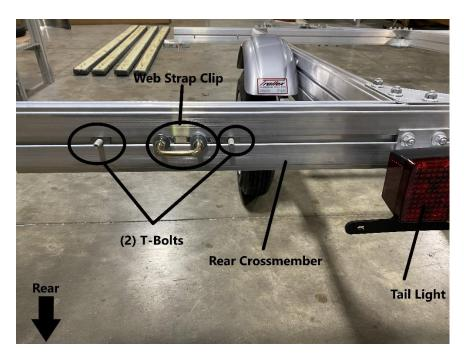
Place (2) T-Bolts and (1) Web Strap Clip into the rear crossmember as shown. Repeat the process for the other side.
