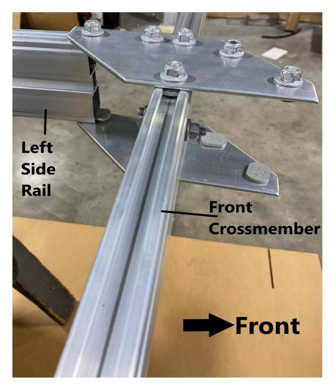
Take the front crossmember and slide the T-bolts in the grooves of the left side-rail.
