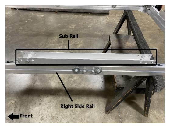
Locate the sub rail. The sub rail will already be installed on both the left and right side rails.
