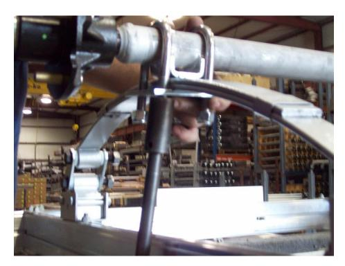
Tighten all the U-bolts nuts evenly using a 9/16 ratchet.
