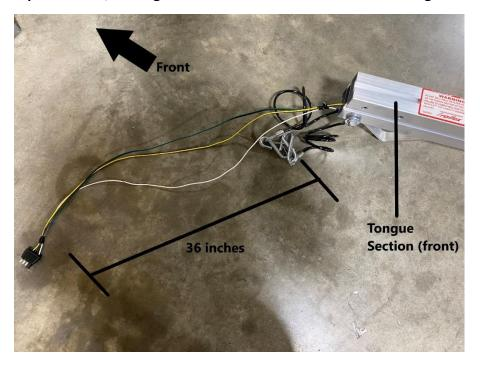
Pull the harness through the tongue section. Leave 36 inches of wiring at the front of the tongue section. This will be used to connect the trailer to the tow vehicle.
