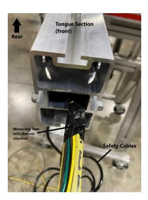
Extend a tape measure inside the middle of the tongue section.
