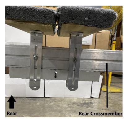
Install (2) slotted angle brackets on the other side of the rear crossmember. Tighten the nuts using a 9/16" wrench.
