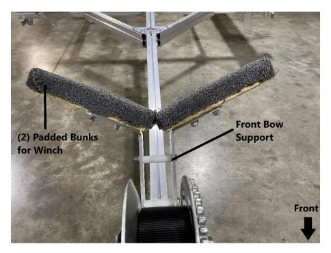
Install the (2) padded bunks to the front bow support as shown. Replace and tighten the nuts using a 9/16" wrench.
