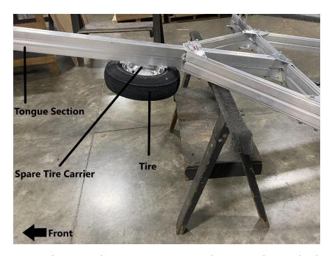
Mount the tire to the spare tire carrier as shown. Replace and tighten the lug nuts.
