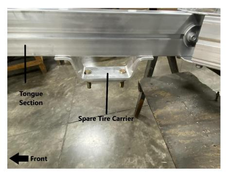
Mount the spare tire carrier to the T-bolts that were placed in the groove on the bottom of the tongue section. Tighten the locknuts using a 9/16" wrench.
