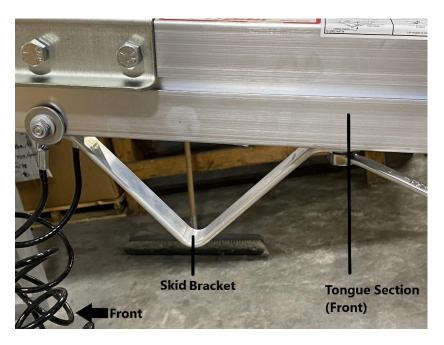
If equipped, the skid bracket will need to be removed before installing the parking jack. Remove the nuts using a 9/16" wrench and then remove the skid bracket from the bottom of the tongue section.
