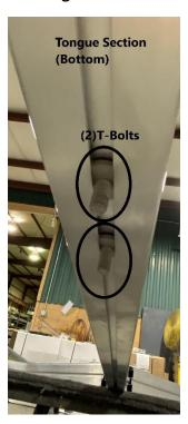
Place the (2) T-bolts that were removed from the spare tire carrier into the groove on the bottom of the tongue section.
