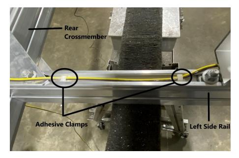
Place two adhesive clamps in the left side rail, right before it connects to the rear crossmember. Run the harness through the clips and leave the excess wire hanging over the rear crossmember. Repeat this process for the right side rail.
