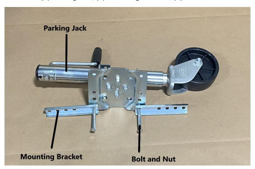
Mount the brackets to the parking jack as shown. Remove the nuts from the bolts and place the bolt through the mounting bracket and jack. Loosely replace the nut.
