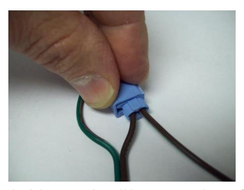
Close the hinge cover on the Scotchlok Connector. Repeat this process for the other side.
