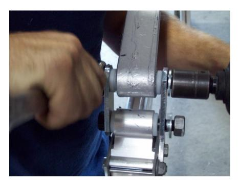
Tighten the rear shackle nuts with 7/8" wrench until the metal washers are secure. Do not over tighten as this will not allow the suspension to move properly.
