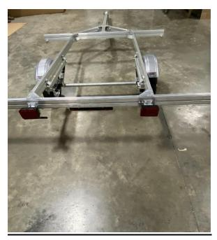
The trailer will now need to be flipped right side up to continue assembly. Note that the trailer will be significantly heavier than the last time it was flipped. At least two people will be needed.
