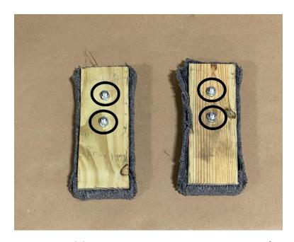
Remove the (4) nuts from the padded bunks using a 9/16" wrench.
