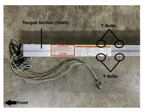
Install (4) T-Bolts into the grooves of the front tongue section as shown. These will be used to mount the winch.
