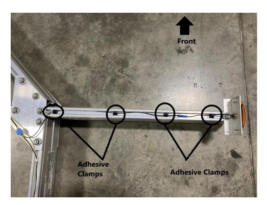
Use (4) Adhesive clamps to secure the side marker light wire into the groove in the front crossmember. Repeat this process for the other side.
