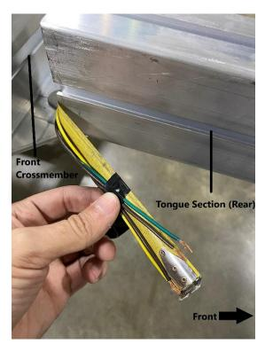
Continue to extend the tape measure inside the front tongue section until it protrudes out of the rear of the tongue by the front crossmember. Remove the electrical tape and retract the tape measure, leaving the harness wires at the rear of the tongue section.
