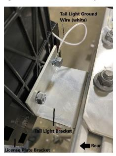
Mount the white tail light ground wire a shown. Tighten both nuts to finish installation of the tail light. Repeat the process for the other side.
