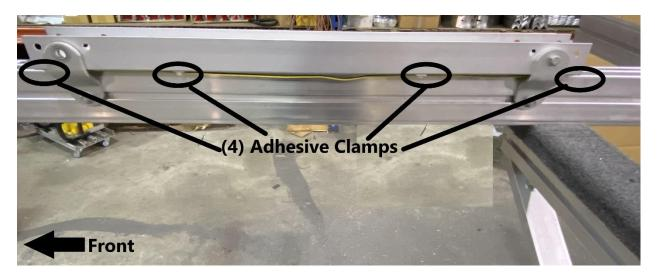
Place four adhesive clamps underneath the sub rail clip and continue running the harness through the clips.
