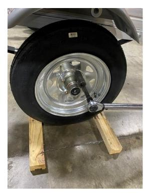
Place (4) wheel chocks as shown, (2) on each tire. Torque the lug nuts to 80 foot pounds using a X pattern. Repeat the process for the other tire. Note that after 20 miles the lug nuts will need to be re-torqued to 80 foot pounds.
