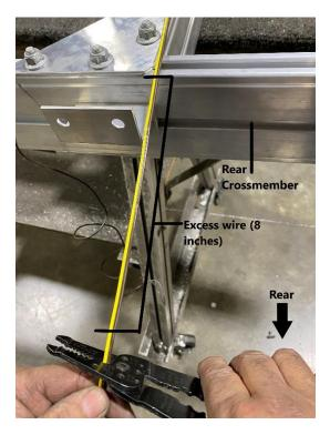
Measure 8" of excess wire from the end of the rear crossmember. Use wire cutters to cut the excess wire. <u>Do not throw away the excess wire.</u> The excess wire will be used to connect the side marker lights to the harness. Repeat the process for the other side.
