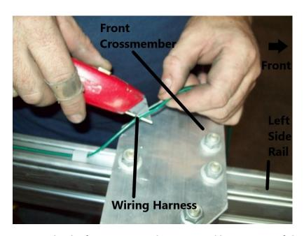
Use a utility knife to separate the green and brown wire of the wiring harness as shown on the front crossmember. This is to splice the side marker light into the harness. Repeat the process for the yellow and brown wire on the other side.
