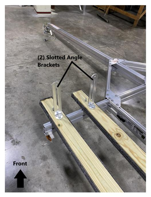
Install (2) slotted angle brackets to the front end of the long padded bunks as shown. Note that these will be installed on the inner bolts on the long padded bunks. Replace the washers and nuts and tighten with a 9/16" wrench.
