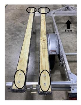
Remove the (8) washers and (8) nuts from the (2) long padded bunks with a 9/16" wrench.
