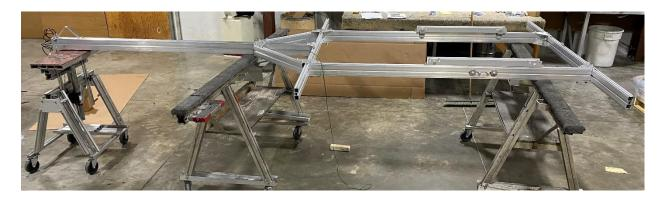
The trailer will now need to be flipped upside down in order to continue assembly. At least two people will be necessary to flip the trailer. Be careful not to damage the harness. See the picture above for how your trailer should look upside down.
