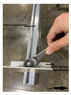
Tighten the nut on the side market light bracket using a 9/16" wrench. Repeat this process to install the second side market light bracket on the other side of the front crossmember.
