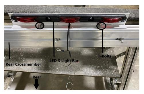
Locate (2) T-Bolts on the top of the rear crossmember. Remove the locknuts from the T-bolts and place the T-bolts through the holes on the LED 3 light bar.
