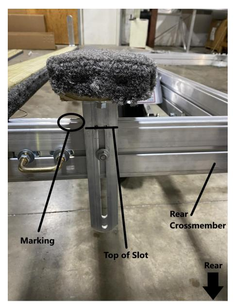
Flip the inside long padded bunk and install the bunk on the right T-bolt on the rear crossmember as shown. Note that the top of the slot on the slotted angle bracket should the same height as the top of the rear crossmember. Also note the marking on the rear crossmember. This marking shows where the left side of the inside long padded bunk should be positioned. Place a locknut on the T-bolt and tighten with a 9/16" wrench.
