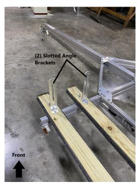
Install (2) slotted angle brackets to the front end of the long padded bunks as shown. Note that these will be installed on the inner bolts on the long padded bunks. Replace the washers and nuts and tighten with a 9/16" wrench.
