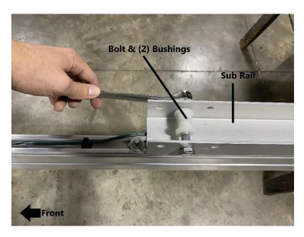
Use a 3/4" wrench to remove the front bolt and 2 nylon bushings.
