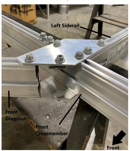
Slide the front diagonal into the aluminum plate connecting the front crossmember to the left side-rail.
