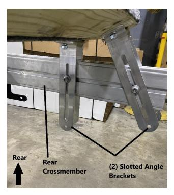
Install (2) slotted angle brackets as shown on the other side of the rear crossmember. Tighten all nuts with a 9/16" wrench. Repeat this process for the other side of the front crossmember.
