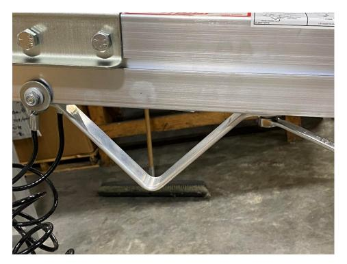
Re-install the skid bracket if necessary.
