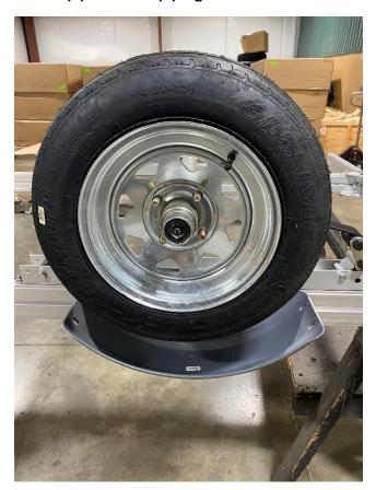
Install the wheels with the valve stems facing out.
