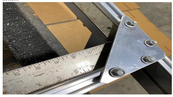
Use a square to confirm that the side-rail and the rear crossmember are at a 90-degree angle.
