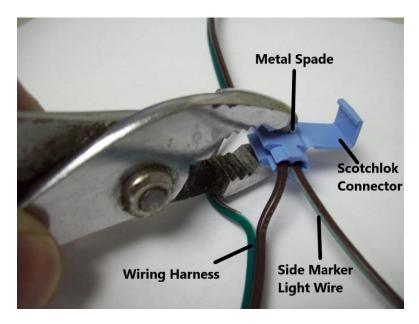
Use pliers to push the metal spade down until it is flush with the plastic of the Scotchlok Connector. This is what makes the electrical connection between the two wires.
