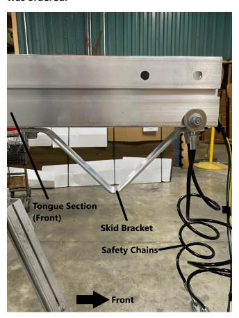
Slide skid bracket into the bottom channel of the tongue section. Position bracket as shown and tighten nuts.
