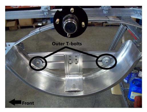
Install the washers over the outer two T-bolts. First two rubber washers, two steel washers and nuts. Slide T-bolts and washer over the inside edge of the fender then tighten nuts. Repeat the process for the other side.
