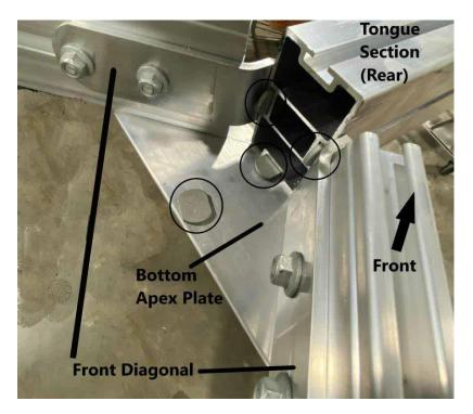
Slide the rear side of the tongue section through the T-bolts on the bottom apex plate and front diagonals. Make sure that the safety cables on the tongue section are on the bottom.
