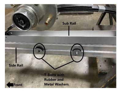
Locate the (2) T-bolts in the groove of the side rail. Place a rubber washer and a metal washer on each T-Bolt.
