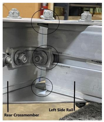
Three T-bolts will now need to slide into the left side rail. One T-bolt for the 90-degree angle will slide into the side, while two more will slide into the top and the bottom.
