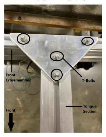
Take the triangle plate and place it through the 4 T-bolts as shown. The locknuts will need to be removed from the two T-bolts on the front crossmember.
