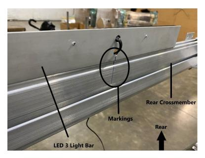
The back of the LED 3 light bar and the rear crossmember will have markings on the back. Line up the markings.
