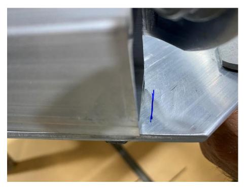
The bottom apex plate will be marked with two lines. Make sure the front diagonals line up with the marked lines.
