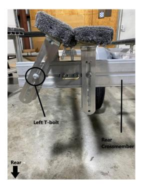
Flip the outside long padded bunk and install the bunk on the left T-bolt on the rear crossmember as shown. This bunk will be positioned at angle towards the middle of the trailer. Place a locknut on the T-bolt and tighten with a 9/16" wrench.
