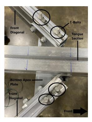
Move to the front diagonals where they are connected to the tongue section. Place 2 T-bolts into both the front diagonals. These will be used to connect the top apex plate.
