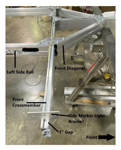
Slide the side marker light bracket into the front crossmember as shown. Leave 1" at the end of the front crossmember for the side marker light.
