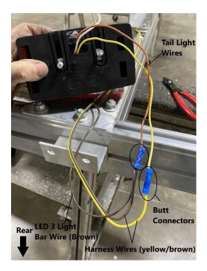
Use butt connectors to connect the tail light and the LED 3 light bar to the wiring harness as shown. Match the brown wire of the harness with the brown wire of the tail light. Same for the yellow wires. Note that both the brown LED 3 light bar wire and the brown harness wire will need to be connected together.
