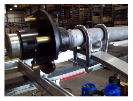
Install U-bolts and Tie Plates as shown.
