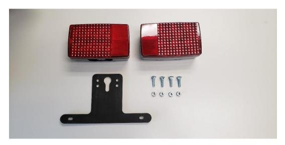
Locate (2) tail lights, (1) license plate bracket, (4) carriage bolts and (4) nuts. These will be inside the LED Light Box.
