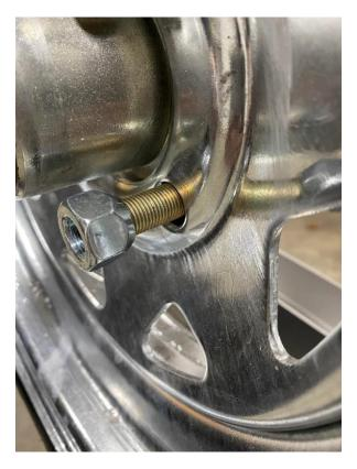
Install the lug nuts with the tapered side facing the wheel. Note that the lug nuts will be torqued later in the assembly.
