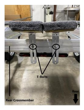
Install the long padded bunks using the T-bolts in the groove of the rear crossmember. These are the T-bolts that were installed earlier during the tail light installation. Tighten the nuts using a 9/16" wrench. Note that the top of the slot on the slotted angle bracket should be level with the top of the rear crossmember.
