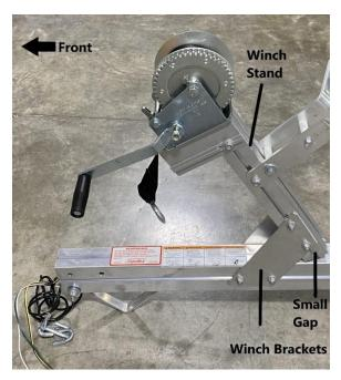
Install the winch stand on the winch brackets as shown. Slide the (4) T-bolts of the winch bracket into the grooves of the winch stand. Leave a very small gap between the winch stand and the tongue section. Tighten all nuts with a 9/16" wrench. This includes the passenger side nuts in the tongue section that were left loose earlier.
