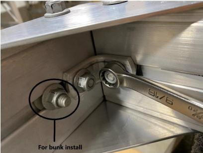
Use a 9/16" wrench to tighten all the T-bolts connecting the side-rails to the rear crossmember. Note that there is a T-bolt and locknut next to the angle. This will be used later to install bunks.
