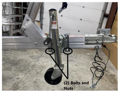
Install the remaining (2) bolt and nuts as shown. Tighten the nuts using a 9/16" ratchet and wrench.
