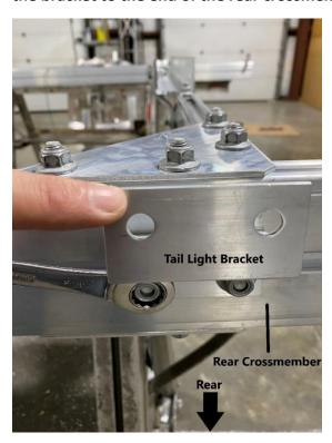
Tighten the nuts on the tail light bracket using a 9/16" wrench. Repeat the process for the other bracket.
