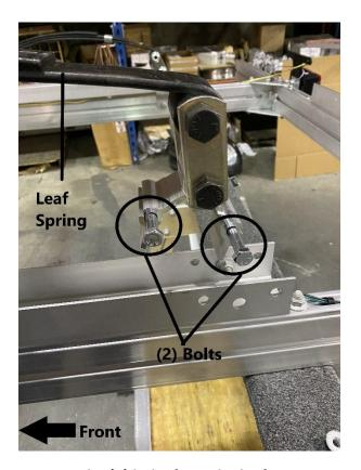
Remove the (2) bolts from the leaf spring assembly using a 9/16" ratchet and wrench.
