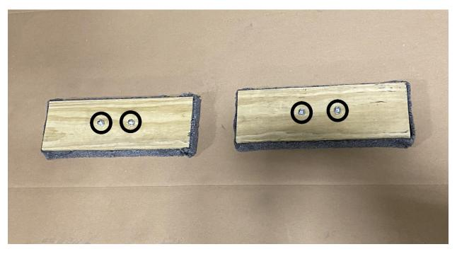
Remove the (4) nuts using a 9/16" wrench.
