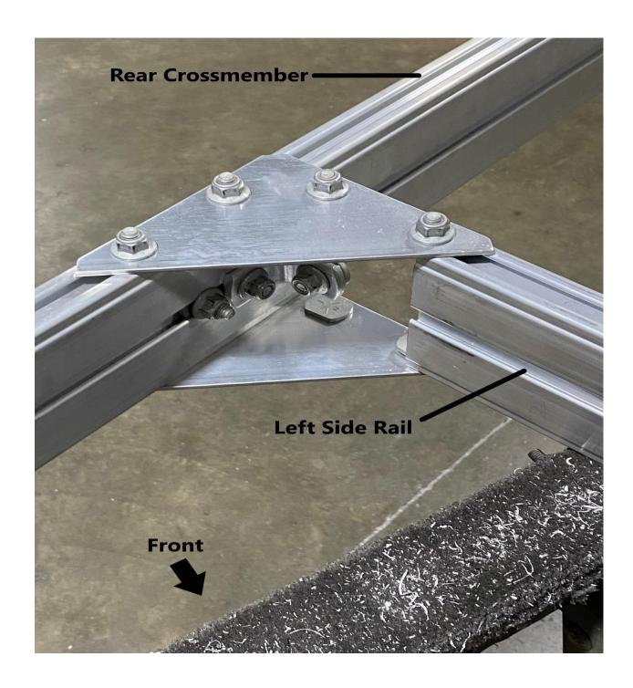
Slide the rear crossmember onto the left side-rail, making sure to engage the T-bolts into the top and bottom slots on the side rail. Spray lubricant (not included) will make this process easier.
