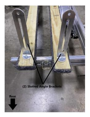
Install (2) slotted angle brackets to the rear end on the long padded bunks as shown. Note the markings on the back of the bunks. "F" stands for front of trailer. "R" stands for rear of trailer. Replace the washers and nuts and tighten with a 9/16" wrench.
