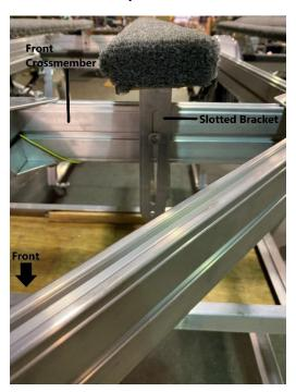
Install the slotted bracket using the T-bolts in the groove of the front crossmember. Tighten the nuts using a 9/16" wrench. Note that the top of the slot on the slotted angle bracket should be level with the top of the rear crossmember.
