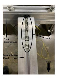
Move to the rear part of the tongue section. Insert 4 T-bolts from the hardware bag into the top groove of the tongue section. These will be used to connect the triangle plate and the top apex plate.
