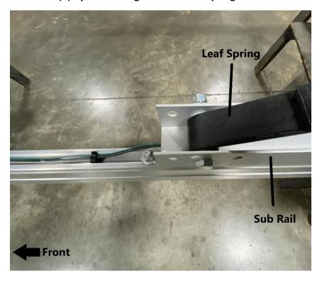
Install the leaf spring into the sub rail as shown. Do not tighten the bolt yet.
