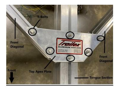
Move two T-bolts down the tongue section until they are by the front diagonals. Take the top apex plate and place it through the 6 T-bolts.
