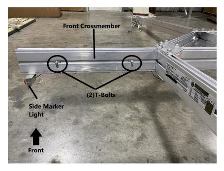
Place (2) T-bolts into the side of the front crossmember as shown. Repeat the process for the other side.
