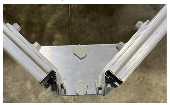
Connect the bottom apex plate to both front diagonals using the T-bolts. Use the locknuts to loosely hold the apex plate in place.
