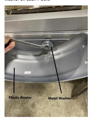
Mount the fender on the T-bolts as shown. Place an additional metal washer on the other side of the fender. Tighten the nuts using a 9/16" wrench. Repeat the process for the other side.
