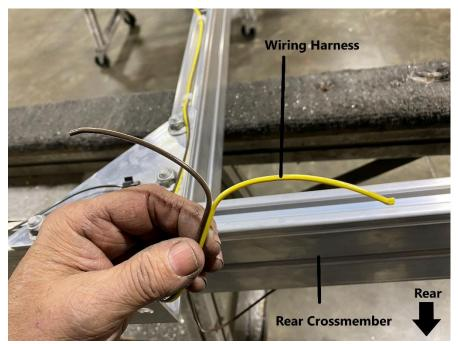
Locate the end of the wiring harness by rear crossmember. Use a utility knife to split the two wires of the wiring harness. Repeat this process for the other side.
