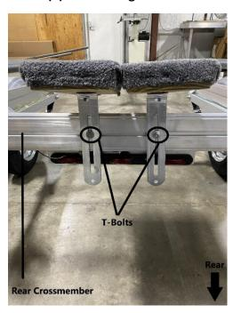
Install the rear padded bunks using the T-bolts in the groove of the rear crossmember. These are the T-bolts that were installed earlier during the tail light installation. Tighten the nuts using a 9/16" wrench. Note that the top of the slot on the slotted angle bracket should be level with the top of the rear crossmember.
